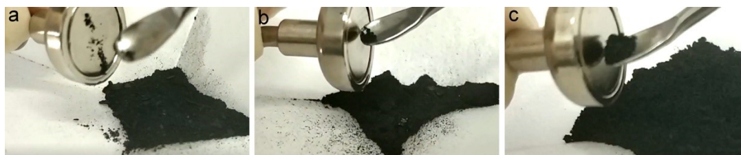
Fig. S12. Magnetic adsorption effects of (a) Co-C, (b) Co-NC and (c) CoN5 SA/NC. Magnetic adsorption effect of Co-C can be observed when the sample is closed to a powerful magnet. Movie S1 also presents the magnetic adsorption effect of Co-C. However, no similar phenomena may be found for Co-NC (Movie S2) and CoN5 SA/NC (Movie S3), indicating abundant Co atoms are bonded to heteroatom N leading to special magnetic properties, which are different from that of Co-C.
