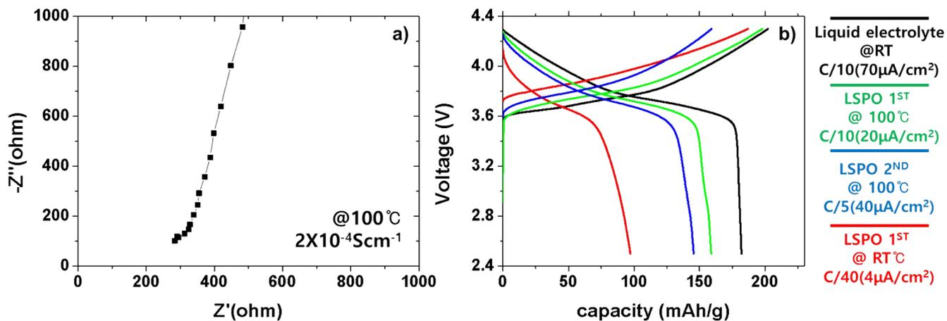
Figure S5. (a) Nyquist plot data of LSPO SE at 100°C (b) Voltage curves of the Co-sintered ASSB with NMC622 and Li at different rates and temperature. Liquid electrolyte at RT: C/10 ( $70 \mu\text{A}/\text{cm}^2$ ), ASSB 1st at 100 °C: C/10 ( $20 \mu\text{A}/\text{cm}^2$ ), ASSB 2nd at 100 °C: C/5 rate ( $40 \mu\text{A}/\text{cm}^2$ ), ASSB at RT: C/40 ( $4 \mu\text{A}/\text{cm}^2$ )
