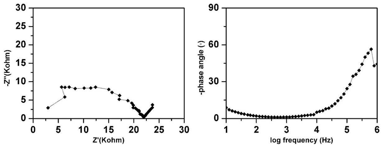
Figure S3. Nyquist and bode plot of the LSPO-based ASSB cell. (NMC622-LSPO SE cathode composite/LSPO SE/Li metal).
