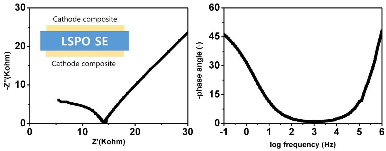
Figure S4. Nyquist and bode plot of the NMC622 cathode composite/LSPO/NMC622 cathode composite symmetric cell
