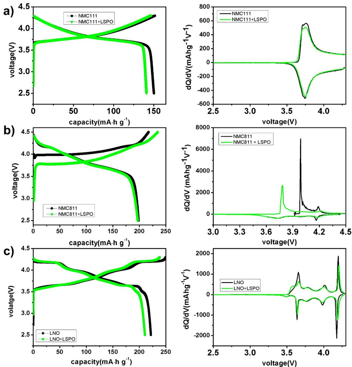
Figure S2. Voltage profiles and differential capacity ( $dQ/dV$ ) plots of (a)  $\text{LiNi}_{1/3}\text{Mn}_{1/3}\text{Co}_{1/3}\text{O}_2$  (NMC111), (b)  $\text{LiNi}_{0.8}\text{Mn}_{0.1}\text{Co}_{0.1}\text{O}_2$  (NMC811) before and after co-sintering with LSPO SE at 700 °C
