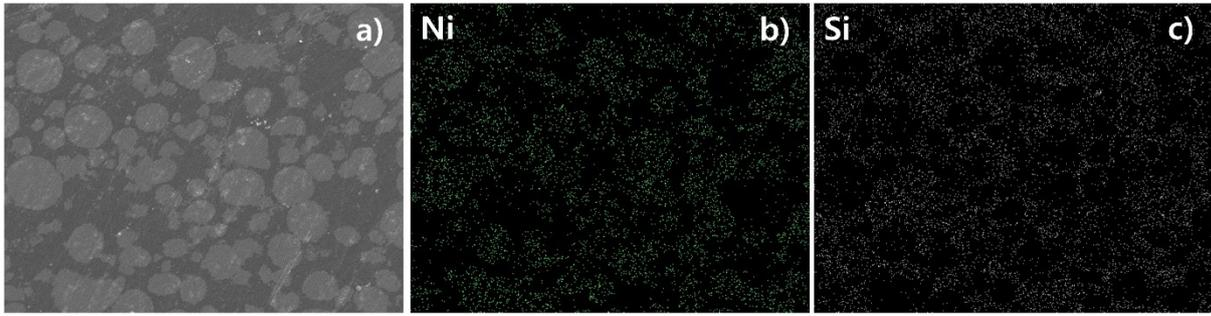
Figure S1. a) SEM and EDS image of b) Ni, c) Si of the co-sintered NMC622 with LSPO SE at 700 °C
