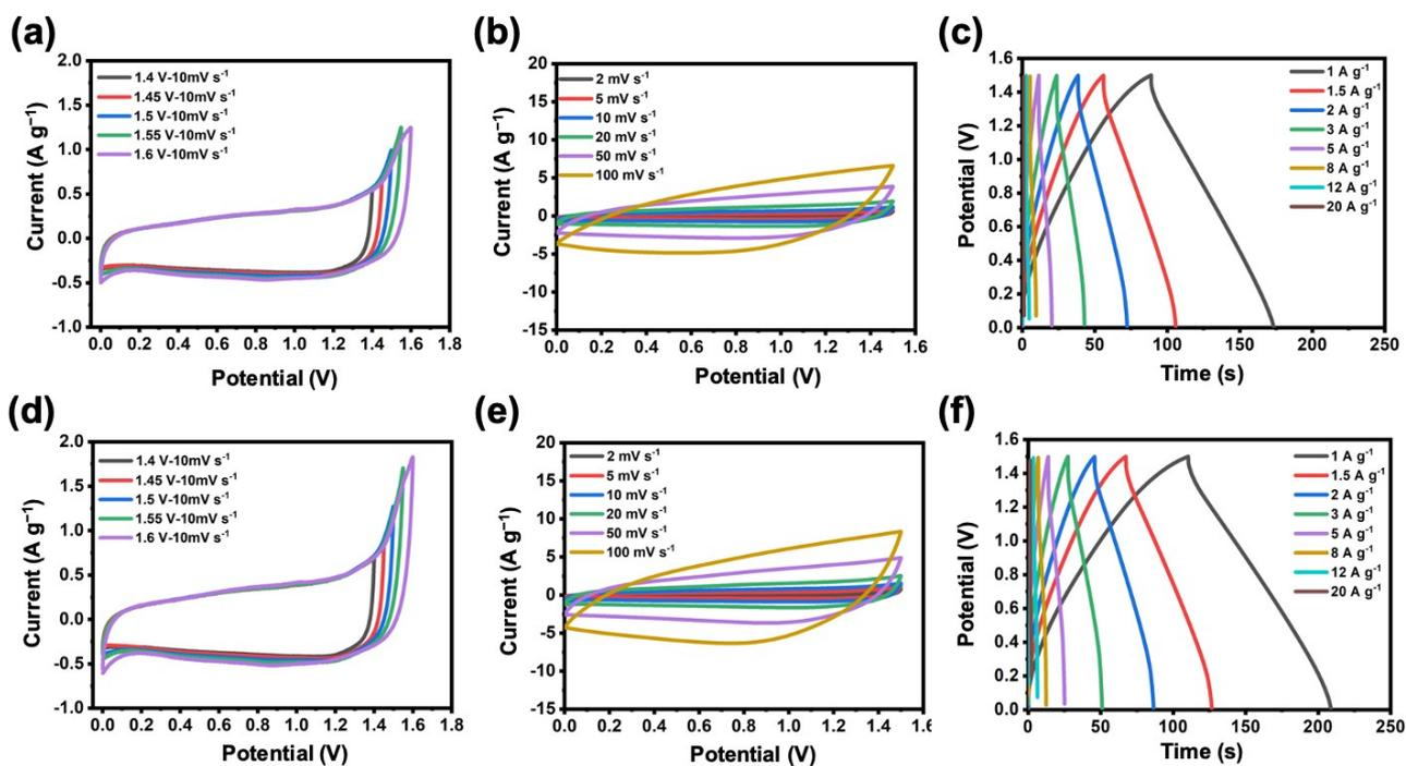
Figure S16 (a) CV curves at 10 mV s<sup>-1</sup>, (b) CV curves and (c) GCD curves of CoNiLDH//AC ASC device. (d) CV curves at 10 mV s<sup>-1</sup>, (e) CV curves and (f) GCD curves of CoNiLDH-rGO//AC ASC device.
