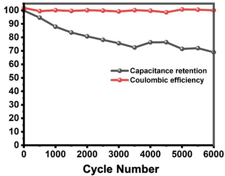
**Figure S17** Long-term cycling performance and coulombic efficiency of the CoNiLDH-rGO-CoNi<sub>2</sub>S<sub>4</sub>-2//AC ASC at 3 A g<sup>-1</sup> for 6 000 cycles.
