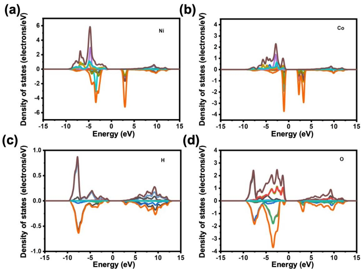
**Figure S1** Projected density of states of (a) Ni (b) Co (c) H and (d) O of CoNiLDH.
