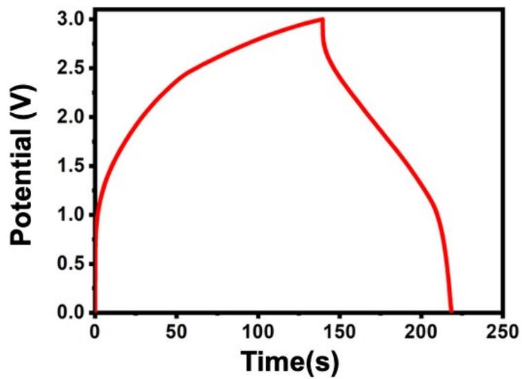
**Figure S18** GCD curves at 1 A g<sup>-1</sup> of CoNiLDH-rGO-CoNi<sub>2</sub>S<sub>4</sub> //KOH+PVA//AC ASC devices in series.
