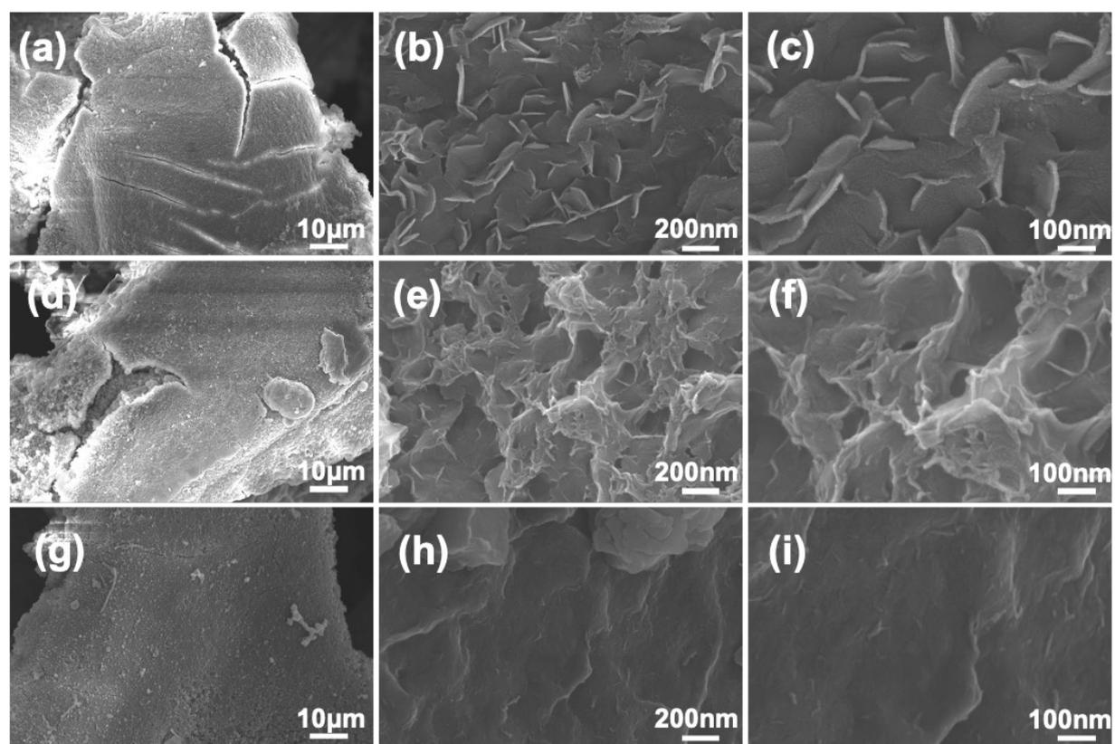
**Figure S7** (a) Low-magnification and (b, c) high-magnification SEM images of  $\text{CoNiLDH-CoNi}_2\text{S}_4$ -2. (d) Low-magnification and (e, f) high-magnification SEM images of  $\text{CoNiLDH-CoNi}_2\text{S}_4$ -6. (g) low-
