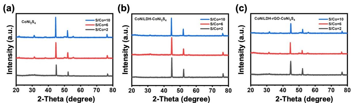
**Figure S3** XRD patterns CoNi<sub>2</sub>S<sub>4</sub>, CoNiLDH-CoNi<sub>2</sub>S<sub>4</sub>, and CoNiLDH-rGO-CoNi<sub>2</sub>S<sub>4</sub> of different S/Co ratios.
