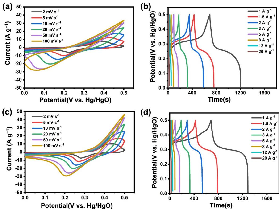
**Figure S11** (a) CV curves and (b) GCD curves of CoNiLDH. (c) CV curves and (d) GCD curves of CoNiLDH-rGO.
