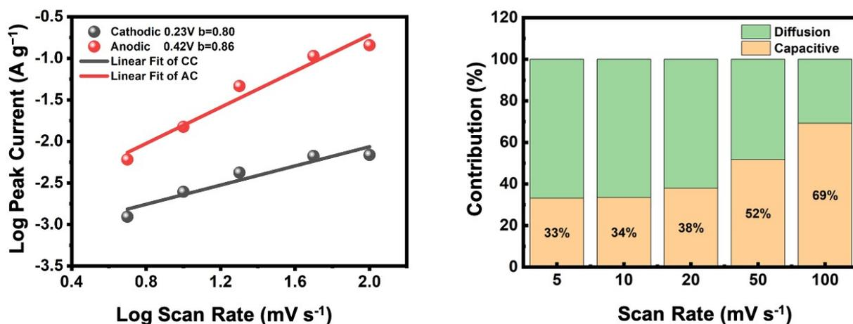
**Figure S13** (a) The relationship between  $\log(i)$  and  $\log(v)$  for CoNiLDH-rGO-CoNi<sub>2</sub>S<sub>4</sub>-2 electrode, (b) comparison of the capacitive contribution and diffusion contribution.
