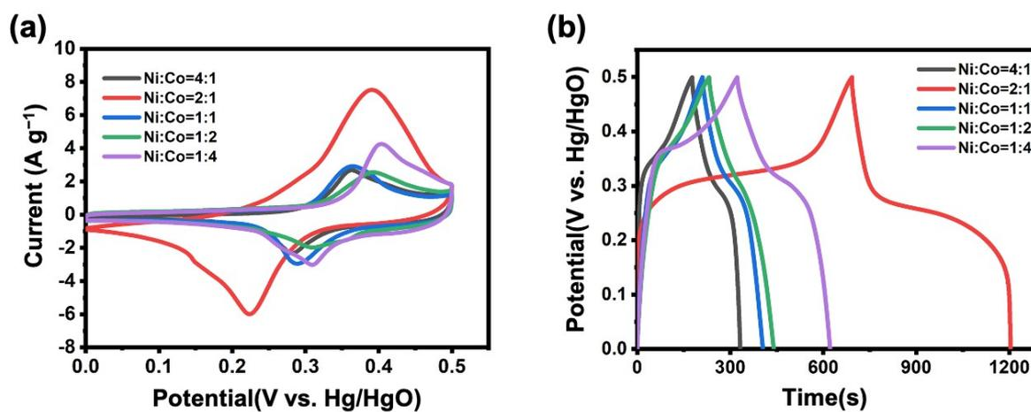
**Figure S10** (a) CV curves and (b) GCD curves of CoNiLDH at different Ni/Co ratio of 4:1,2:1,1:1,1:2, and 1:4.
