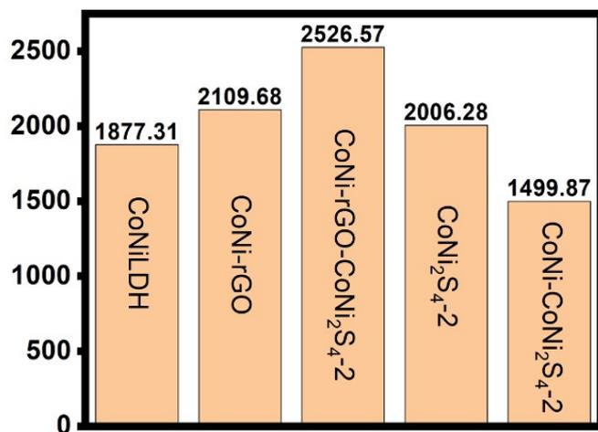
**Figure S12** Mass specific capacitances of different electrodes calculated from CV curves.
