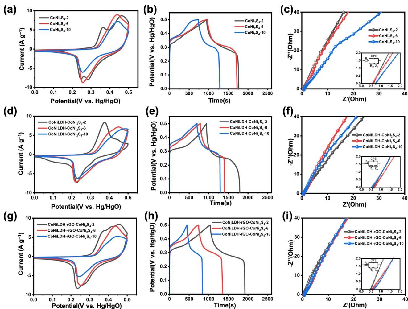
**Figure S14** (a) CV curves at 2 mV s<sup>-1</sup>, (b) GCD curves at 1 A g<sup>-1</sup> and (c) Nyquist plots of CoNi<sub>2</sub>S<sub>4</sub>-2, CoNi<sub>2</sub>S<sub>4</sub>-6 and CoNi<sub>2</sub>S<sub>4</sub>-10. (d) CV curves at 2 mV s<sup>-1</sup>, (e) GCD curves at 1 A g<sup>-1</sup> and (f) EIS spectra of CoNiLDH-CoNi<sub>2</sub>S<sub>4</sub>-2, CoNiLDH-CoNi<sub>2</sub>S<sub>4</sub>-6 and CoNiLDH-CoNi<sub>2</sub>S<sub>4</sub>-10. (h) CV curves at 2 mV s<sup>-1</sup>, (i) GCD curves at
