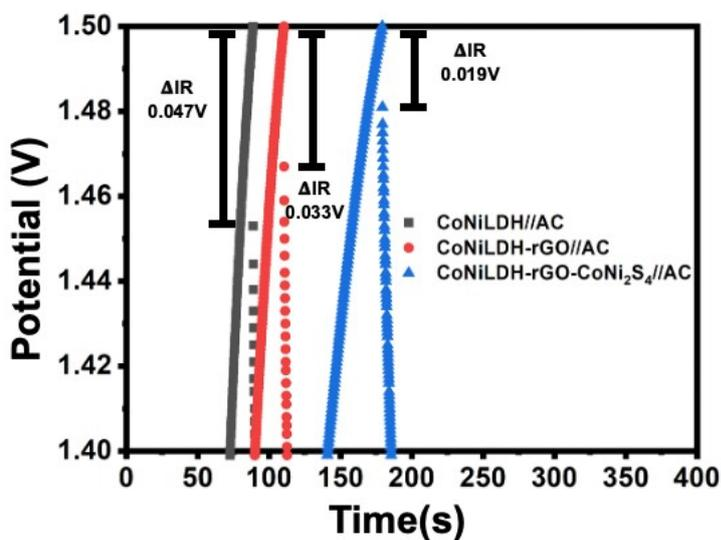
Figure S15  $\Delta$ IR drop of different ASC devices.
