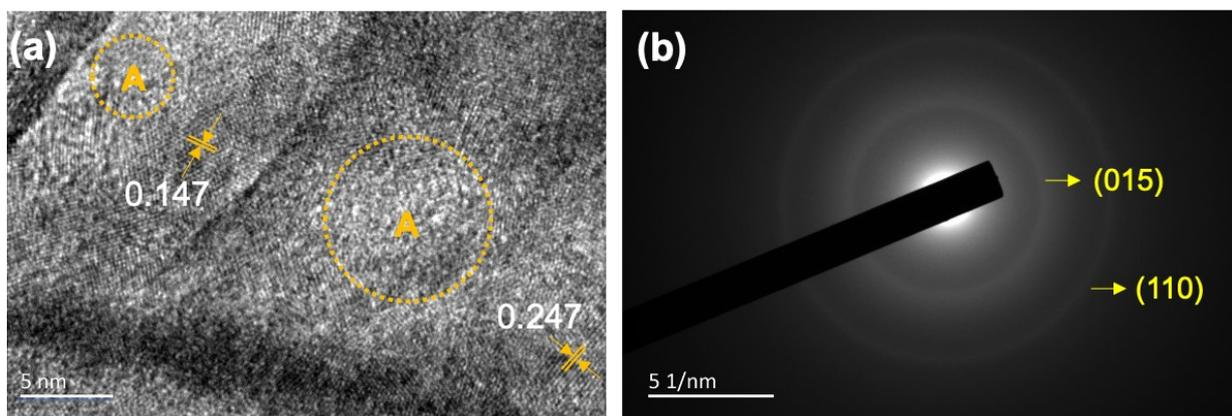
**Figure S9** (a) HRTEM and (b) SAED images of CoNiLDH-rGO-CoNi<sub>2</sub>S<sub>4</sub>.
