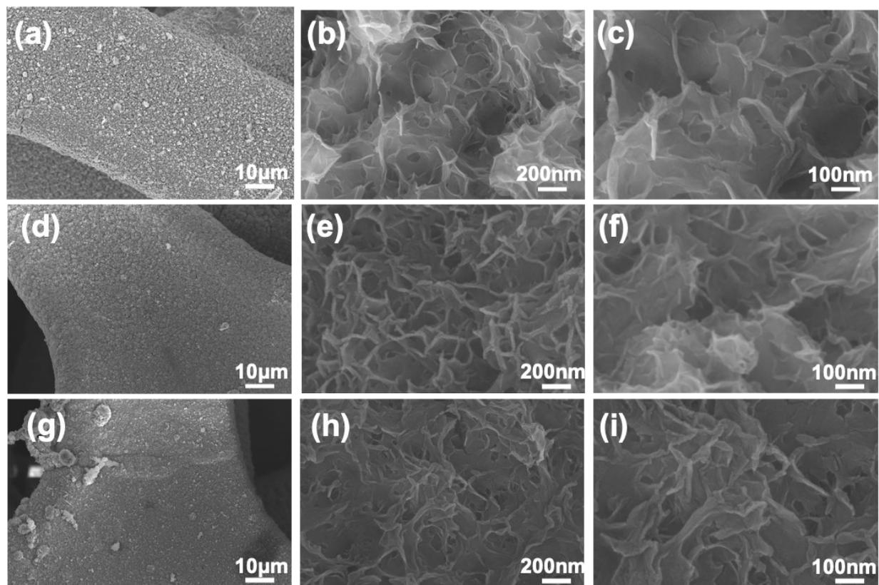
**Figure S6** (a) Low-magnification and (b,c) high-magnification SEM images of  $\text{CoNi}_2\text{S}_4$ -2. (d) low-magnification and (e, f) high-magnification SEM images of  $\text{CoNi}_2\text{S}_4$ -6. (g) low-magnification and (h, i) high-magnification SEM images of  $\text{CoNi}_2\text{S}_4$ -10.
