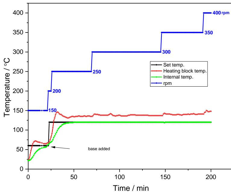
**Fig. S1** PIM-1 polymerization temperature and stirring conditions.
