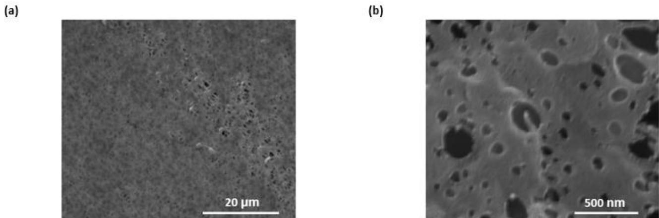
**Fig. S3** (a) and (b) show the porosity of the surface of PAN supports at low and high magnifications, respectively. From the images acquired, the average pore size and surface porosity are 45.6 nm and 11.7 %, respectively.
