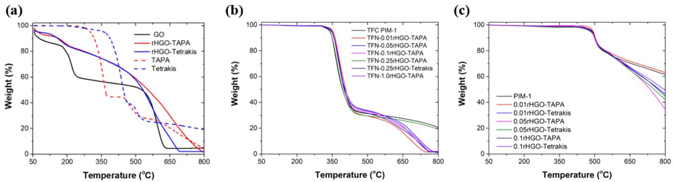
**Fig. S7** TGA curves of (a) GO, rHGO-TAPA and rHGO-Tetrakis, TAPA (as received) and Tetrakis (as received), (b) TFC PIM-1 and TFN membranes, and (c) MMMs. These measurements were conducted under a nitrogen atmosphere and a heating rate of  $10\text{ }^{\circ}\text{C min}^{-1}$ .
