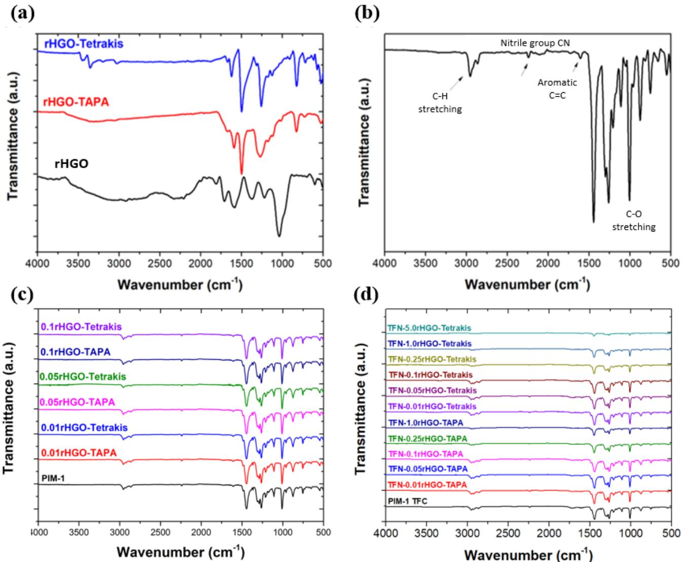
**Fig. S6** (a) FTIR spectra of rHGO, rHGO-TAPA and rHGO-Tetrakis and (b) freestanding PIM-1 membrane, (c) MMMs and (d) TFC PIM-1 and TFN membranes.
