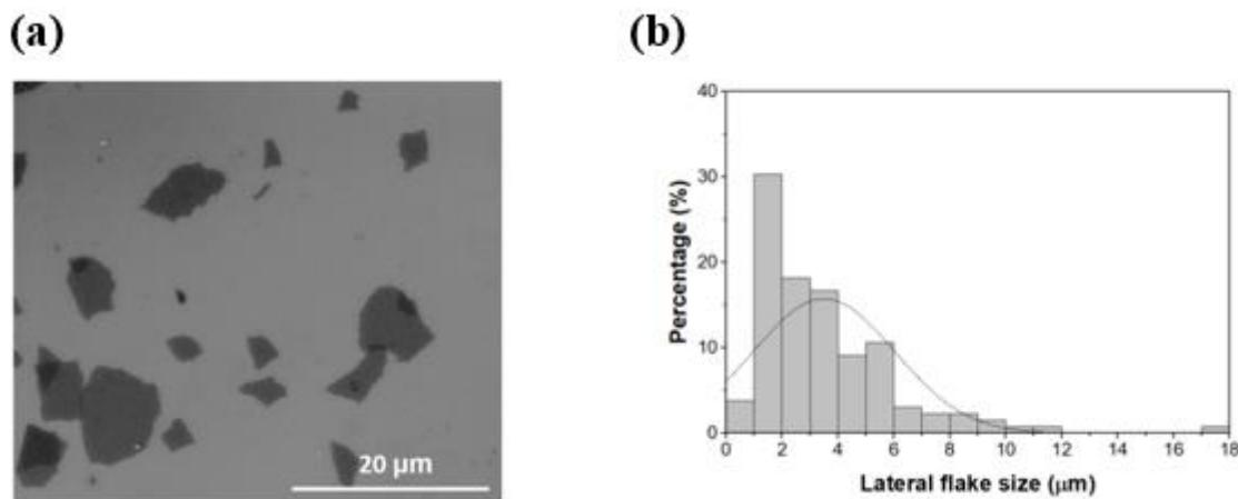
**Fig. S4** (a) SEM image of graphene flakes used in this study and (b) analysis of the lateral flake size. The histogram was fitted using the normal function as shown in the black line. The sizes of 132 flakes from multiple SEM images were measured using ImageJ®.
