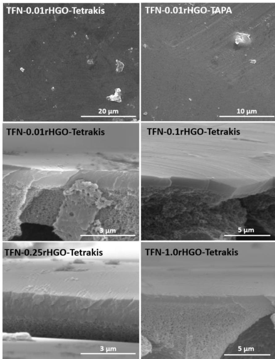
**Fig. S5** (a) Representative SEM images of the surface and cross-sections of membranes prepared in this study.
