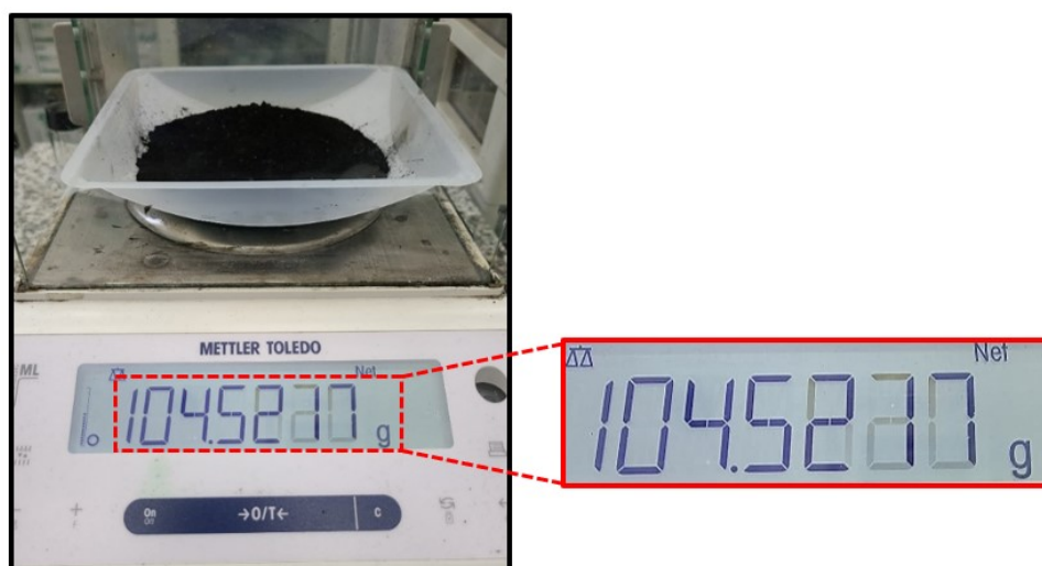
Fig. S1. The photograph of weighing results of obtained electrocatalyst in the synthesis process.
