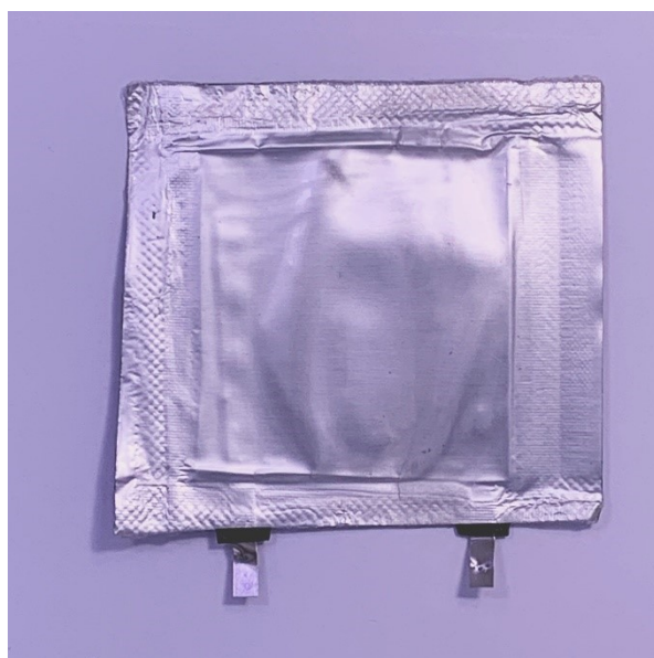
Fig. S20 Optical photo of a SiPAC//LFP pouch cell after 90° bending for 10,000 times.
