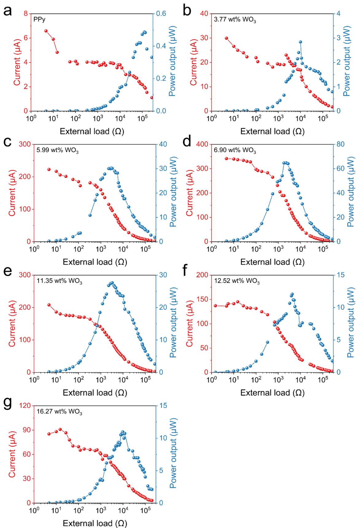
**Fig. S12** Dependency of the current and power outputs on external resistances for PPy-WO<sub>3</sub> devices with (a) 0 wt%, (b) 3.77 wt%, (c) 5.99 wt%, (d) 6.90 wt%, (e) 11.35 wt%, (f) 12.52 wt%, (g) 16.27 wt% different WO<sub>3</sub> in the nanocomposite.
