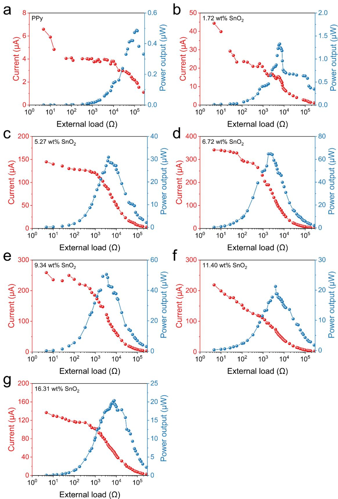
**Fig. S13** Dependency of the current and power outputs on external resistances for PPy-SnO<sub>2</sub> devices with (a) 0 wt%, (b) 1.72 wt%, (c) 5.27 wt%, (d) 6.72 wt%, (e) 9.34 wt%, (f) 11.40 wt%, (g) 16.31 wt% SnO<sub>2</sub> in the nanocomposite.
