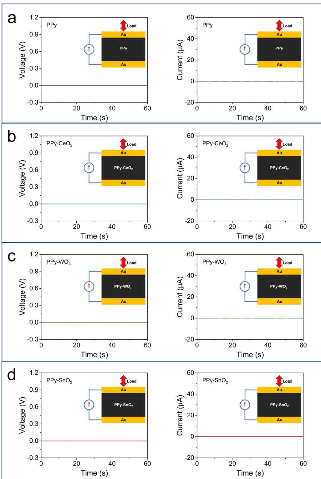
**Fig. S9** Electrical response of (a) Au/PPy/Au, (b) Au/PPy-CeO<sub>2</sub>/Au, (c) Au/PPy-WO<sub>3</sub>/Au, and Au/PPy-SnO<sub>2</sub>/Au devices under repeated compressive deformation (metal oxide content: 7.17 wt%, 6.90 wt%, and 6.73 wt% for PPy-CeO<sub>2</sub>, PPy-WO<sub>3</sub>, and PPy-SnO<sub>2</sub>, strain rate: 6.0%, compressing & releasing speed: 0.035mm s<sup>-1</sup>).
