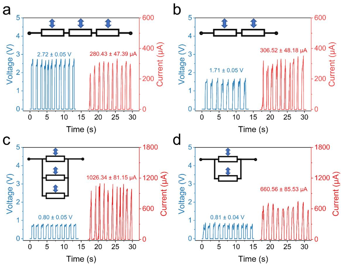
**Fig. S18** Electrical outputs of (a) three and (b) two devices series-connected coin devices. Electrical outputs of (a) three and (b) two devices parallel-connected coin devices.
