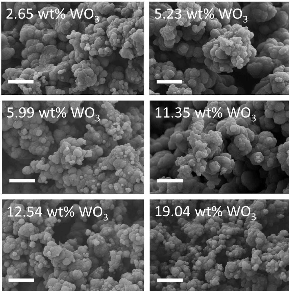
**Fig. S4** SEM images of PPy-WO<sub>3</sub> nanocomposites containing different WO<sub>3</sub> contents (scale bar: 1 μm).
