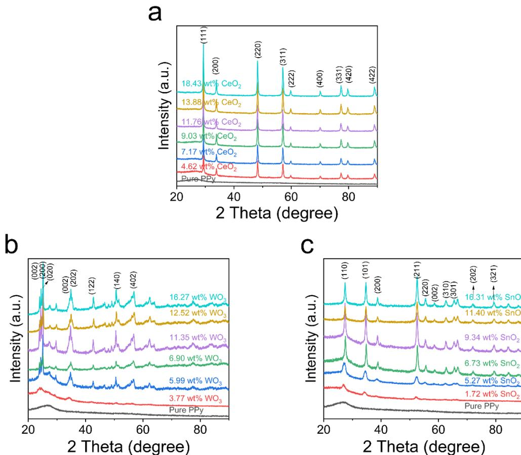
**Fig. S1** XRD patterns of (a) PPy-CeO<sub>2</sub>, (b) PPy-WO<sub>3</sub>, and (c) PPy-SnO<sub>2</sub> nanocomposites with different metal oxide contents.
