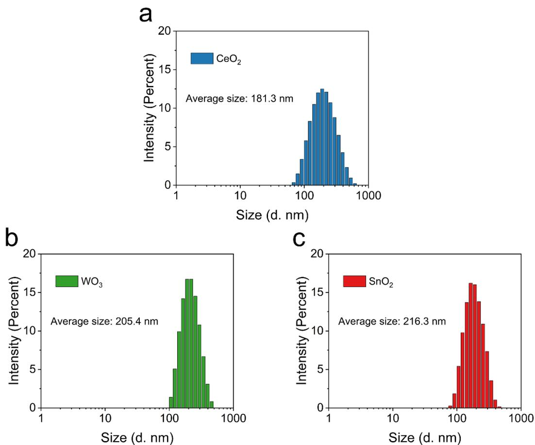
**Fig. S6** Malvern Zetasizer Nano size measurement of (a) CeO<sub>2</sub>, (b) WO<sub>3</sub>, and (c) SnO<sub>2</sub> nanoparticles.
