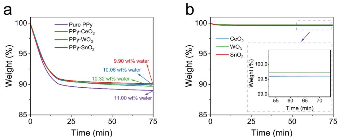
**Fig. S17** (a) Weight loss of PPy and PPy nanocomposites (metal oxide content 7.17 wt%, 6.90 wt%, and 6.73 wt% for PPy-CeO<sub>2</sub>, PPy-WO<sub>3</sub>, and PPy-SnO<sub>2</sub>) at 105 °C, (b) weight loss of three metal oxide powder at 105 °C.
