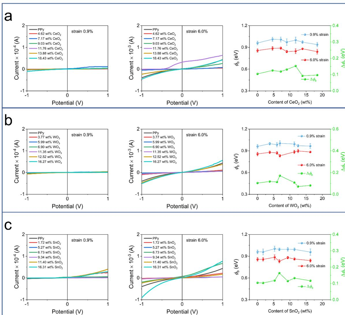
**Fig. S14** I–V curves and calculated Schottky barrier height ( $\phi_b$ ) of (a) PPy-CeO<sub>2</sub>, (b) PPy-WO<sub>3</sub>, and (c) PPy-SnO<sub>2</sub> devices with different metal oxide contents (the Au/PPy-based nanocomposites/Al devices at the strain levels of 0.9% and 6.0%).
