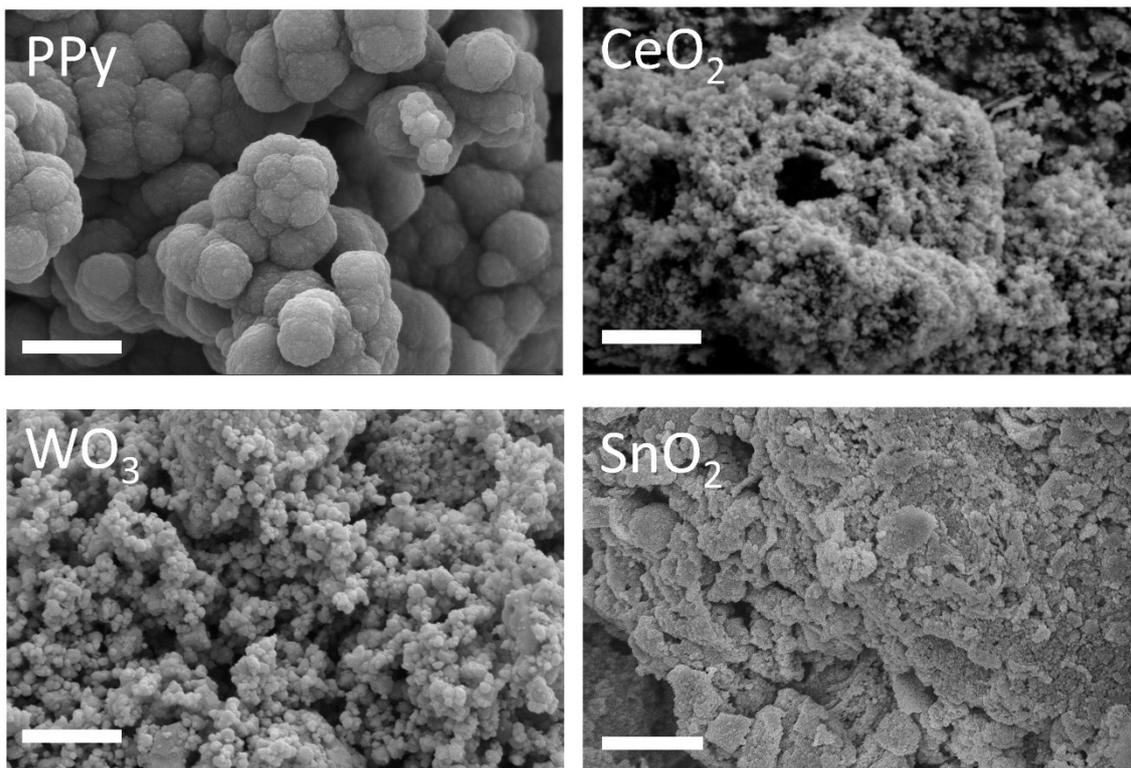
**Fig. S2** SEM images of pure PPy and raw metal oxide materials (CeO<sub>2</sub>, WO<sub>3</sub>, and SnO<sub>2</sub>) (scale bar: 1 μm).
