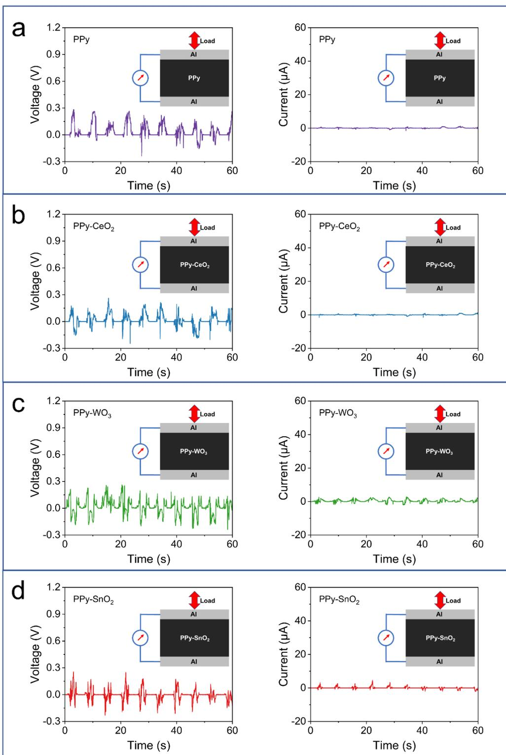
**Fig. S10** Electrical response of (a) Al/PPy/Al, (b) Al/PPy-CeO<sub>2</sub>/Al, (c) Al/PPy-WO<sub>3</sub>/Al, and Al/PPy-SnO<sub>2</sub>/Al devices under repeated compressive deformation (metal oxide content: 7.17 wt%, 6.90 wt%, and 6.73 wt% for PPy-CeO<sub>2</sub>, PPy-WO<sub>3</sub>, and PPy-SnO<sub>2</sub>, strain rate: 6.0%, compressing & releasing speed: 0.035mm s<sup>-1</sup>).
