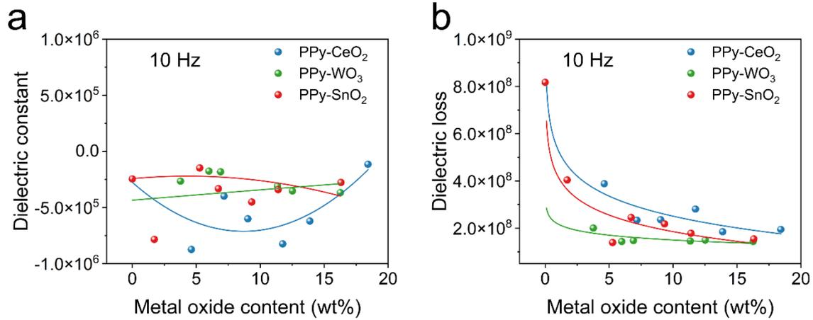
**Fig. S16** Effect of CeO<sub>2</sub>, WO<sub>3</sub>, and SnO<sub>2</sub> content on (a) dielectric constant and (b) dielectric loss of the nanocomposites (at 10 Hz).
