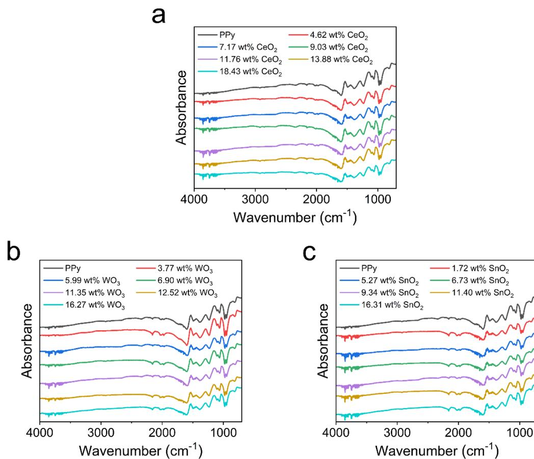
**Fig. S7** FTIR spectra of (a) PPy-CeO<sub>2</sub>, (b) PPy-WO<sub>3</sub>, and (c) PPy-SnO<sub>2</sub> nanocomposites with different metal oxide contents.
