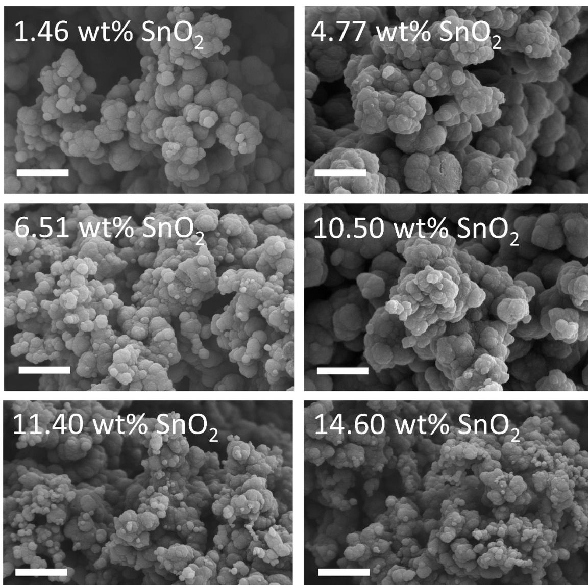
**Fig. S5** SEM images of PPy-SnO<sub>2</sub> nanocomposites containing different SnO<sub>2</sub> contents (scale bar: 1 μm).
