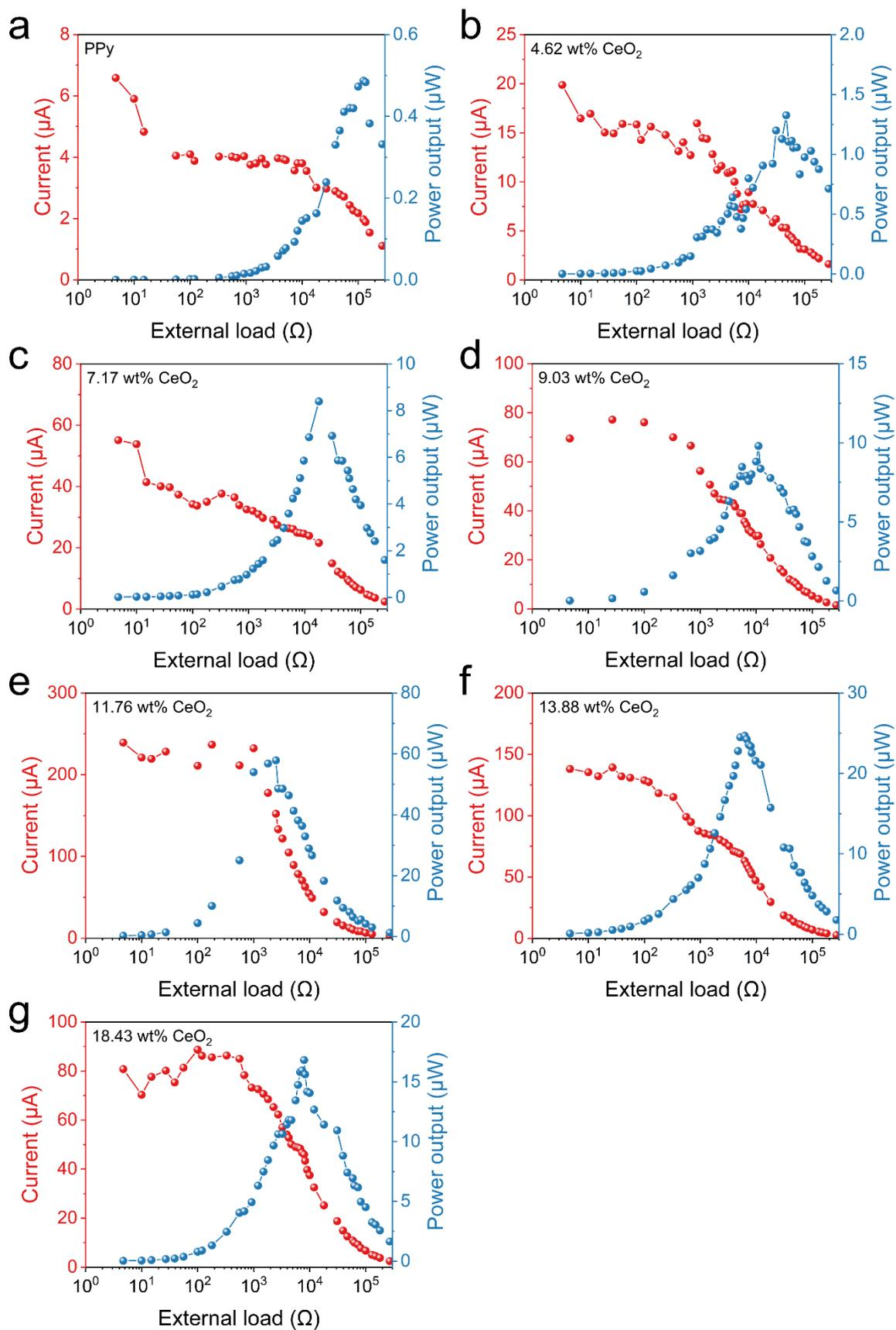
**Fig. S11** Dependency of the current and power outputs on external resistances for PPy-CeO<sub>2</sub> devices with (a) 0 wt%, (b) 4.62 wt%, (c) 7.17 wt%, (d) 9.03 wt%, (e) 11.76 wt%, (f) 13.88 wt%, (g) 18.43 wt% CeO<sub>2</sub> in the nanocomposite.
