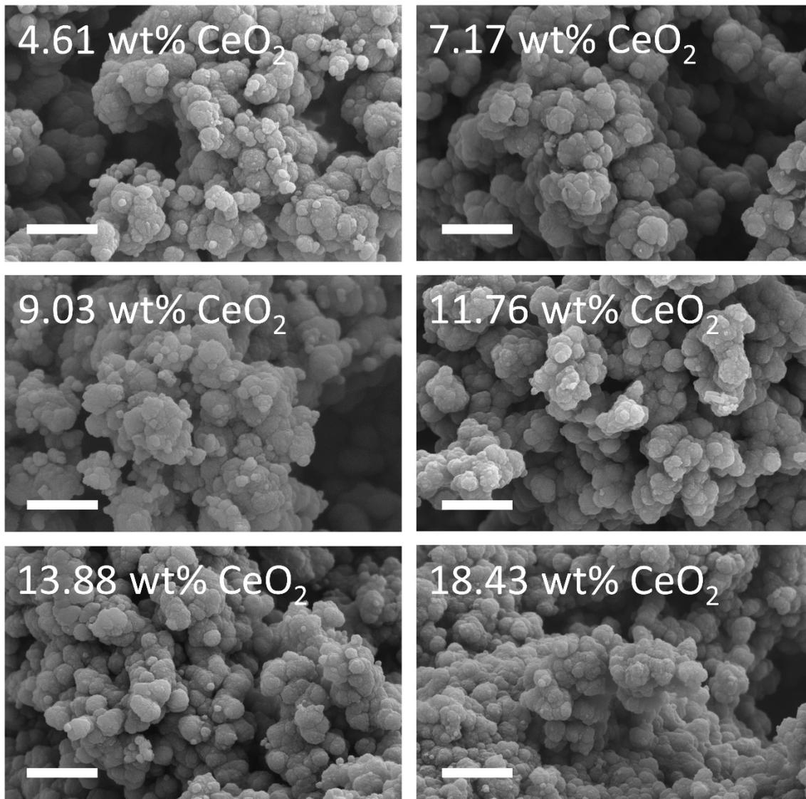
**Fig. S3** SEM images of PPy-CeO<sub>2</sub> nanocomposites containing different CeO<sub>2</sub> contents (scale bar: 1 μm).
