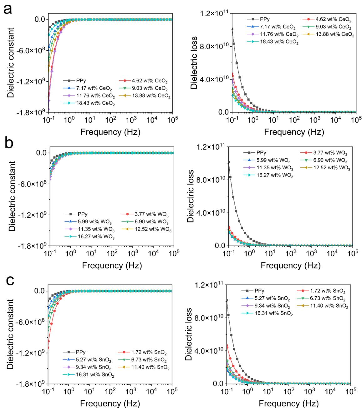
**Fig. S15** The dielectric constant and dielectric loss of (a) PPy-CeO<sub>2</sub>, (b) PPy-WO<sub>3</sub>, and (c) PPy-SnO<sub>2</sub> nanocomposites with different metal oxide contents.
