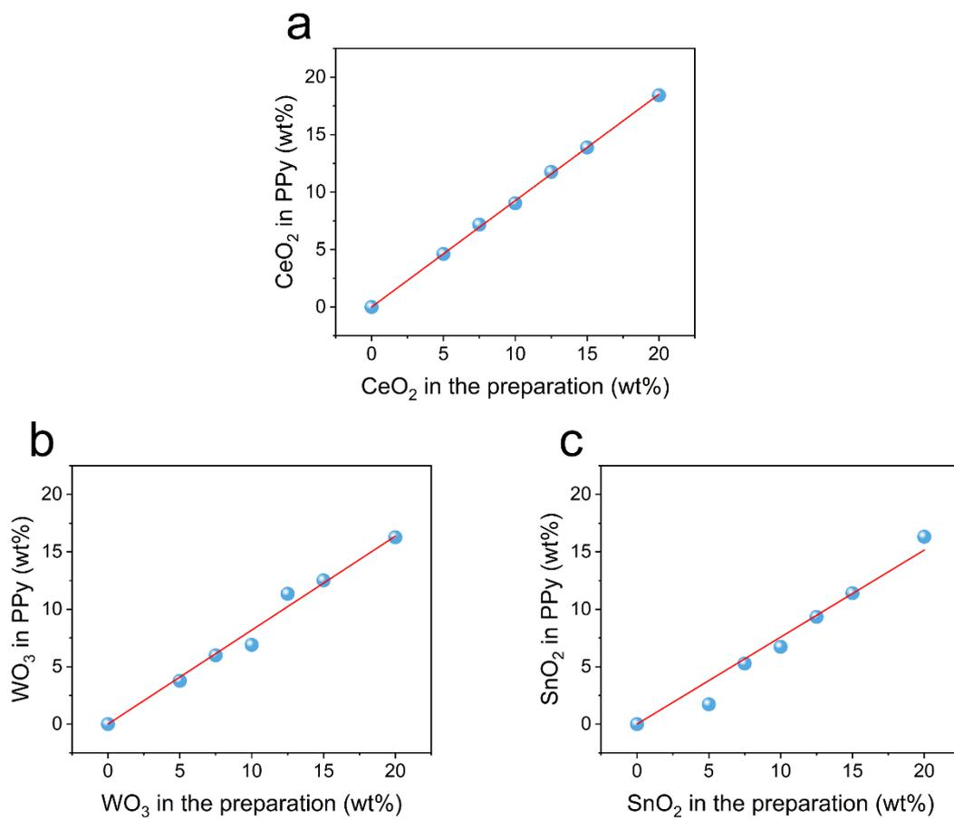
**Fig. S8** Effect of (a)  $\text{CeO}_2$ , (b)  $\text{WO}_3$ , and (c)  $\text{SnO}_2$  content in the PPy synthesis (based on pyrrole) on its actual content in the nanocomposites.
