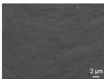
Figure S14. SEM images of the surface for metallic lithium anode with v-NBR/TAC/IL electrolyte after cycling at various current densities from 0.05 to 1 \text{ mA cm}^{-2} at 0.05 \text{ mAh cm}^{-2} at room temperature.
