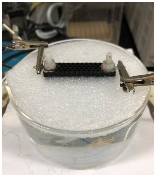
Figure S5 The photo of the MPC/cloth-F device for vapor generation via Joule heat. During the experiment, the DC power supply provides Joule heat, and the resistance of the MPC is suitable for obtaining higher heat under lower voltages. The heat is relatively evenly distributed in the bulk material MPC. Because of the rich pore structure and high specific surface area of MPC, the interfacial evaporation of bulk materials is formed and the effect is excellent.
