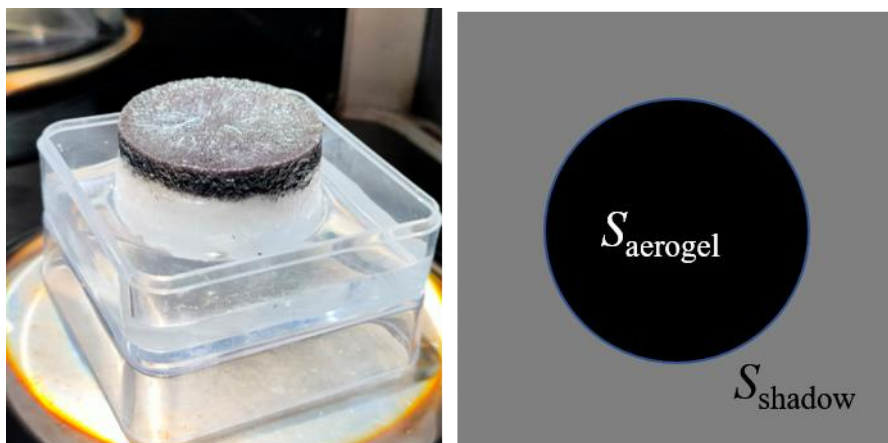
Figure S8 Left: Digital photo of HCE-T 2 during evaporation. Right: diagram of calculation area.
