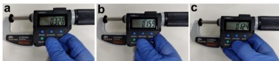
Fig. S17. Thickness of the self-supported rGO pellets fabricated at a) 2 MPa, b) 14 MPa and c) 28 MPa.
