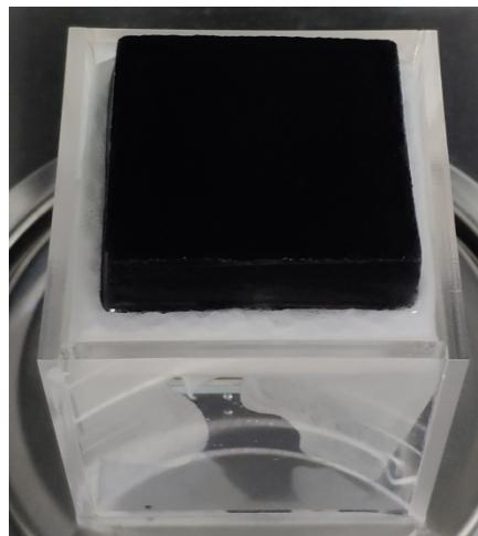
**Figure S4.** The real photo of solar desalination device (Setup2).
