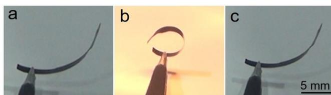
**Figure S18.** Photographs of the PVDF-CB/PEA/PAM actuator (a) before NIR light irradiation, (b) reaching the maximum angle by switching on the light irradiation, and (c) after switching off light irradiation.
