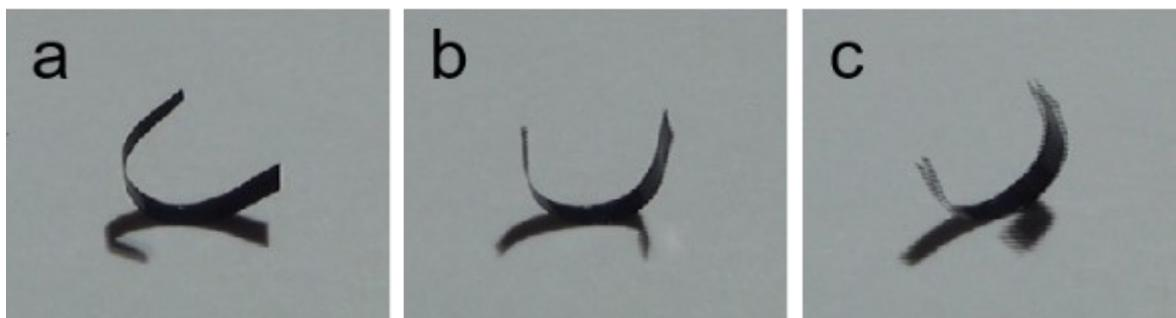
**Figure S37.** Photographs showing oscillatory swing of a curved PVDF-CB/PEA/PAM actuator placed on the surface.
