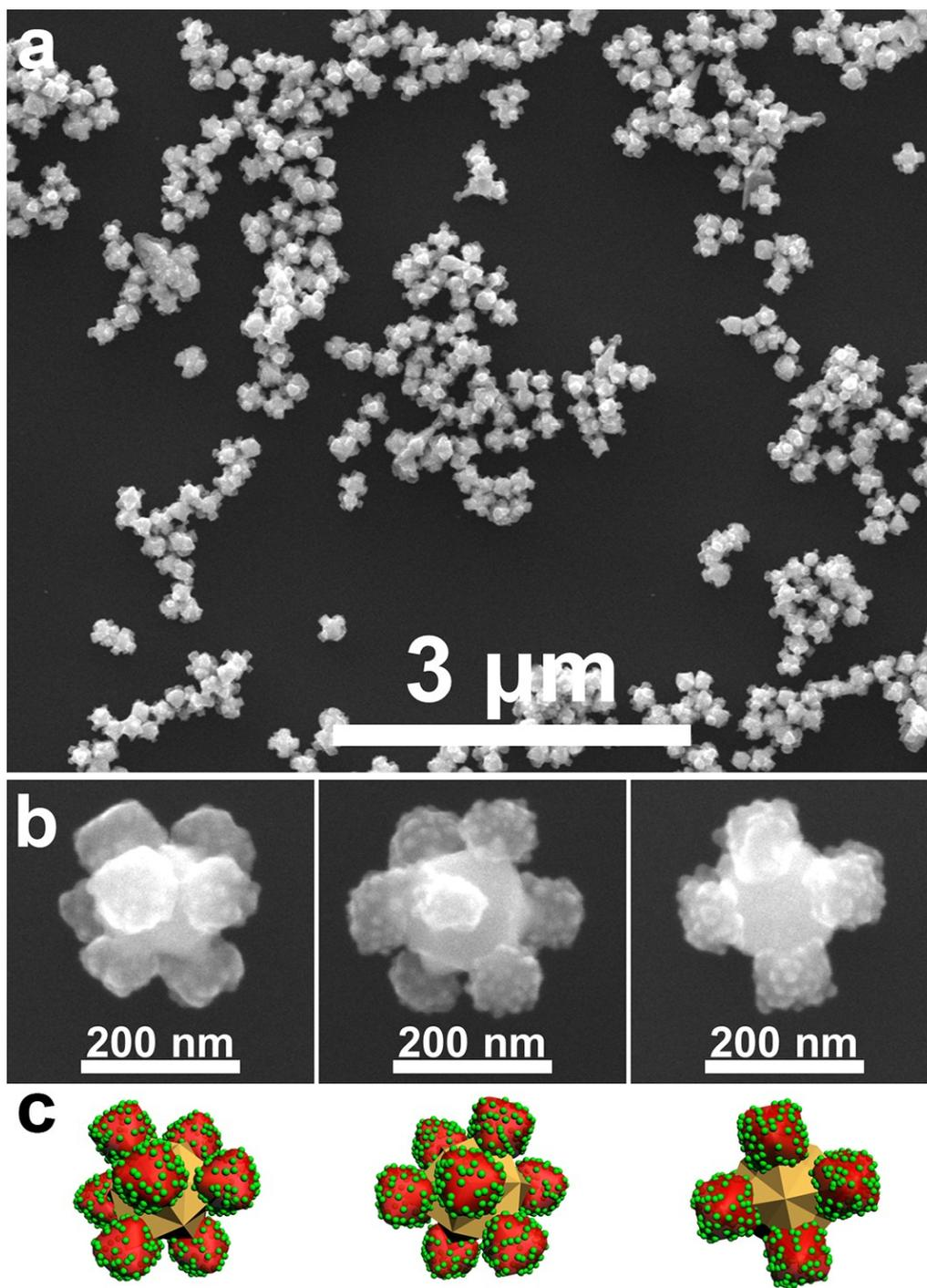
**Fig. S5** (a) Low-magnification SEM image of  $\text{Au}_{\text{vertex}}\text{-Cu}_2\text{O-Ag}$  HNCs. (b) High-magnification SEM images and (c) corresponding three-dimensional geometric models of  $\text{Au}_{\text{vertex}}\text{-Cu}_2\text{O-Ag}$  HNCs viewed along different directions.
