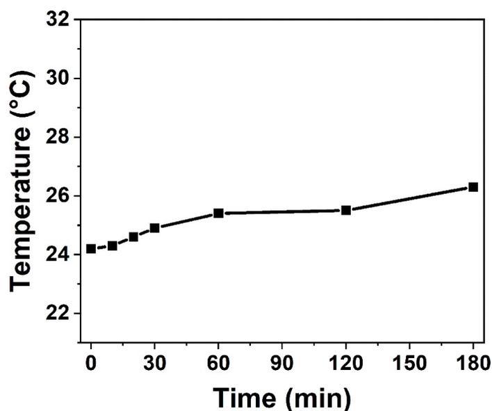
**Fig. S10** Temperature of the reaction mixture during the photocatalysis for Au<sub>vertex</sub>-Cu<sub>2</sub>O-Ag<sub>5.9</sub> HNCs. The temperature was measured by inserting a thermometer (Summit Inc., TPI-330L) into the reaction cell.
