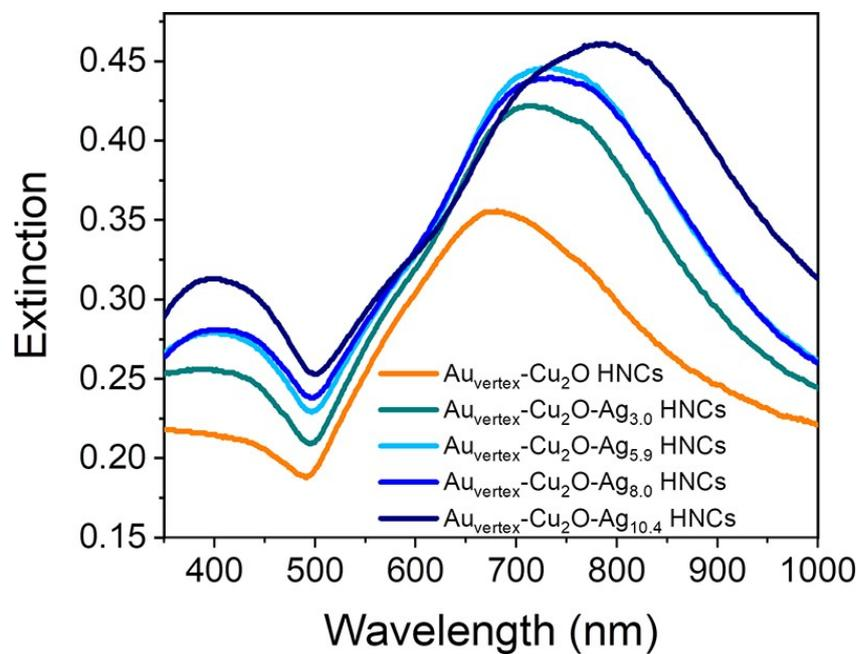
**Fig. S7** Extinction spectra of  $\text{Au}_{\text{vertex}}\text{-Cu}_2\text{O}$  and  $\text{Au}_{\text{vertex}}\text{-Cu}_2\text{O-Ag}$  HNCs.
