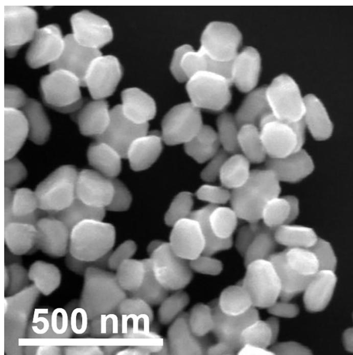
**Fig. S4** SEM image of  $\text{Au}_{\text{vertex}}\text{-Ag}$  HNCs prepared by the reduction of  $\text{AgNO}_3$  on HOH Au NCs in the presence of PVP.
