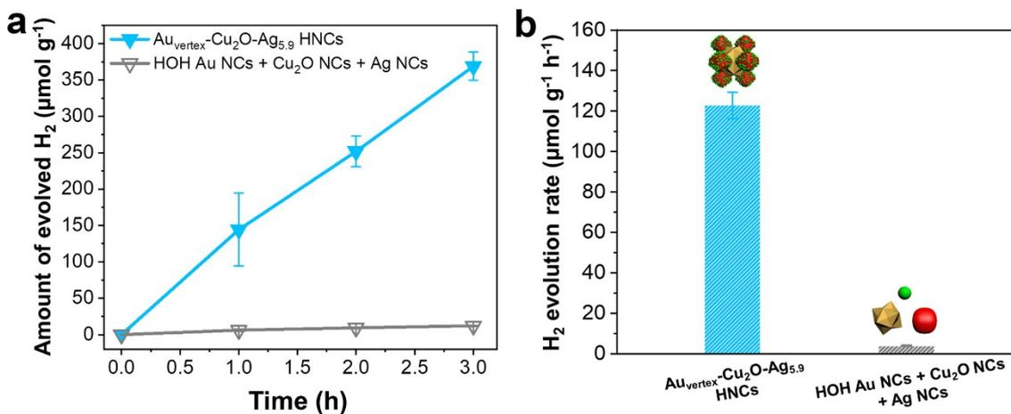
**Fig. S9** (a) Amounts of H<sub>2</sub> evolved during the photocatalysis and (b) corresponding H<sub>2</sub> evolution rates obtained with Au<sub>vertex</sub>-Cu<sub>2</sub>O-Ag<sub>5.9</sub> HNCs and a physical mixture of HOH Au NCs, Ag NCs, and Cu<sub>2</sub>O NCs.
