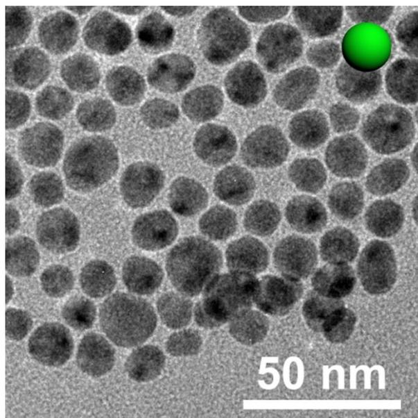
**Fig. S1** TEM image of Ag NCs. Inset shows a three-dimensional geometric model of Ag NCs. The average size of Ag NCs was  $11.9 \pm 1.5$  nm.
