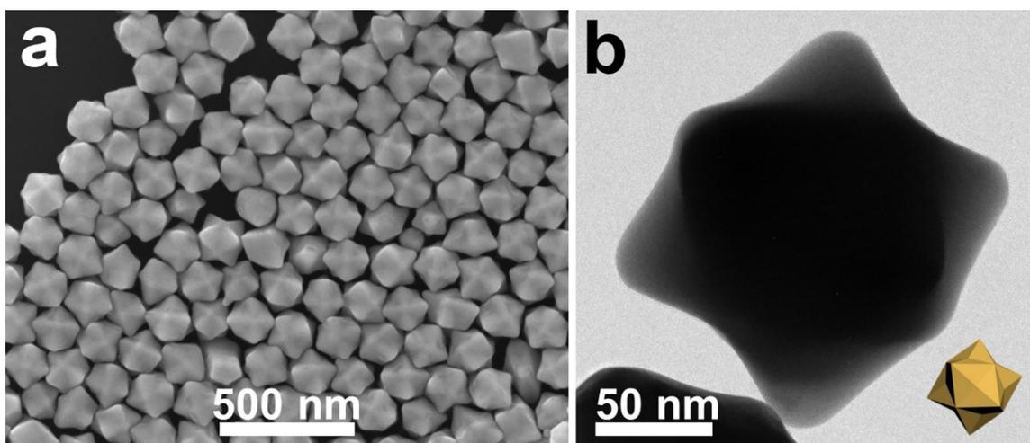
**Fig. S3** (a) SEM and (b) TEM images of HOH Au NCs. Inset in b shows a three-dimensional geometric model of HOH Au NCs. The SEM-determined average size of HOH Au NCs was  $136 \pm 6$  nm.
