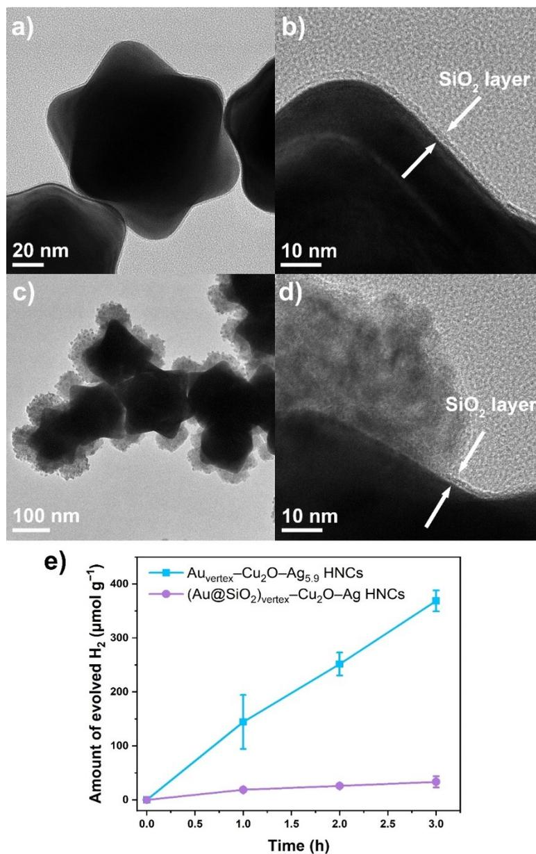
**Fig. S13.** TEM images of (a,b) HOH Au@SiO<sub>2</sub> core-shell NCs and (c,d) (Au@SiO<sub>2</sub>)<sub>vertex</sub>-Cu<sub>2</sub>O-Ag HNCs. (e) Amounts of H<sub>2</sub> evolved during the photocatalysis with Au<sub>vertex</sub>-Cu<sub>2</sub>O-Ag<sub>5.9</sub> and (Au@SiO<sub>2</sub>)<sub>vertex</sub>-Cu<sub>2</sub>O-Ag HNCs, which were normalized to the total mass of catalysts.
