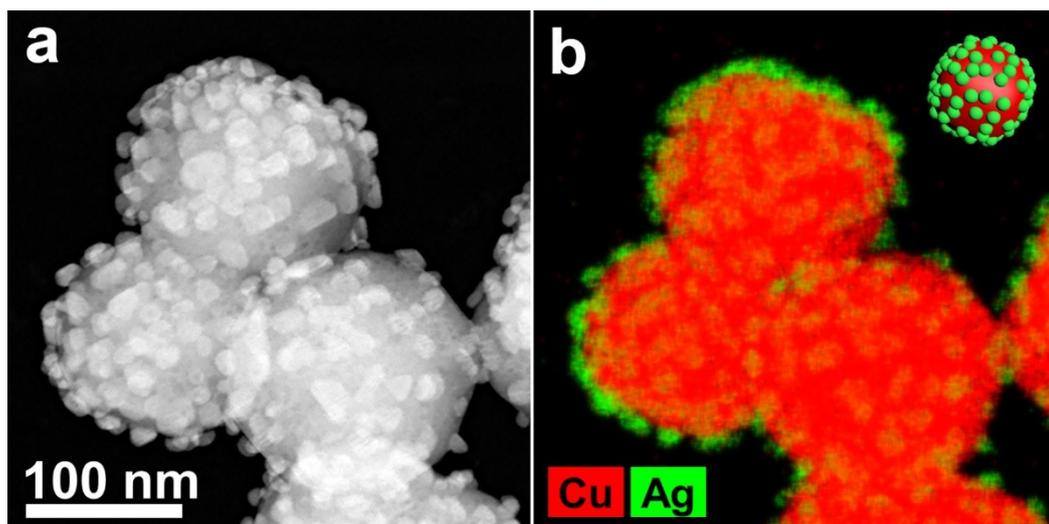
**Fig. S8** (a) HADDF-STEM and (b) corresponding EDS elemental mapping images of  $\text{Cu}_2\text{O}$ -Ag HNCs. Inset in b shows a three-dimensional geometric model of  $\text{Cu}_2\text{O}$ -Ag HNCs.
