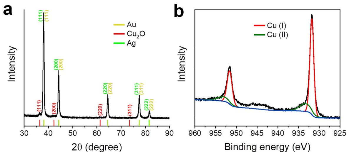
**Fig. S6** (a) XRD pattern of  $\text{Au}_{\text{vertex}}\text{-Cu}_2\text{O-Ag}$  HNCs. The positions of Au,  $\text{Cu}_2\text{O}$ , and Ag references were taken from the ICDD database (Au: 00-004-0784,  $\text{Cu}_2\text{O}$ : 00-005-0667, Ag: 00-004-0783). (b) Cu 2p XPS spectrum of  $\text{Au}_{\text{vertex}}\text{-Cu}_2\text{O-Ag}$  HNCs.
