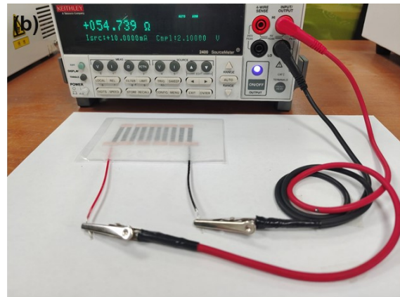
Figure S24 The internal resistance of TEG-XFS16/non-compressed (a) and TEG-XFS16/compressed (b).
