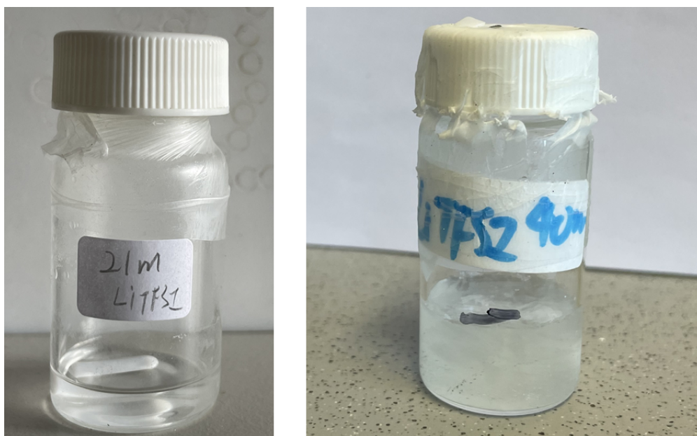
Figure S8. Photos of water-in-salt electrolytes: (left) 21 m, (right) 40 m.
