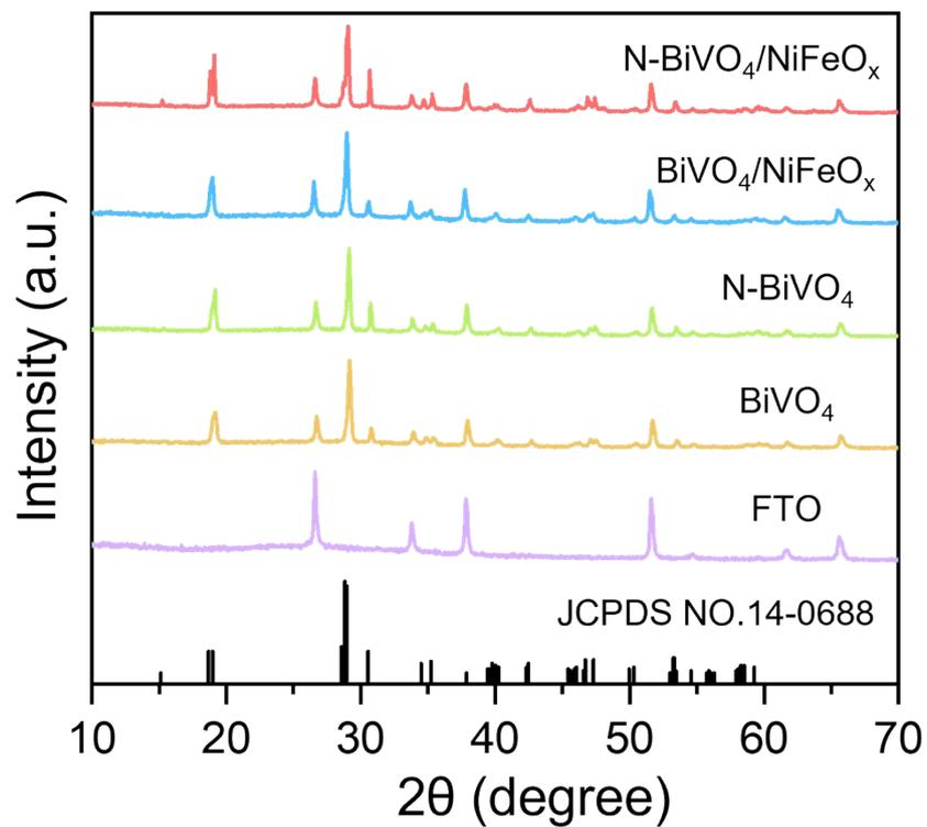
**Fig. S2.** XRD pattern of fluorine-doped SnO<sub>2</sub> (FTO), BiVO<sub>4</sub>, N-BiVO<sub>4</sub>, BiVO<sub>4</sub>/NiFeO<sub>x</sub>, N-BiVO<sub>4</sub>/NiFeO<sub>x</sub>.
