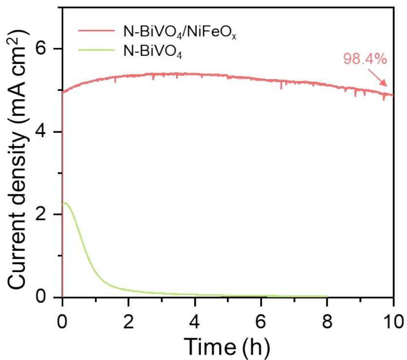
**Fig. S22.** Photocurrent density stabilities of N-BiVO<sub>4</sub>/NiFeO<sub>x</sub> and N-BiVO<sub>4</sub> photoanodes measured in 0.5 M KBi electrolyte at 1.23 V vs. RHE.
