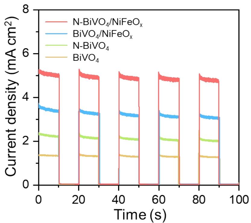
**Fig. S15.** Photocurrent density under chopping irradiation of BiVO<sub>4</sub>, N-BiVO<sub>4</sub>, BiVO<sub>4</sub>/NiFeO<sub>x</sub> and N-BiVO<sub>4</sub>/NiFeO<sub>x</sub> photoanodes.
