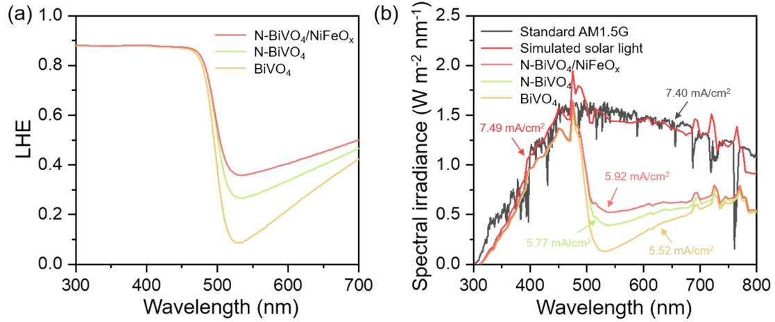
**Fig. S20.** (a) Light harvesting efficiency (LHE) of BiVO<sub>4</sub>, N-BiVO<sub>4</sub> and N-BiVO<sub>4</sub>/NiFeO<sub>x</sub> photoanodes. (b) Spectra of the simulated solar light and corresponding
