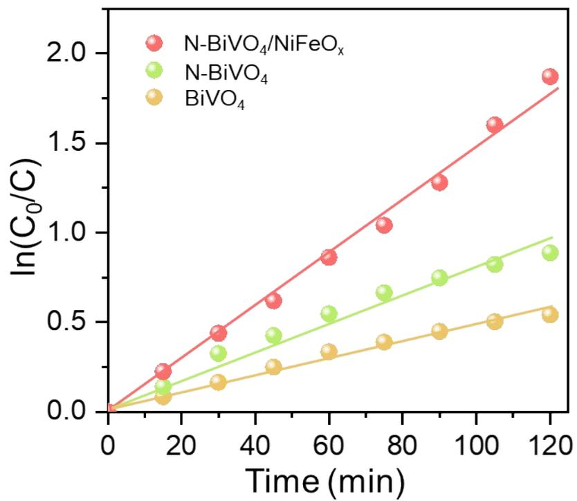
**Fig. S25.** Comparison of PEC kinetic curves of TCH removal by different photoanodes.
