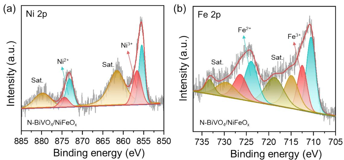
**Fig. S8.** High-resolution XPS spectra of N-BiVO<sub>4</sub>/NiFeO<sub>x</sub>: (a) Ni 2p; (b) Fe 2p.
