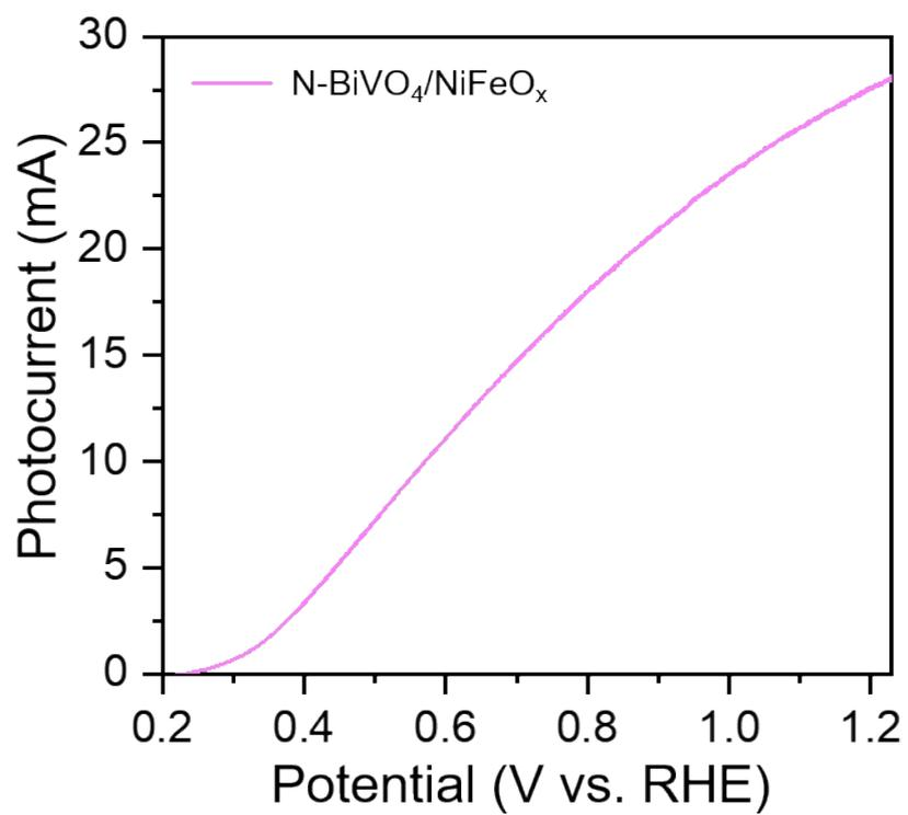
**Fig. S24.** LSV curve of large size N-BiVO<sub>4</sub>/NiFeO<sub>x</sub> photoanode (9 cm<sup>2</sup>).
