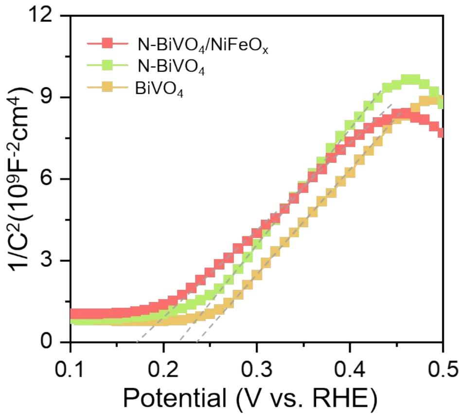
**Fig. S16.** Mott-Schottky curves under dark of BiVO<sub>4</sub>, N-BiVO<sub>4</sub> and N-BiVO<sub>4</sub>/NiFeO<sub>x</sub>.
