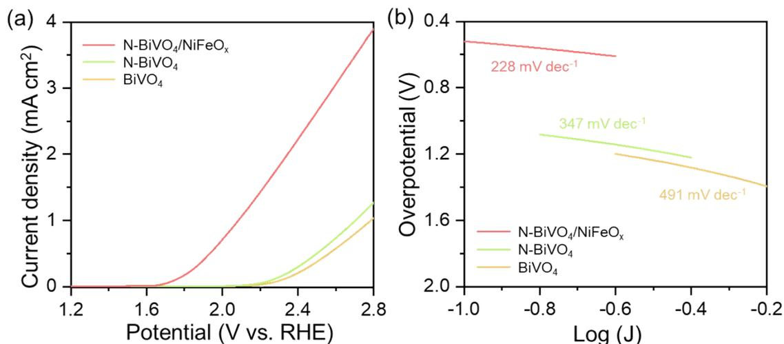
**Fig. S13.** (a) LSV curves in dark for BiVO<sub>4</sub>, N-BiVO<sub>4</sub> and N-BiVO<sub>4</sub>/NiFeO<sub>x</sub>; (b) the estimated Tafel slope for BiVO<sub>4</sub>, N-BiVO<sub>4</sub> and N-BiVO<sub>4</sub>/NiFeO<sub>x</sub>.
