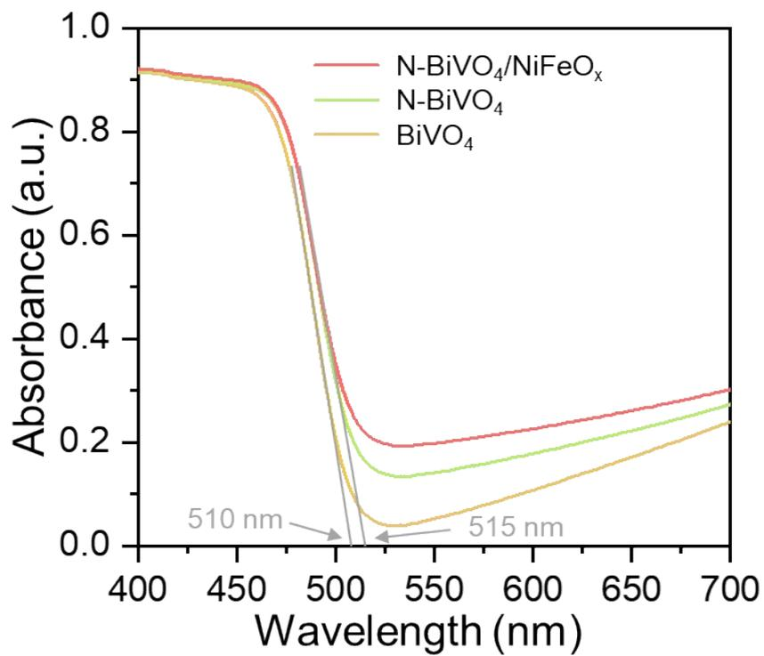
**Fig. S19.** UV-vis absorbance spectrum of BiVO<sub>4</sub>, N-BiVO<sub>4</sub>, and N-BiVO<sub>4</sub>/NiFeO<sub>x</sub> photoanodes.
