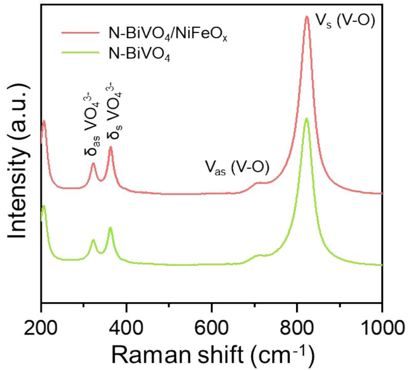
**Fig. S5.** Raman spectra of N-BiVO<sub>4</sub> and N-BiVO<sub>4</sub>/NiFeO<sub>x</sub> photoanodes.
