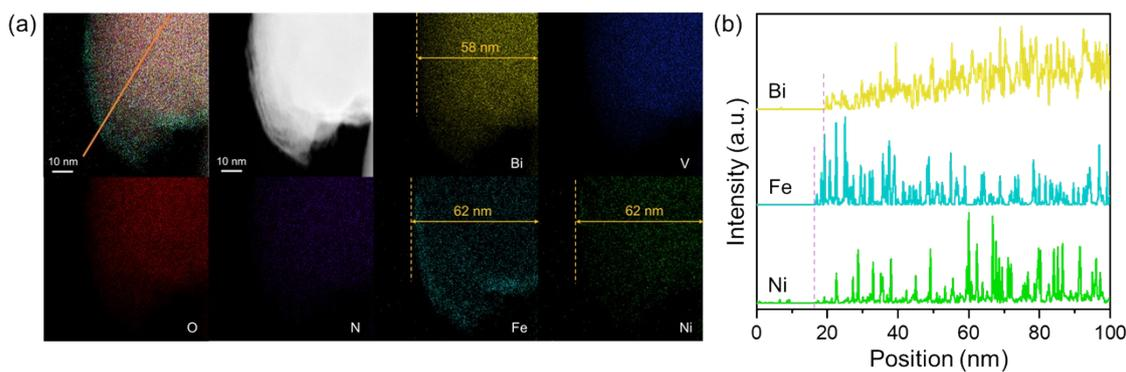
**Fig. S6.** TEM-EDS (a) elemental mapping (b) and line scanning analysis for N-BiVO<sub>4</sub>/NiFeO<sub>x</sub> photoanodes.
