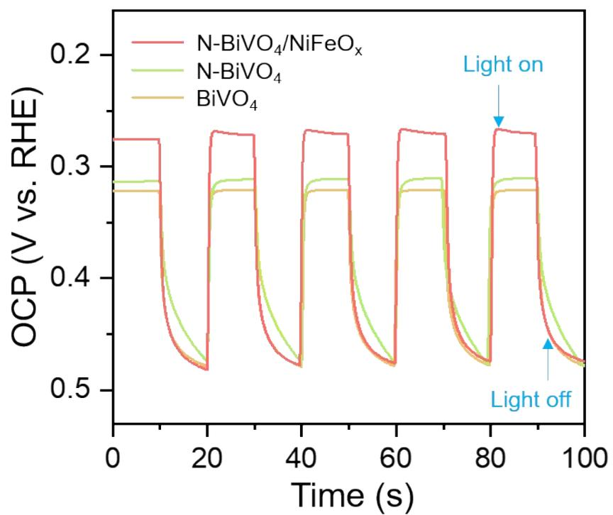
**Fig. S18.** Open-circuit potential under AM 1.5 G illumination in 0.5 M KBi electrolyte (pH=9.3).
