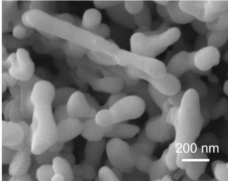
**Fig. S3.** SEM image of the top view of BiVO<sub>4</sub>.
