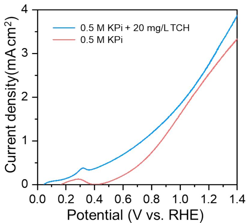
**Fig. S26.** LSV curves of N-BiVO<sub>4</sub>/NiFeO<sub>x</sub> photoanode measured in different electrolytes.
