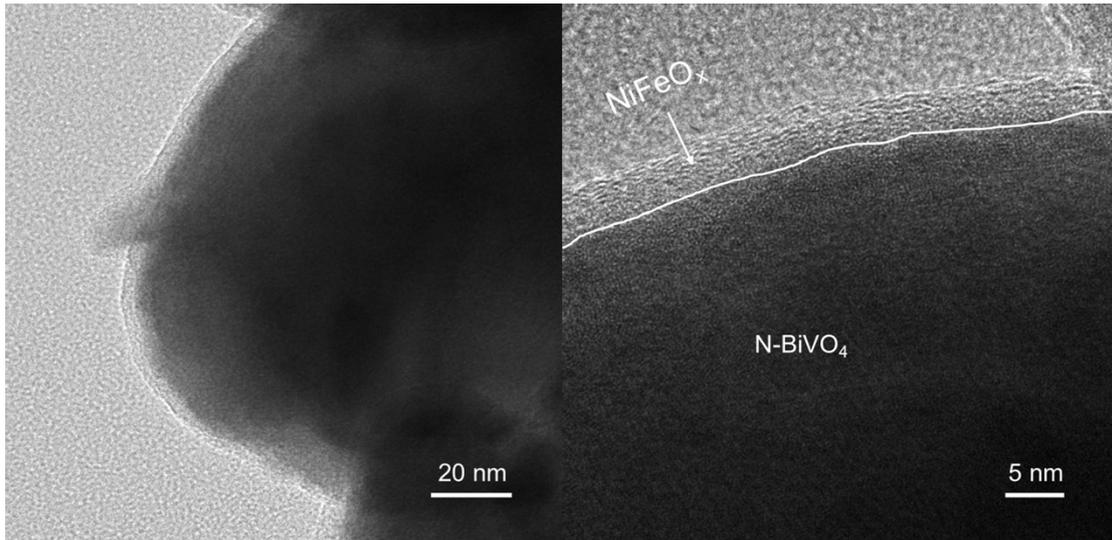
**Fig. S22.** TEM images of N-BiVO<sub>4</sub>/NiFeO<sub>x</sub> photoanode after stability test.
