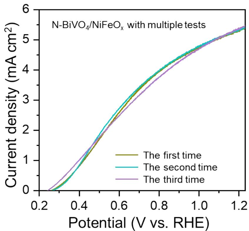
**Fig. S11.** The multiple test LSV curves for N-BiVO<sub>4</sub>/NiFeO<sub>x</sub> photoanodes measured in 0.5 M KBi electrolyte.
