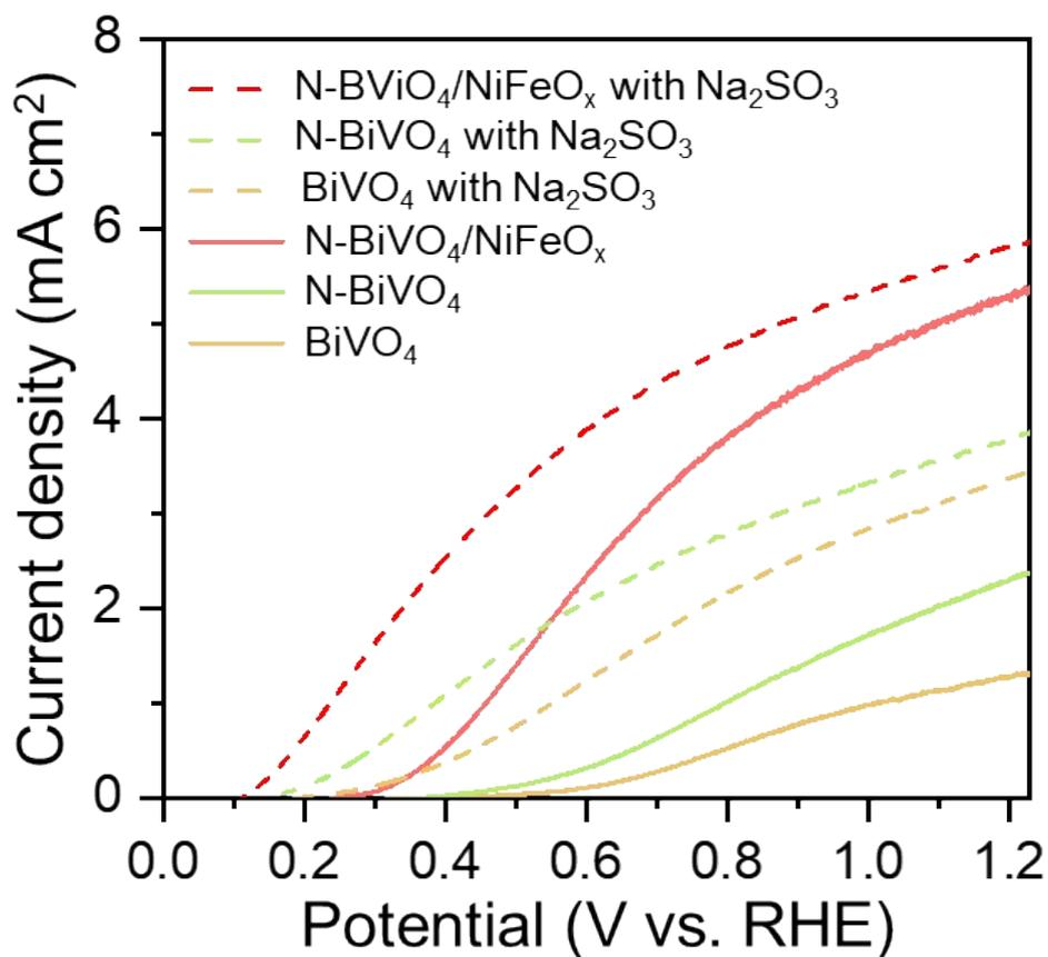
**Fig. S21.** LSV curves of BiVO<sub>4</sub>, N-BiVO<sub>4</sub> and N-BiVO<sub>4</sub>/NiFeO<sub>x</sub> photoanodes in 0.5 M KBi electrolyte with and without hole scavenger (0.5 M Na<sub>2</sub>SO<sub>3</sub>).
