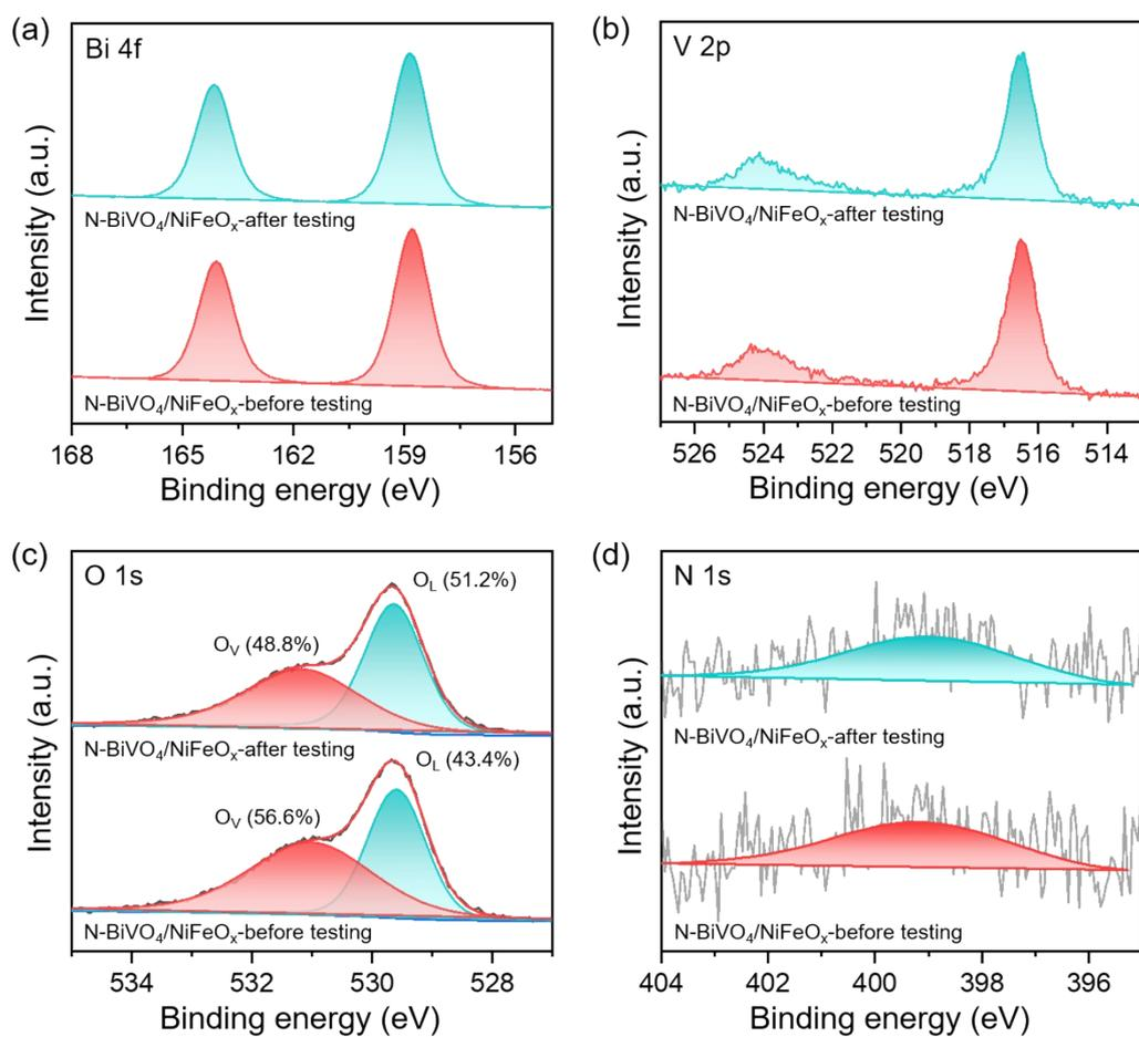
**Fig. S23.** XPS spectra of N-BiVO<sub>4</sub>/NiFeO<sub>x</sub> photoanode before and after PEC measurements (a) Bi 4f; (b) V 2p; (c) O 1s and (d) N 1s.
