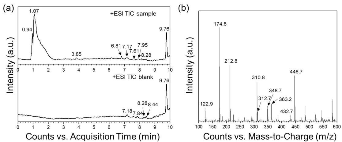
**Fig. S27.** (a) The LC-MS spectra of the TCH solution during degradation by N-BiVO<sub>4</sub>/NiFeO<sub>x</sub> photoanode; and (b) the total spectrum of mass-to-charge ratio (m/z).
