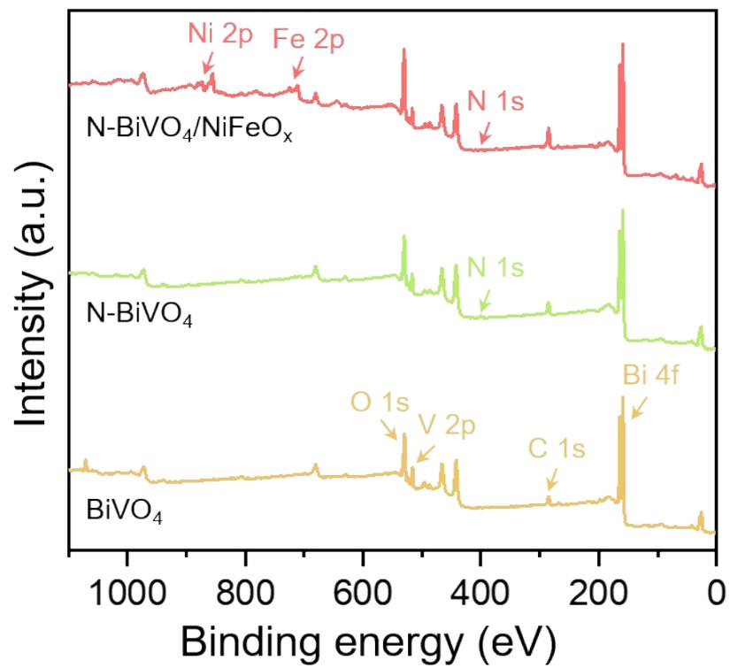
**Fig. S7.** XPS survey scan spectra of BiVO<sub>4</sub>, N-BiVO<sub>4</sub> and N-BiVO<sub>4</sub>/NiFeO<sub>x</sub>.
