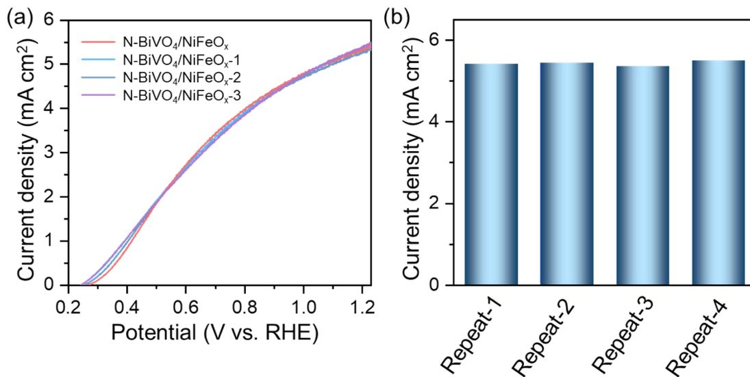
**Fig. S10.** The repeatability of LSV curves for N-BiVO<sub>4</sub>/NiFeO<sub>x</sub> photoanodes measured in 0.5 M KBi electrolyte.
