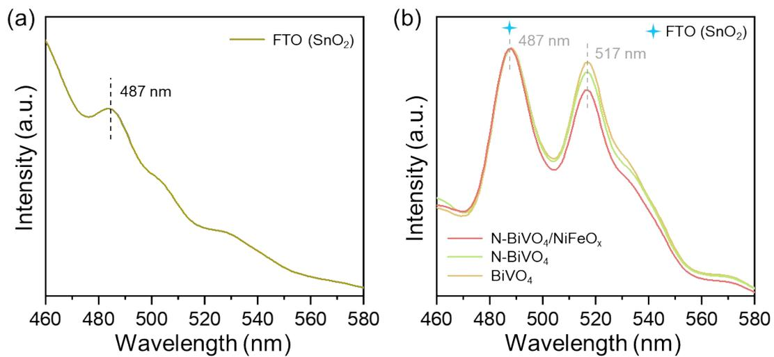
**Fig. S17.** PL spectrum under laser excitation of 380nm: (a) FTO (SnO<sub>2</sub>) substrates; (b) as-prepared photoanodes.
