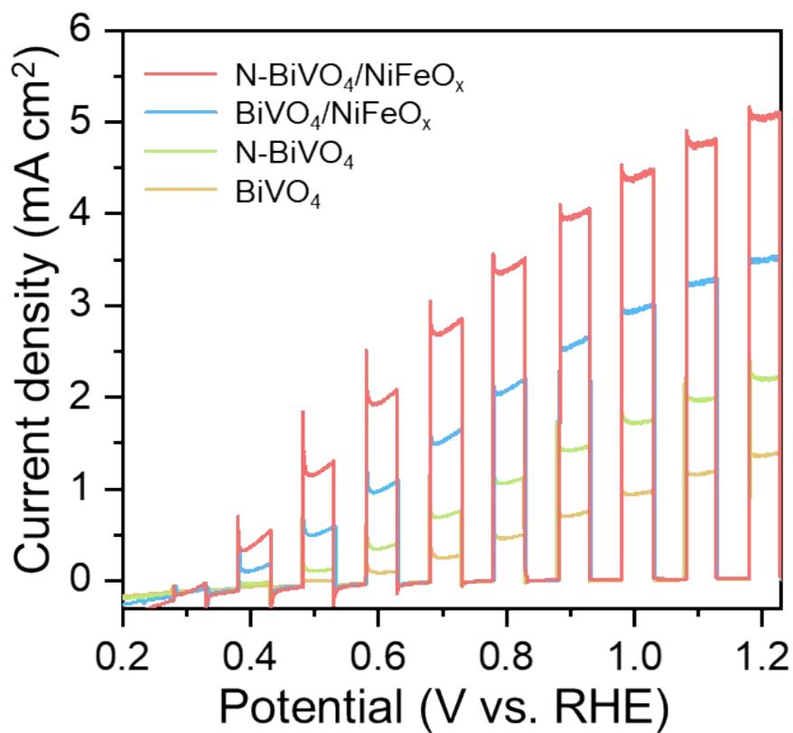
**Fig. S12.** Chopped photocurrent density in 0.5 M KBi electrolyte (pH=9.3).
