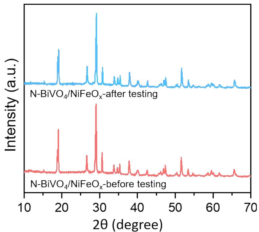
**Fig. S24.** XRD patterns of N-BiVO<sub>4</sub>/NiFeO<sub>x</sub> photoanode before and after stability testing.
