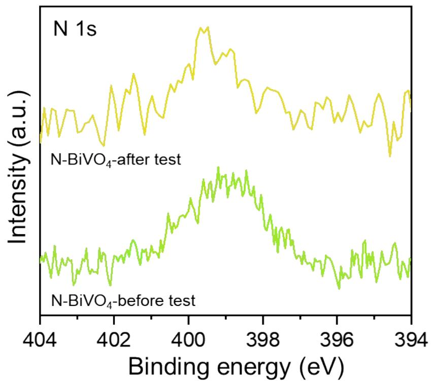
**Fig. S23.** High-resolution XPS spectra of N 1s for N-BiVO<sub>4</sub> before and after test.
