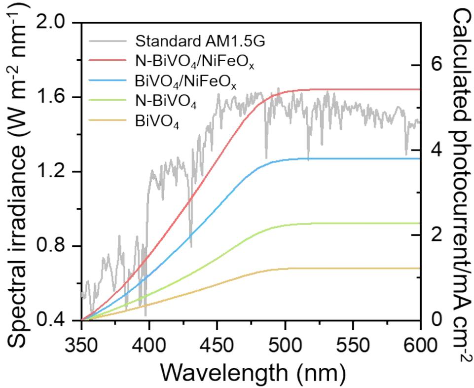
**Fig. S14.** Calculated photocurrent density curves by integrating IPCE curves (Fig. 3c) and the standard AM 1.5G solar spectrum.
