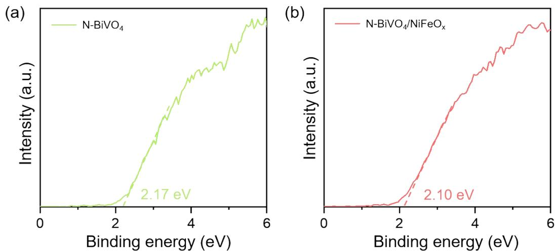
**Fig. S9.** VB XPS of N-BiVO<sub>4</sub> and N-BiVO<sub>4</sub>/NiFeO<sub>x</sub>.
