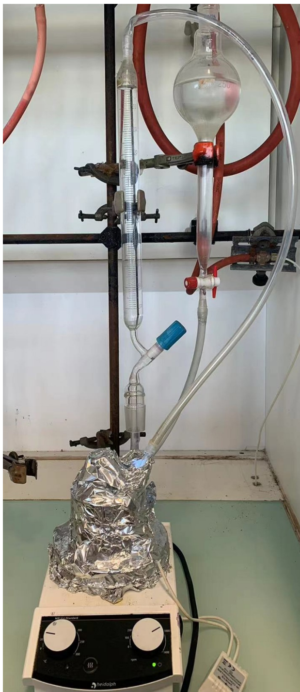
Fig. S2. The reaction for hydrogen generation from ammonia borane methanolysis with visible light irradiation.
