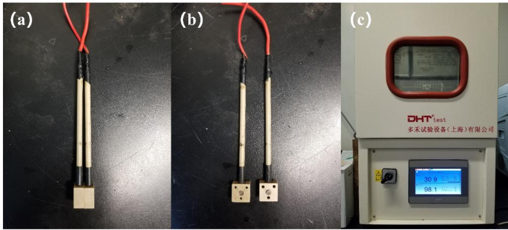
**Fig. S7** Sample preparation and test equipment: (a, b) test electrode, (c) constant temperature and humidity oven.
