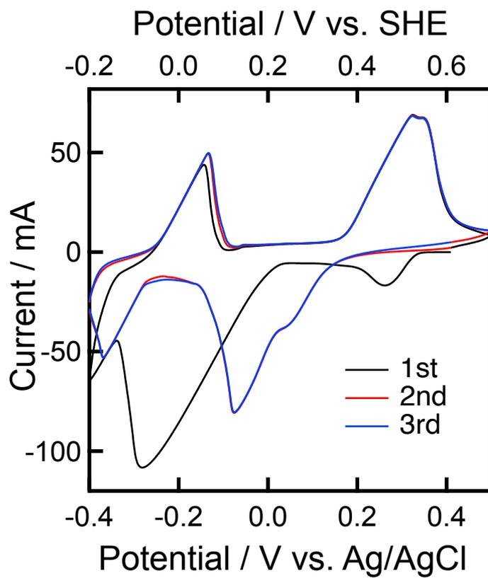
Figure S1. A cyclic voltammogram of the MoO<sub>3</sub> composite electrode at 10 mV sec<sup>-1</sup> in 50 wt% H<sub>2</sub>SO<sub>4</sub> aq.
