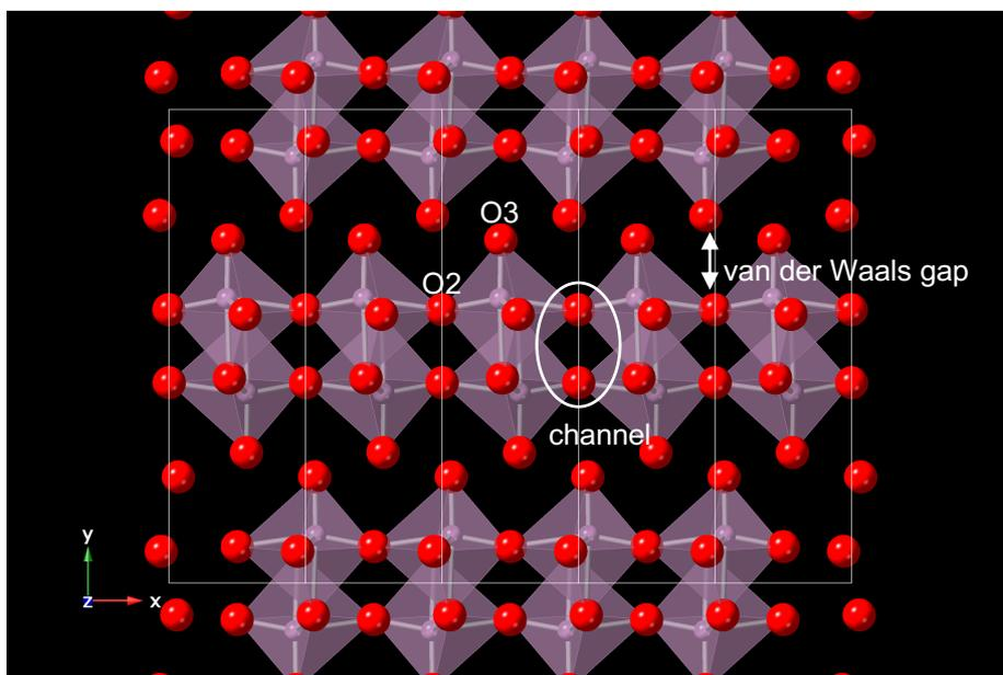
Figure S5. Schematic views of crystal structure of MoO<sub>3</sub>. Purple polyhedral and red spheres denote MoO<sub>6</sub> octahedra and O atoms, respectively.
