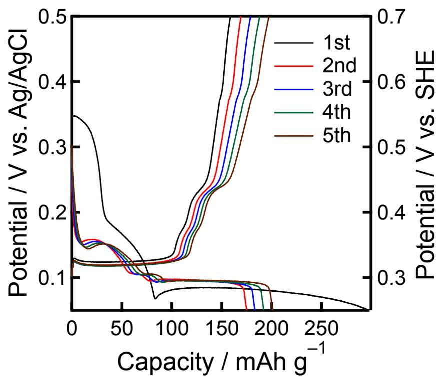
Figure S6. Charge-discharge curves of the MoO<sub>3</sub> electrode in the potential range from 0.05 to 0.50 V at 100 mA g<sup>-1</sup>.
