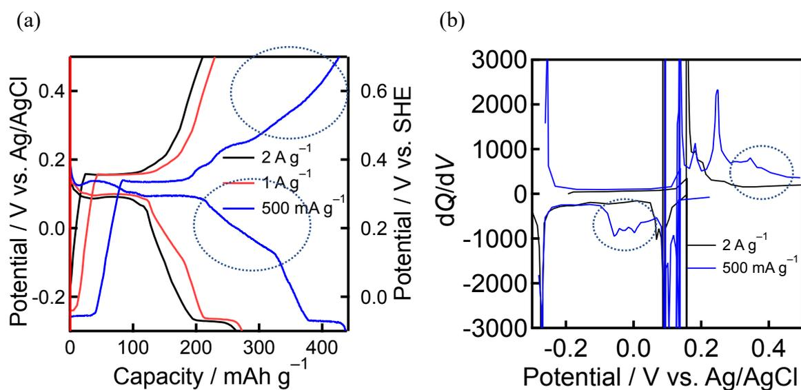
Figure S4. Charge-discharge property of the  $\text{MoO}_3$  electrode in the potential range from  $-0.30$  to  $0.50$  V; (a) charge-discharge curves; (b)  $dQ/dV$  plots. Dotted circles show the redox couple at around  $0.3$  and  $-0.1$  V, which is only observed at low-rate reduction-oxidations ( $< 500 \text{ mA g}^{-1}$ ) as describe in the manuscript.
