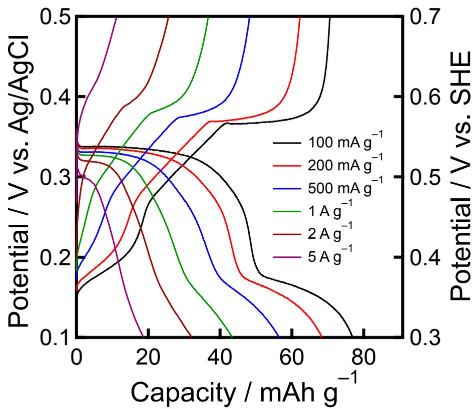
Figure S8. Reduction-oxidation curves of the MoO<sub>3</sub> electrode at different current densities.
