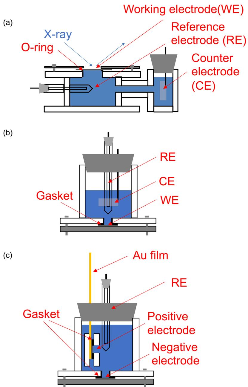
Figure S2. Schematics of electrochemical three-electrode half-cells for (a) operando X-ray diffraction and (b) charge-discharge measurements and (c) electrochemical three-electrode full-cells.
