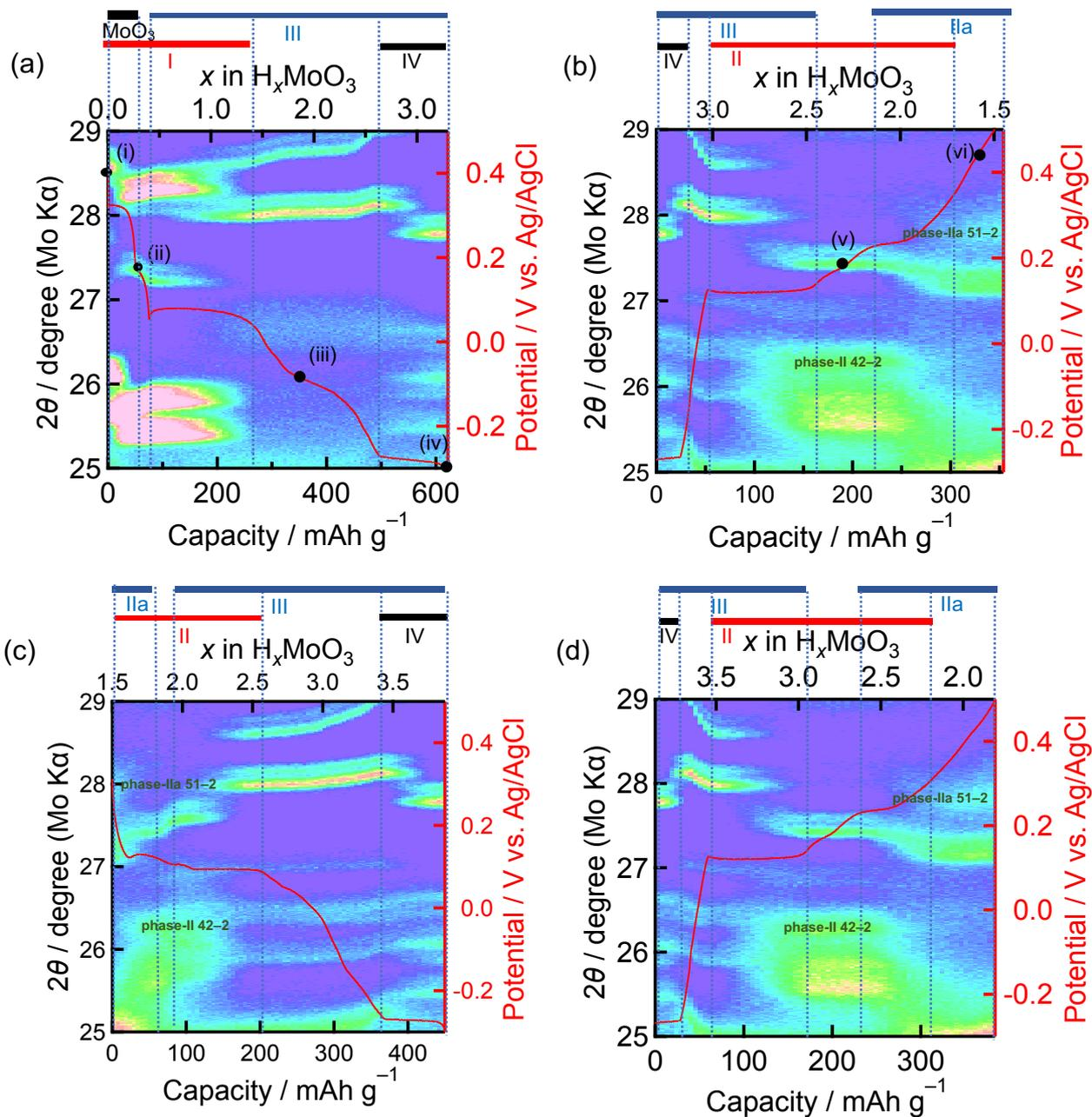
Figure S3. Operando XRD patterns of the  $\text{MoO}_3$  electrode during reduction-oxidation in the potential range from  $-0.30$  to  $0.50$  V at  $100$  mA  $\text{g}^{-1}$ ; contour plots of (a) 1st reduction, (b) 1st oxidation, (c) 2nd reduction, and (d) 2nd oxidation.
