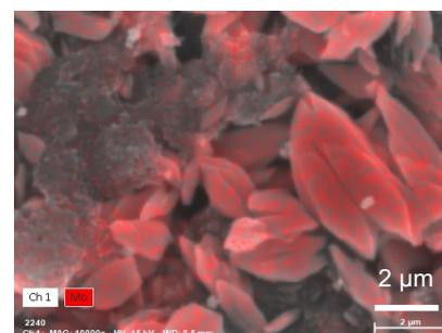
Figure S7. Ex-situ SEM images of the MoO<sub>3</sub> electrodes (upper). EDX maps of Mo element (red) (lower).
