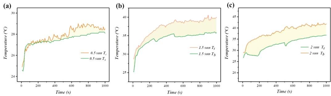
**Fig. S4** Temperatures of the upper and lower surfaces of the GA during SSG under different irradiation intensities.
