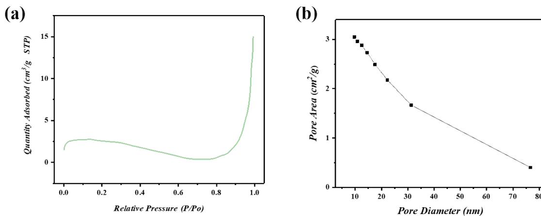
**Fig. S1** (a) N<sub>2</sub> adsorption isotherms of the HGA. (b) Pore area distributions of the HGA calculated by Barrett–Joyner–Hallenda (BJH) method.
