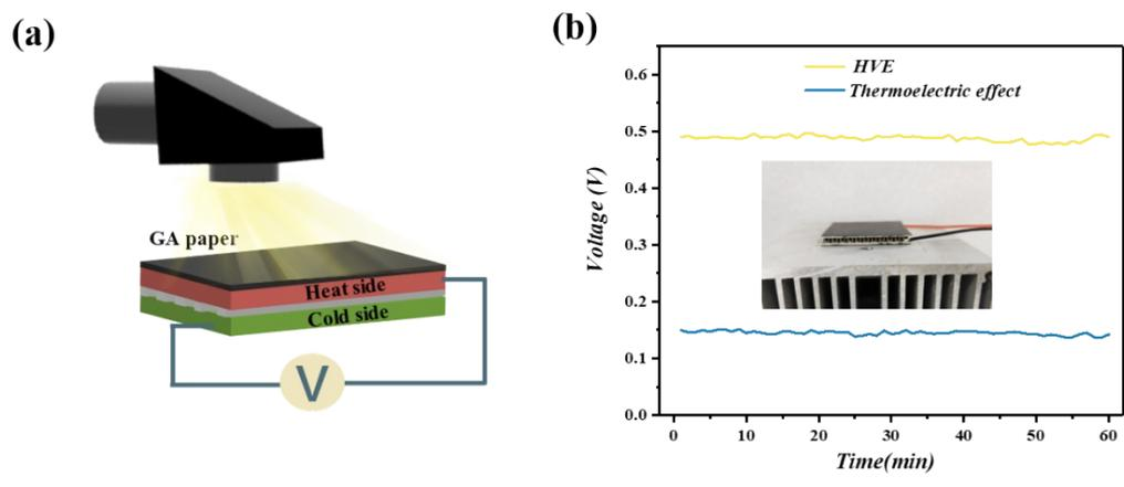
**Fig. S7** (a) Schematic illustration of thermoelectric semiconductor driven by GA paper. (b) Comparison of  $V_{OC}$  generated by thermoelectric effect and HVE under 1 sun irradiation. Inset: Photo of thermoelectric semiconductor.
