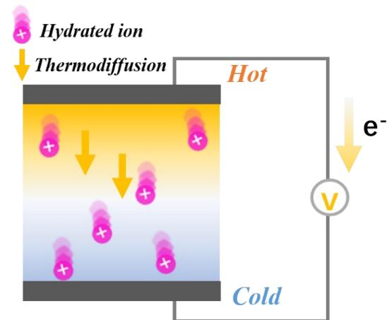
**Fig. S6** Hydrated ions move along the evaporation flow while the thermos-diffusion effect makes the hydrated ions move from the hot to cold electrode.
