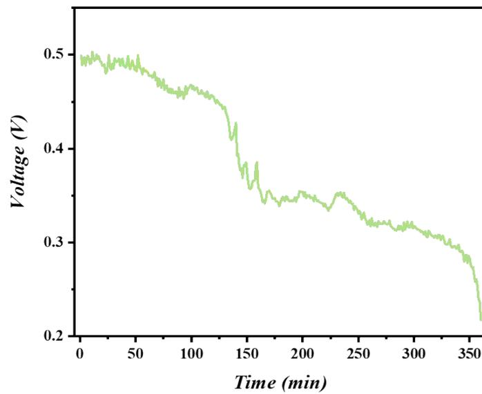
**Fig. S5**  $V_{OC}$  of the HGA in DI water without wind and irradiation. The  $V_{OC}$  gradually decreases from 0.49 V to 0.22 V in 6 h.
