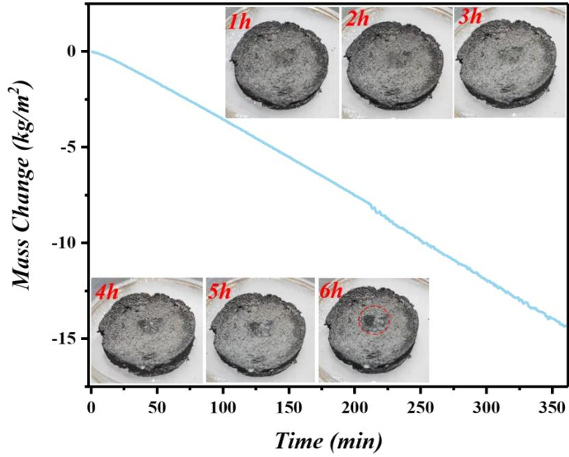
**Fig. S9** Mass change of seawater induced by continuous SSG for 6 h. Inset: Photographs of salt accumulation during the long-term desalination.
