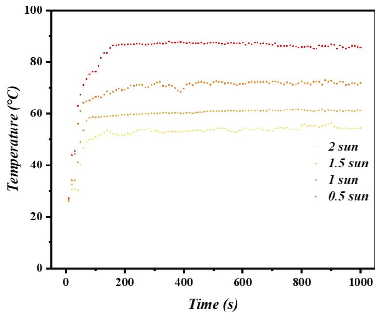
Fig. S3 Temperature rising curves of the pure GA under different solar irradiations.
