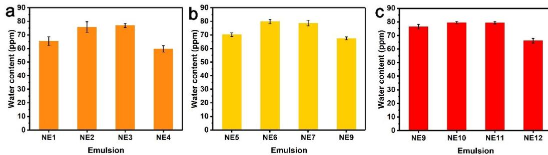
**Fig. S7** (a) Water contents in the filtrates of NE1, NE2, NE3 and NE4 separated by the CFs-superamphiphilic aerogel, (b) water contents in the filtrates of NE5, NE6, NE7 and NE8 separated by the CFs-superamphiphilic aerogel, (c) water contents in the filtrates of NE9, NE10, NE11 and NE12 separated by the CFs-superamphiphilic aerogel.
