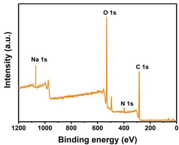
**Fig. S1** XPS survey scan spectrum of the CFs-superamphiphilic aerogel.
