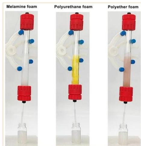
**Fig. S8** Images showing the separation failure of NE1 by melamine foam, polyurethane foam and polyether foam, respectively.
