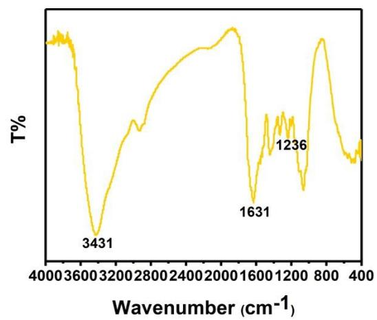
**Fig. S2** FTIR spectra of the CFs-superamphiphilic aerogel.
