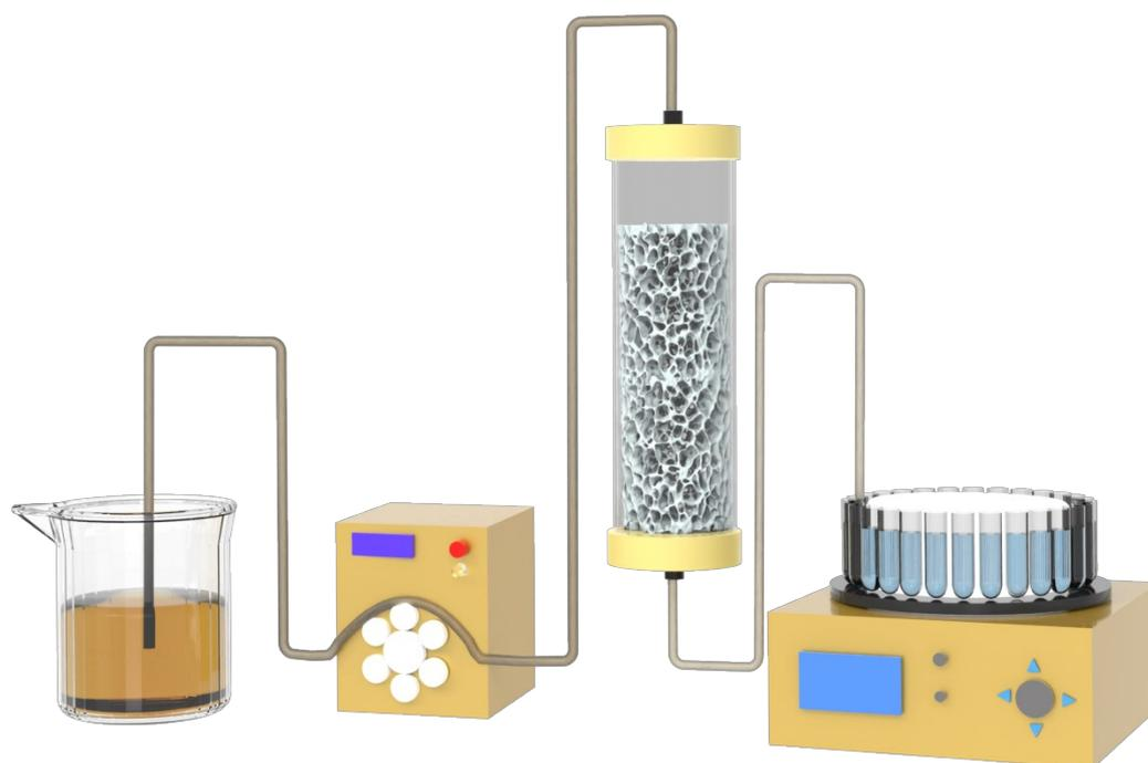
**Fig. S3** Schematic illustration showing the emulsion separation system.
