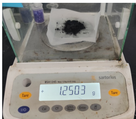
Figure S2. The weighing photograph of the obtained \text{Fe}_4\text{N@N-C} catalyst when the quality of precursors is 6 g.
