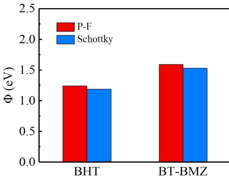
**Fig S3** P-F barrier height and Schottky barrier height of parent materials BHT and BT-BMZ.
