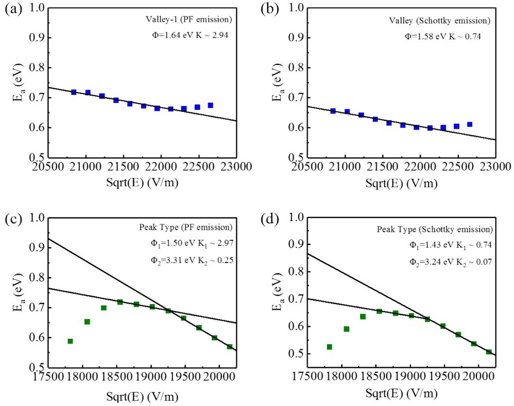
**Fig S7** Plots of  $E_a$  values to extrapolate the barriers height  $\Phi_{P,F}$  for **(a)** the valley-1 film, **(c)** the Peak Type film, and  $\Phi_{\text{Schottky}}$  for **(b)** the valley-1 film, **(d)** the peak Type film.
