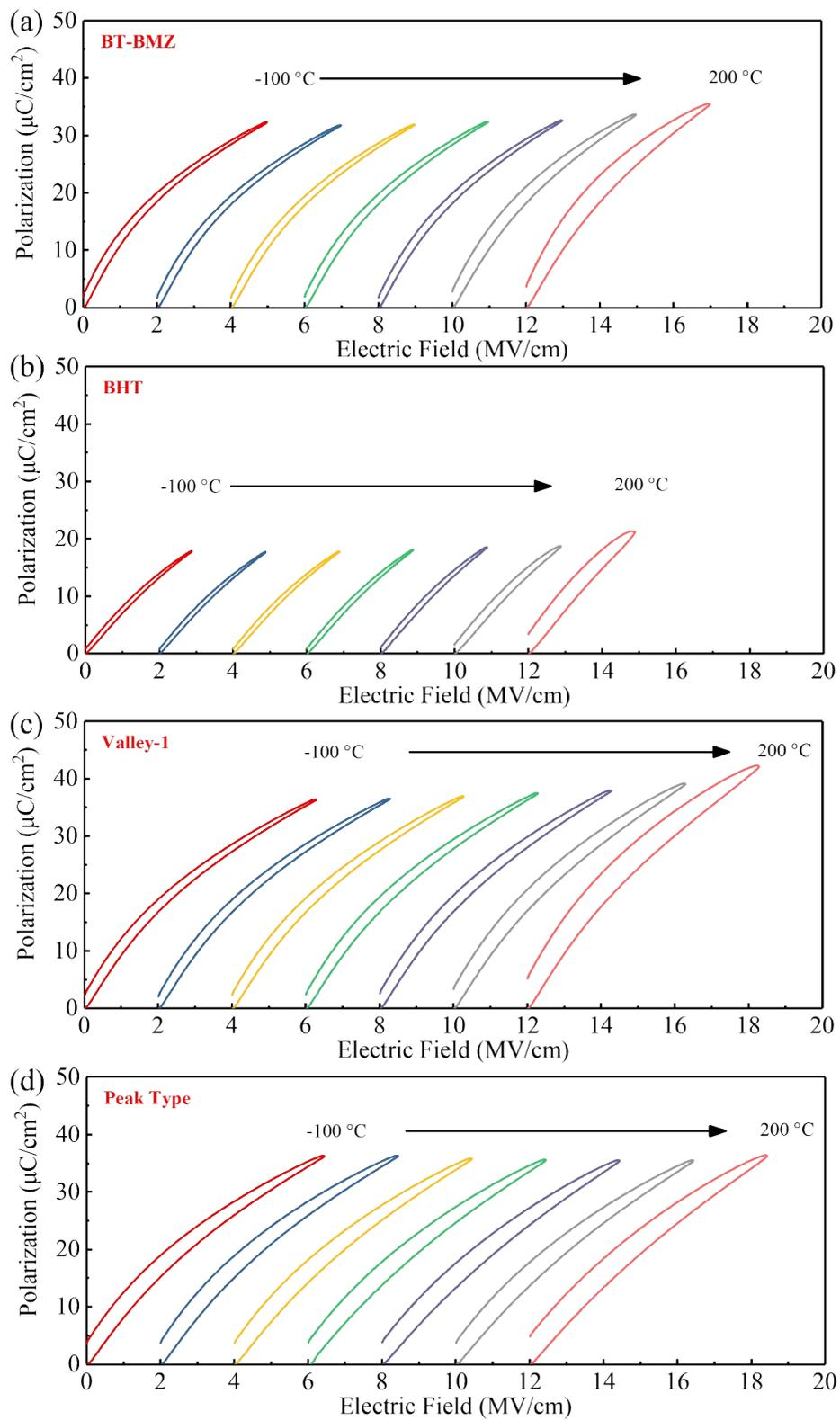
**Fig S10** Unipolar  $P$ - $E$  loops for the films of (a) BT-BMZ, (b) BHT, (c) Valley-1 and (d) Peak Type at 1 kHz at different temperature ( $-100 - 200^\circ\text{C}$ ).
