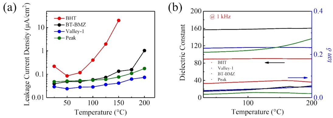
**Fig S11** (a) Leakage current density as a function of temperature under 1.5 MV/cm for BHT, BT-BMZ, Valley-1 and Peak thin films. (b) Dielectric constant and dielectric loss of BHT, BT-BMZ, Valley-1 and Peak thin films as a function of temperature under 1 kHz frequency.
