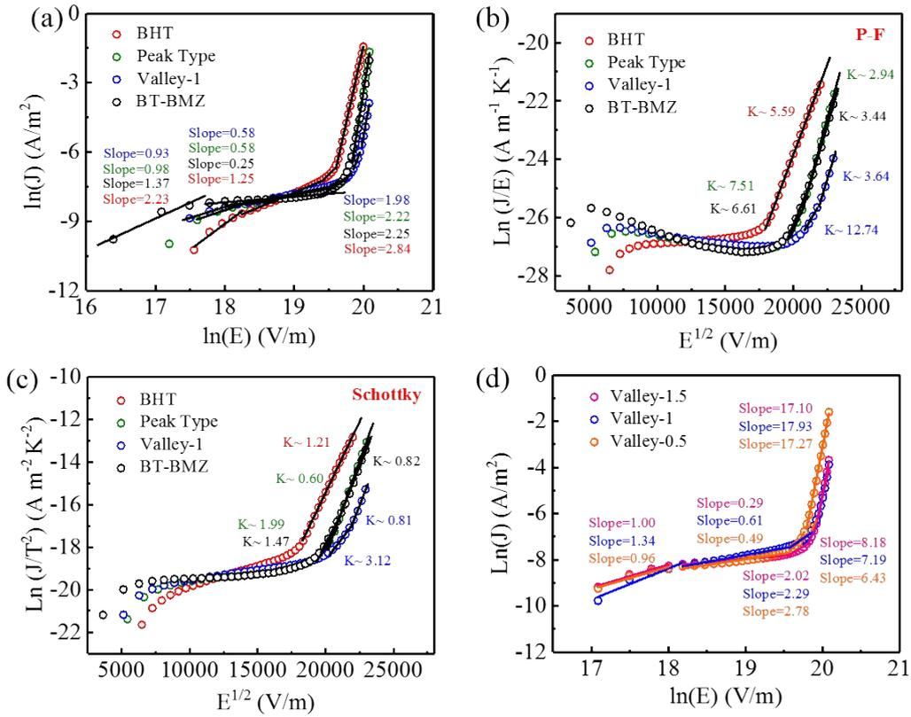
**Fig S5** Fittings of leakage current density of the BHT, Peak Type, Valley-1 and BT-BMZ thin films based on conduction mechanism of (a) ohmic conduction and space charge limited conduction (SCLC), (b) P-F emission, and (c) schottky emission. (d) Fittings of leakage current density of the Valley-1.5, Valley-1, Valley-0.5 thin films based on conduction mechanism of Ohmic conduction and SCLC.
