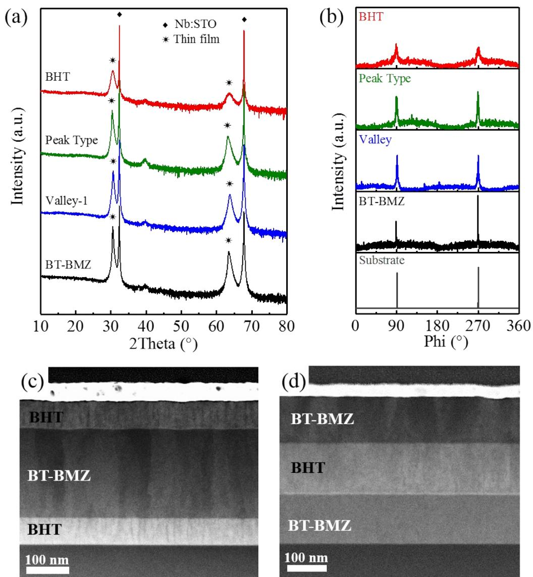
**Fig S4** (a) XRD  $\theta$ - $2\theta$  result of the BHT, Peak Type, Valley-1 and BT-BMZ films. (b)  $\Phi$ -scan result of the BHT, BT-BMZ, Valley-1, Peak type thin films and corresponding substrate around. Cross-sectional STEM images of (c) the Peak Type and (d) the Valley-1 multilayer thin films.
