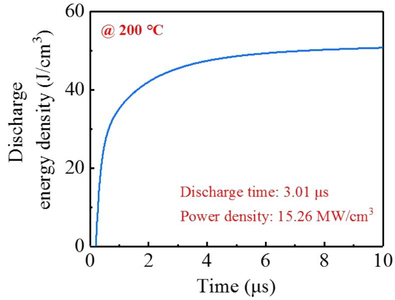
**Fig S12** Discharge energy density as a function of time for the Valley-1 film (Charge electric field is 5.26 MV/cm,  $R_L=10$  k $\Omega$ ).
