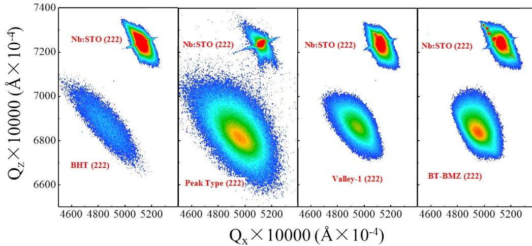
**Fig S8** RSM results of (222) diffraction spots for the BHT, Peak Type, Valley-1 and BT-BMZ thin films.
