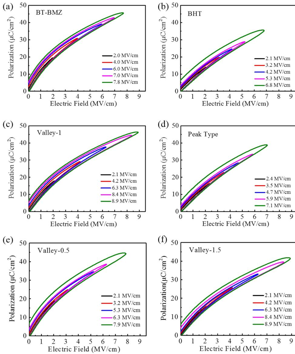
**Fig S9** Unipolar  $P$ - $E$  loops for the films of (a) BT-BMZ, (b) BHT, (c) Valley-1 (d) Peak Type (e) Valley-0.5 and (f) Valley-1.5 at 1 kHz under room temperature.
