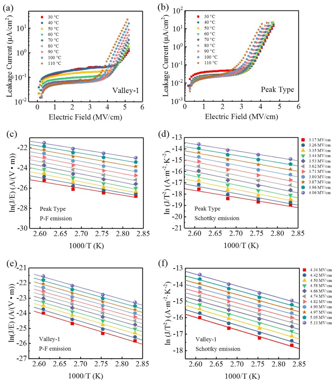
**Fig S6** Leakage current density of **(a)** the Valley-1 and **(b)** Peak Type films as a function of electric field under different temperature. Linear fittings of the temperature-dependent leakage currents to extract thermal activation energies ( $E_a$ ) based on **(c)(e)** P-F emission and **(d)(f)** schottky emission mechanisms.
