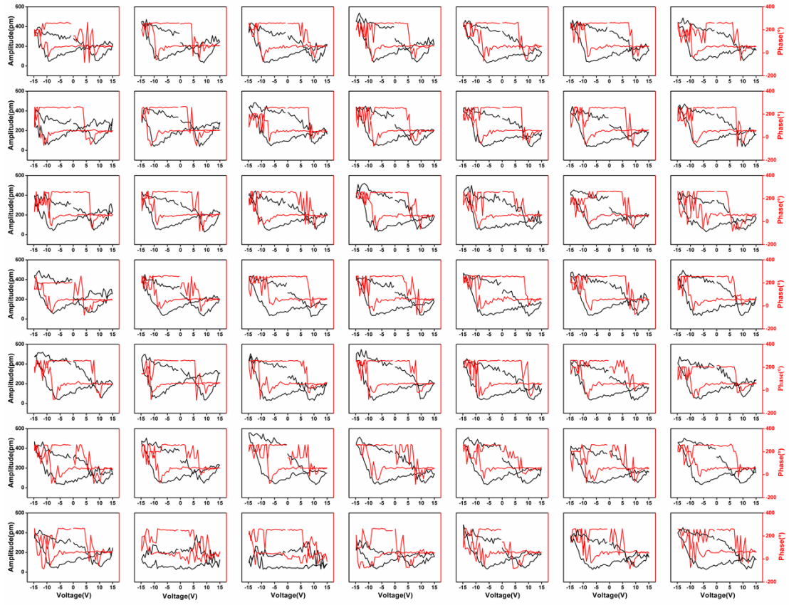
Fig. S3 Typical SS-PFM loops. Amplitude and phase measured at different points with x = 0 .
