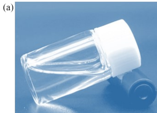
Figure S5. Photographs of the cellulose-ZnCl 2 solution a) and cellulose-ZnCl 2 ionogel b).
