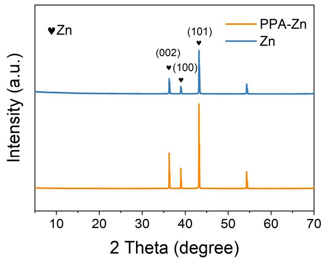
**Figure S6.** XRD patterns of PPA-Zn and Zn foil.
