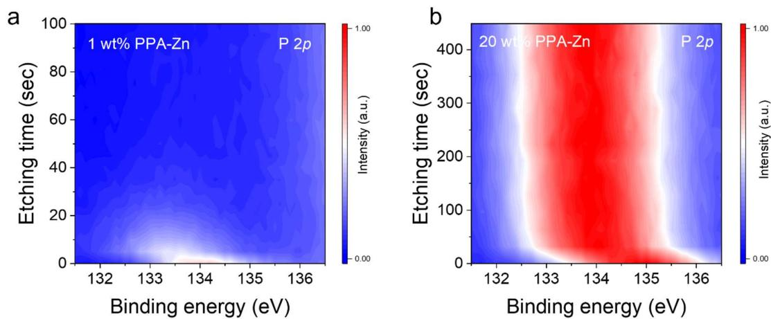
**Figure S5.** The XPS depth profile of P 2p for (a) 1 wt% PPA-Zn and (b) 20 wt% PPA-Zn.
