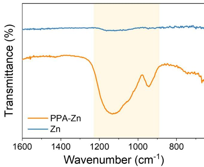
**Figure S4.** FTIR spectra of PPA-Zn and Zn foil.
