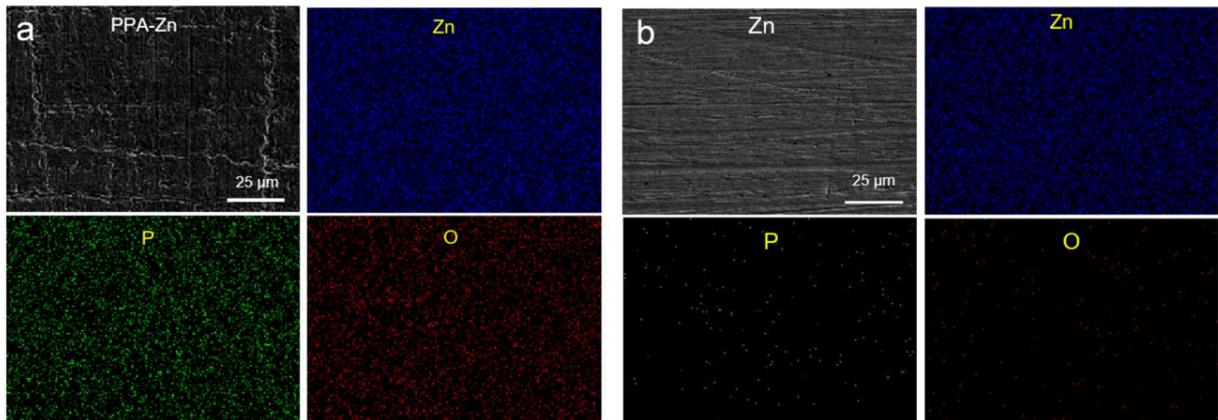
**Figure S3.** Element mapping results obtained by SEM-EDX for (a) PPA-Zn and (b) Zn
