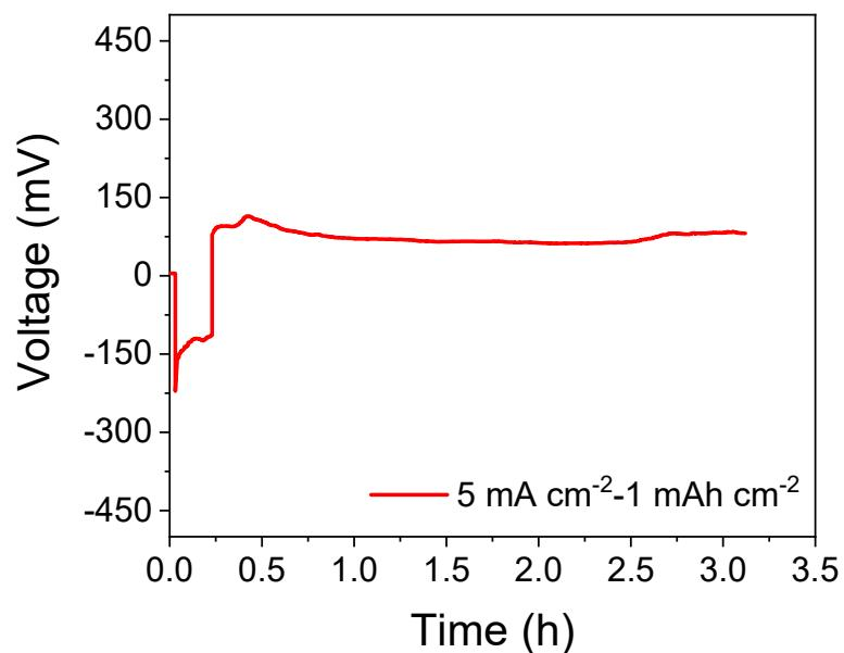
**Figure S9.** The discharge-charge curve of a symmetric cell assembled using PPA-Zn. Because there is Zn at the initial stage, the cut-off voltage cannot reach 0.5 V.
