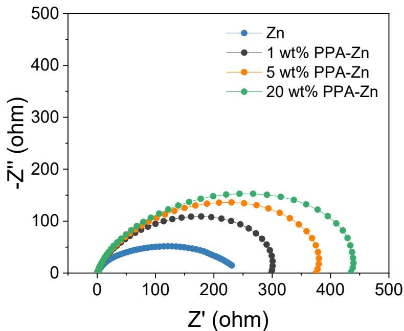
**Figure S1.** EIS profiles of symmetric cells assembled using Zn foils with Zn phosphate protective layers in different thicknesses: bare Zn, 1wt% PPA-Zn, 5wt% PPA-Zn, and 20wt% PPA-Zn.
