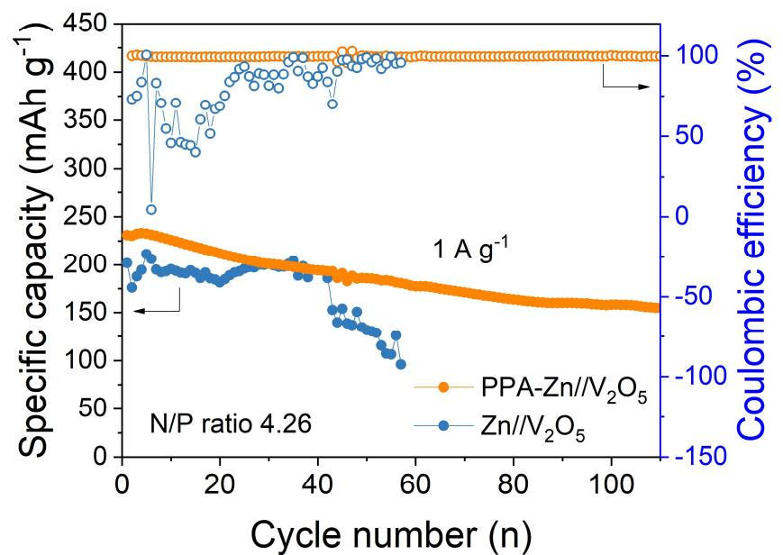
**Figure S10.** The cycle stability of PPA-Zn/V<sub>2</sub>O<sub>5</sub> and the Zn/V<sub>2</sub>O<sub>5</sub> full cells.
