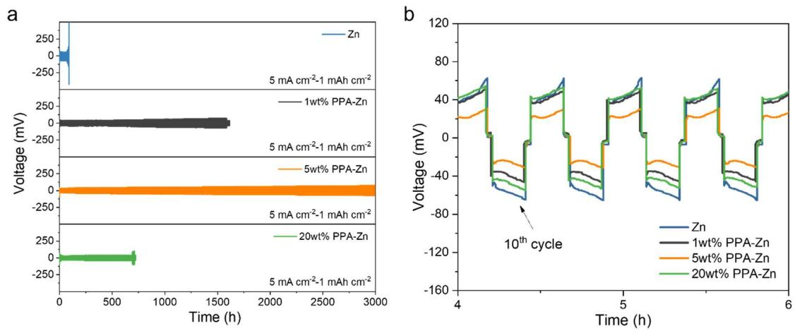
**Figure S2.** (a) Cycle stability and (b) voltage profiles of symmetric cells assembled using Zn foils with Zn phosphate protective layers in different thicknesses: bare Zn, 1wt% PPA-Zn, 5wt% PPA-Zn, and 20wt% PPA-Zn.
