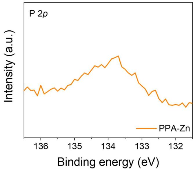
**Figure S8.** XPS spectrum of PPA-Zn after Zn plating at the current density of  $10 \text{ mA cm}^{-2}$  and areal capacity of  $1 \text{ mAh cm}^{-2}$ .
