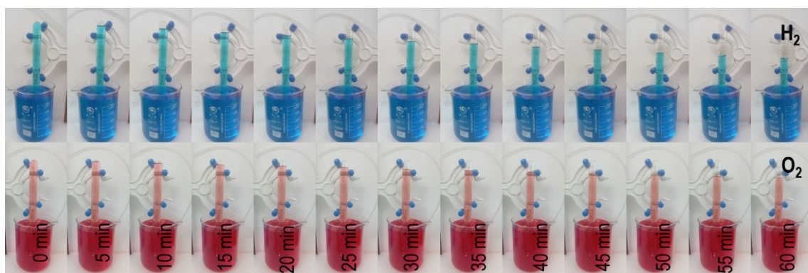
Fig. S24. Enlarged digital images of the measuring gas quantity generated in 60 min in the two-electrode electrolyzer derived by two zinc-air batteries connected in series.
