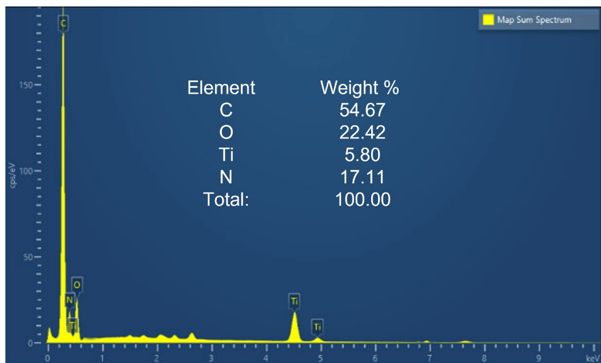
Fig. S14. EDX spectrum from HRTEM image of MX-5@PCNF (inset: weight percentage of different elements).
