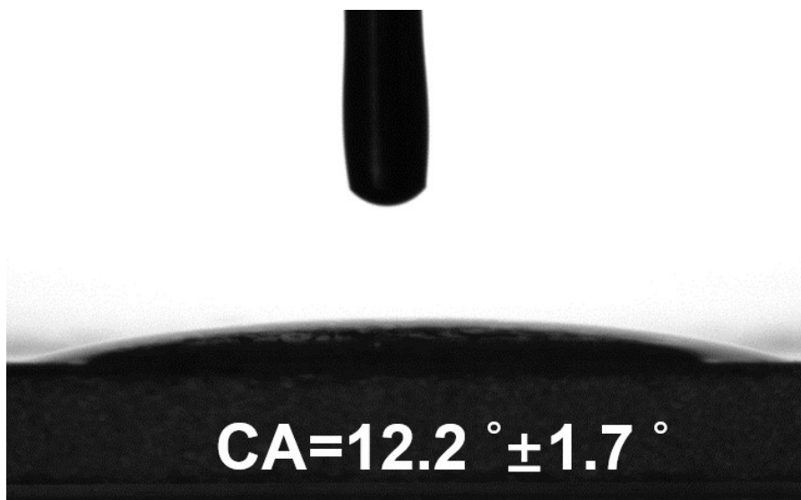
Figure S3. The contact angle of the PVDF membrane with a thickness of 16.9 \mu\text{m} after adding a drop of the \text{LiClO}_4\text{-PC} electrolyte.
