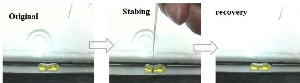
**Fig. S27** Images of **SPH** punctured by using a sharp needle and then rapid recovery without piercing.
