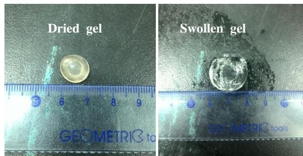
**Fig. S25** Photographs of the swelling experiment of gel before and after being soaked for two hour in water. Left: the dried gel; right: the water-swollen gel.
