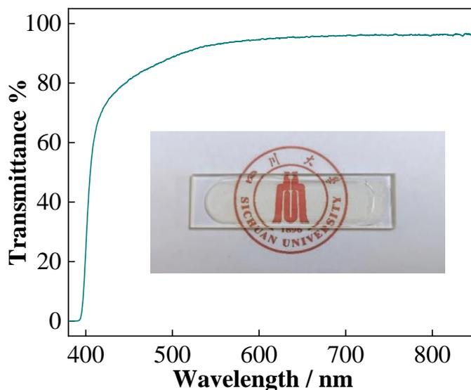
**Fig. S26** Optical transmittance of **SPH** in the wavelength range of 380 to 850 nm; inset: light transmission photographs of **SPH** (water content: 62 wt%; thickness: 1.5 mm)
