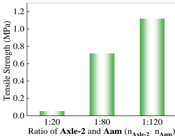
**Fig. S28** Tensile strength of SPH with different ratios of Axle-2 and Aam.
