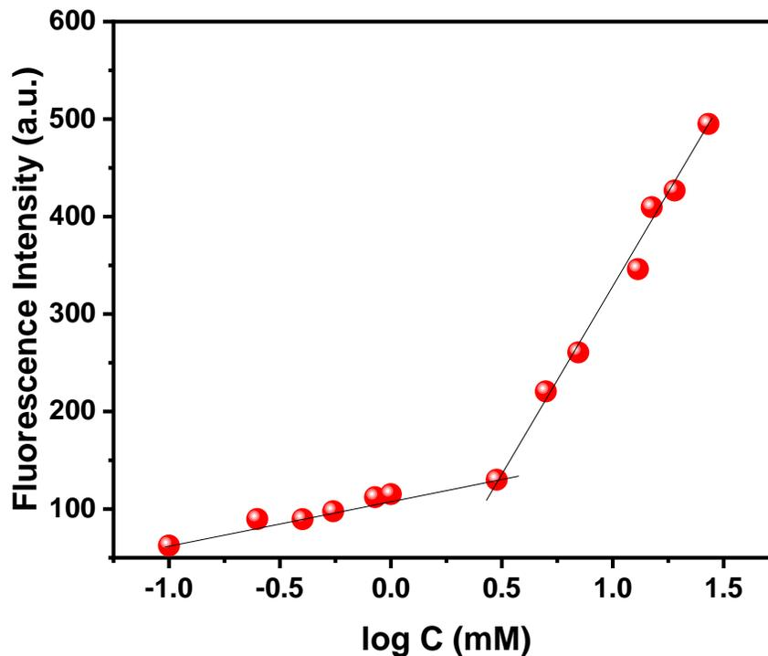
**Fig. S5** Plot showing the fluorescence intensities of DPH versus log (concentration in mM) of the surfactant. The intersection of two lines drawn through the intensities obtained at low and high concentrations of the surfactant gives the CMC of PEG-4-L. The intensities (at the emission wavelength of 430 nm) in the plot were obtained by exciting the sample at 358 nm.
