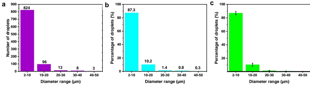
**Fig. S7** Histograms showing the (a) total number and (b) the percentage of droplets in each diameter range of 944 PEG-4-L-decorated LC droplets from 3 representative polarized optical micrographs. (c) The average and standard deviation of the percentage of droplet population in each diameter range was calculated from 3 representative optical micrographs. The concentration of PEG-4-L was 0.5 mM.
