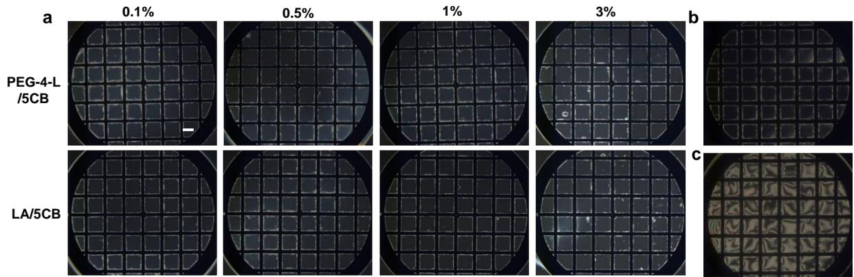
**Fig. S3** (a) Polarized optical micrographs of PEG-4-L/5CB and LA/5CB doped films at LC/air interfaces. At all the concentrations (0.1, 0.5, 1, 3%) investigated, the LC film shows a homeotropic anchoring as observed with (b) pure 5CB at LC/air interface. (c) Planar/tilted alignment of LC observed with pure 5CB at the aqueous interface. The scale bar is 200  $\mu\text{m}$ .
