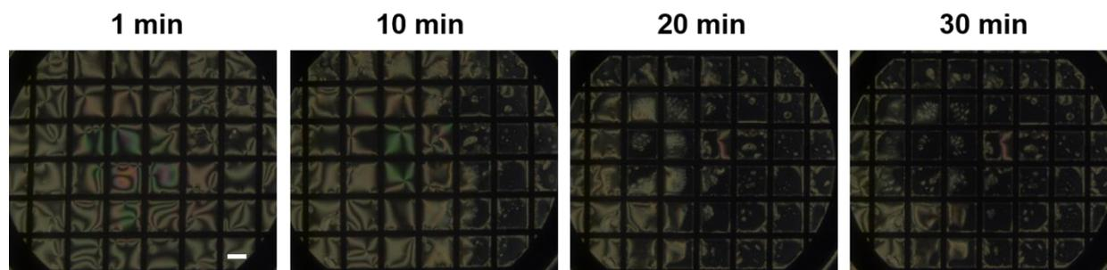
**Fig. S6** Dynamic ordering transition of LC upon addition of a pre-incubated mixture of 0.5 mM PEG-4-L and 1  $\mu$ M deactivated lipase. The lipase was deactivated by heating at 80  $^{\circ}$ C for 4 h. The incubation time was 2 h. The scale bar is 200  $\mu$ m.
