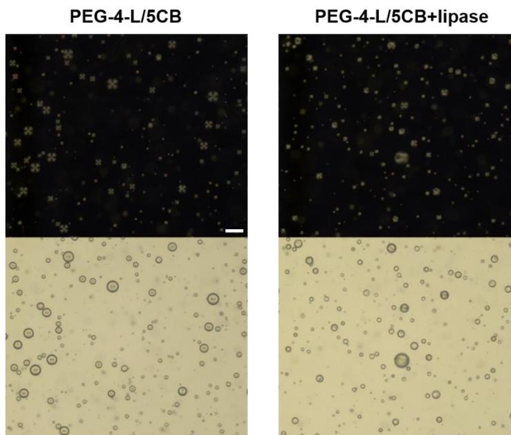
**Fig. S10** Polarized light and bright-field micrographs of 1% PEG-4-L/5CB droplets before and after the addition of 1  $\mu\text{M}$  lipase. The radial configuration of droplets in presence of 1% PEG-4-L/5CB changed to intermediate configurations upon the addition of lipase. The upper and lower panels show polarized light and bright-field micrographs, respectively. The scale bar is 50  $\mu\text{m}$ .
