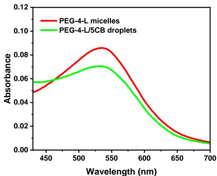
**Fig. S12** Absorption spectra of PEG-4-L micelles and PEG-4-L-decorated 5CB droplets. The concentration of PEG-4-L was 5 mM. The appearance of a peak with  $\lambda_{\text{max}} = 536$  nm indicates that the dye is present in a hydrophobic environment.
