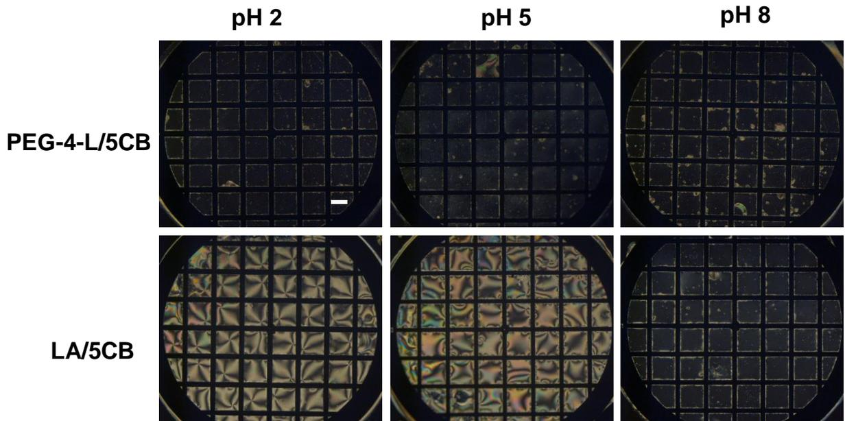
**Fig. S4** Polarized optical micrographs of LC films doped with 0.5% PEG-4-L and LA in 5CB in contact with aqueous PBS at pH 2, 5, and 8. The homeotropic orientation of LC was retained at all pH in the case of 0.5% PEG-4-L/5CB. The scale bar is 200  $\mu\text{m}$ .
