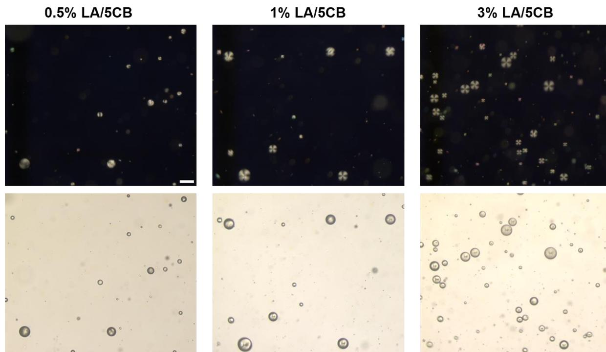
**Fig. S9** Polarized light and bright-field micrographs of 0.5, 1, and 3% LA/5CB droplets in aqueous PBS (pH 7.4). The upper and lower panels show polarized light and bright-field micrographs, respectively. The scale bar is 50  $\mu\text{m}$ .
