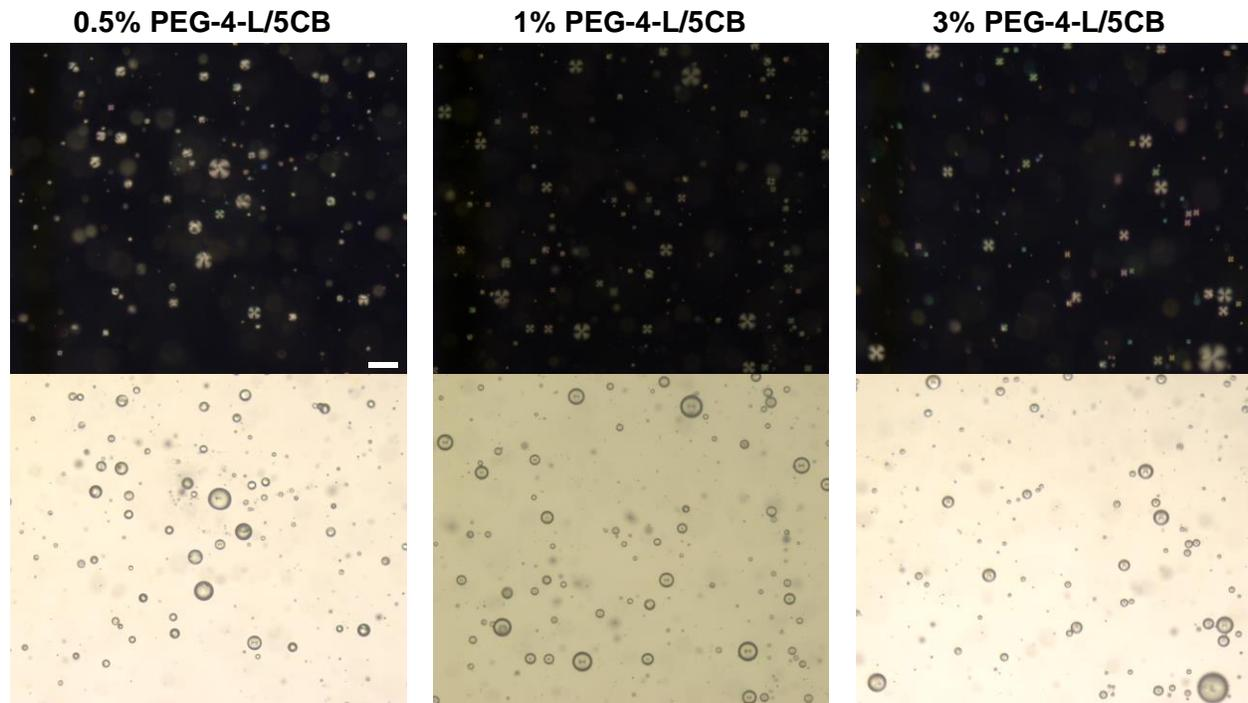
**Fig. S8** Polarized light and bright-field micrographs of 0.5, 1, and 3% PEG-4-L/5CB droplets in aqueous PBS (pH 7.4). The upper and lower panels show polarized light and bright-field micrographs, respectively. The scale bar is 50  $\mu\text{m}$ .
