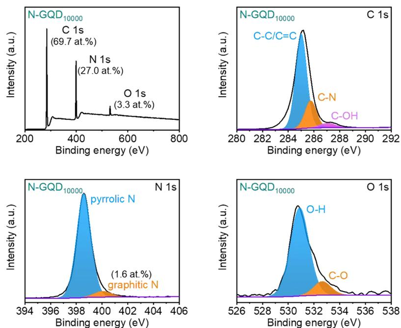
**Fig. S9** Survey XPS spectrum, High-resolution C 1s, N 1s, and O 1s spectra of N-GQD<sub>10000</sub>.
