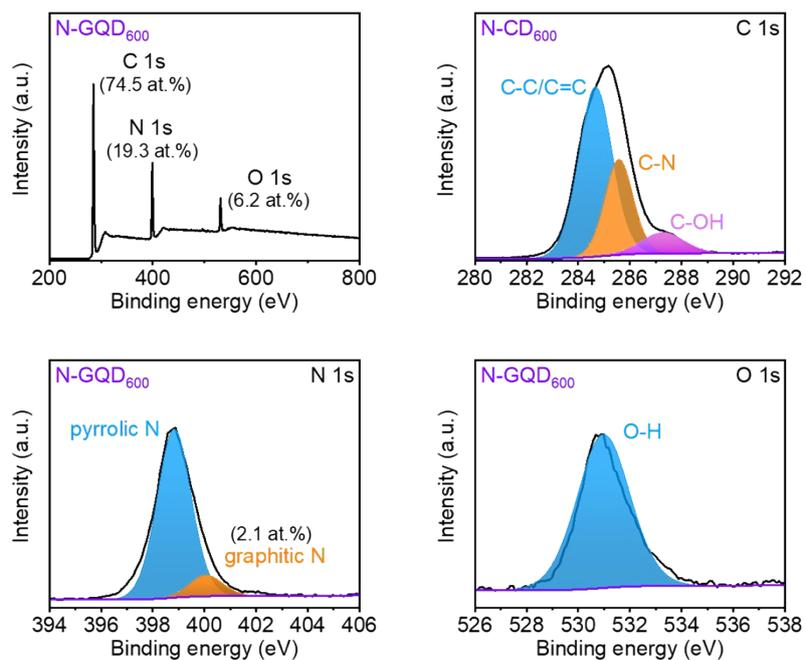
**Fig. S8** Survey XPS spectrum, High-resolution C 1s, N 1s, and O 1s spectra of N-GQD<sub>600</sub>.
