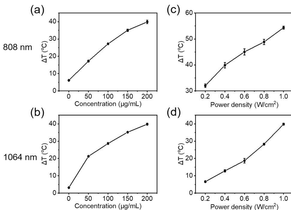
**Fig. S6** (a, b) Plot of temperature change ( $\Delta T$ ) over a period of 300 s versus different concentrations of N-GQDs under irradiation with an 808 (a) and 1064 nm (b) laser irradiation at the power density of 0.4 and 1.0  $\text{W/cm}^2$ , respectively. (c, d) Plot of temperature change ( $\Delta T$ ) over a period of 300 s versus 808 (c) or 1064 nm (d) laser power density.
