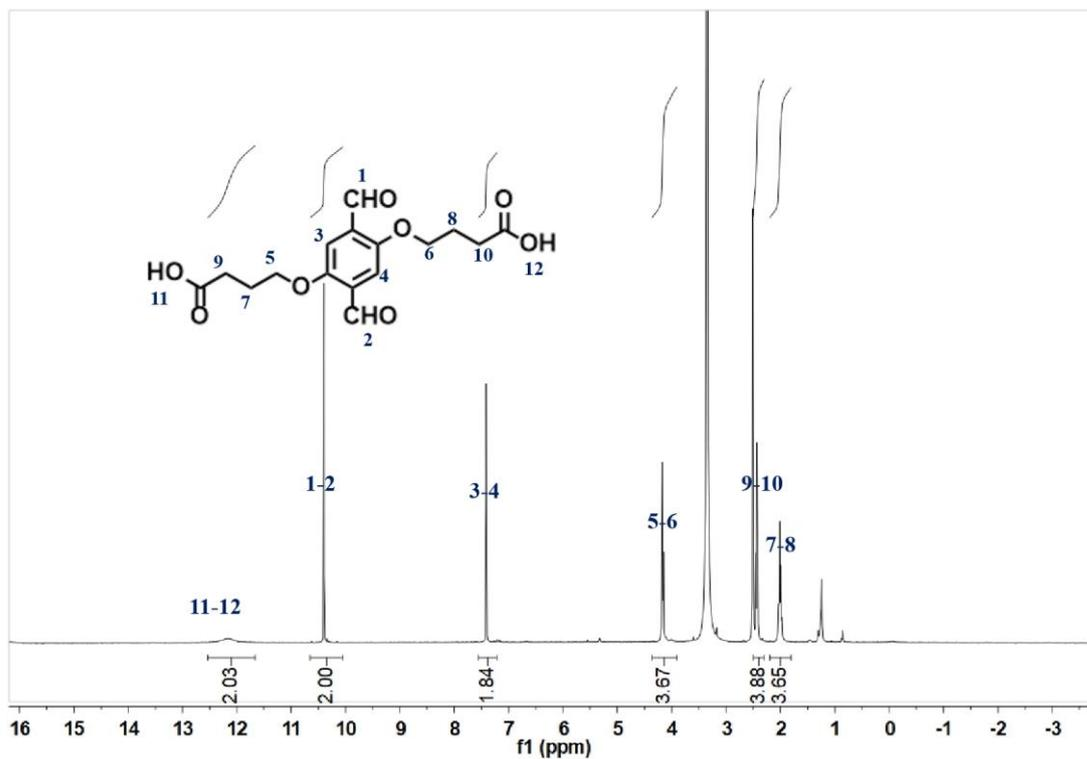
Fig. S3.  $^1\text{H}$  NMR spectrum of 4,4'-((2,5-diformyl-1,4-phenylene)bis(oxy))dibutyric acid (FPBA) in DMSO- $d_6$ .
