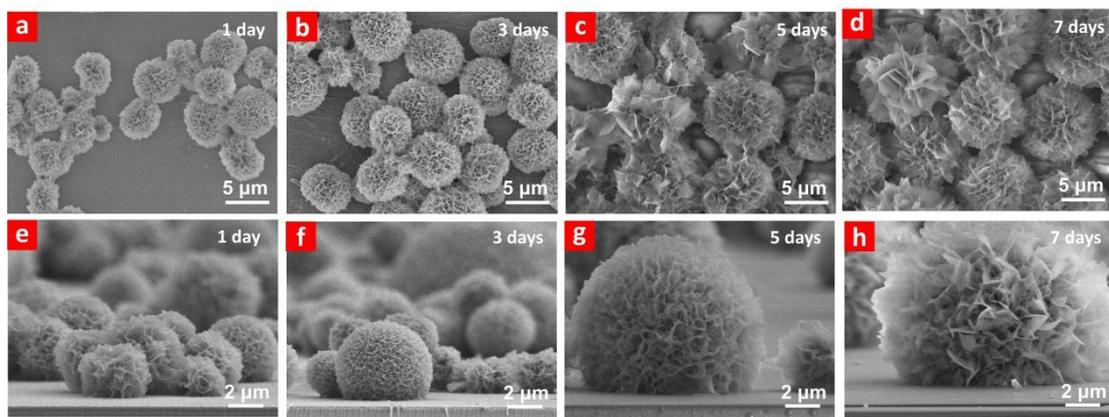
Fig. S10. SEM images show the surface morphology and cross section of 2DP-25% surface after (a)(e)1 day, (b)(f) 3 days, (c)(g) 5 days, and (d)(h) 7 days of biomineralization.
