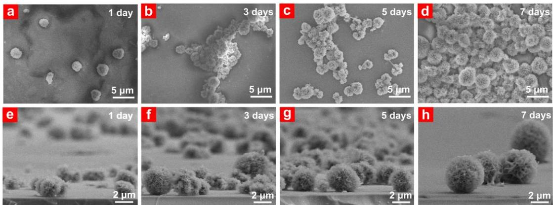
Fig. S11. SEM images show the surface morphology and cross section of 2DP<sub>TAPB+OTPA</sub> surface after (a)(e)1 day, (b)(f) 3 days, (c)(g) 5 days, and (d)(h) 7 days of biomineralization.
