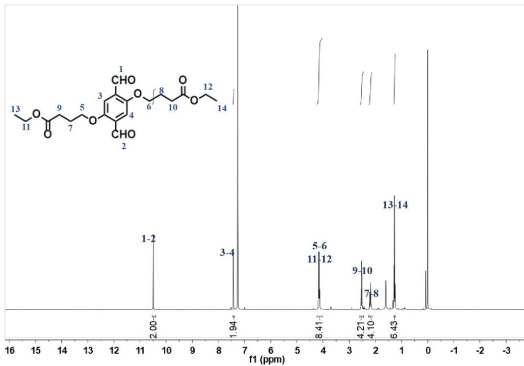
Fig. S1. <sup>1</sup>H NMR spectrum of diethyl-4,4'-((2,5-diformyl-1,4-phenylene)bis(oxy))dibutyrate in CDCl<sub>3</sub>.
