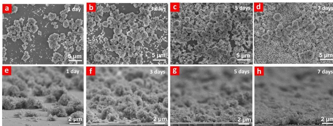
Fig. S8. SEM images show the surface morphology and cross section of 2DP-75% surface after (a)(e) 1 day, (b)(f) 3 days, (c)(g) 5 days, and (d)(h) 7 days of biomineralization.
