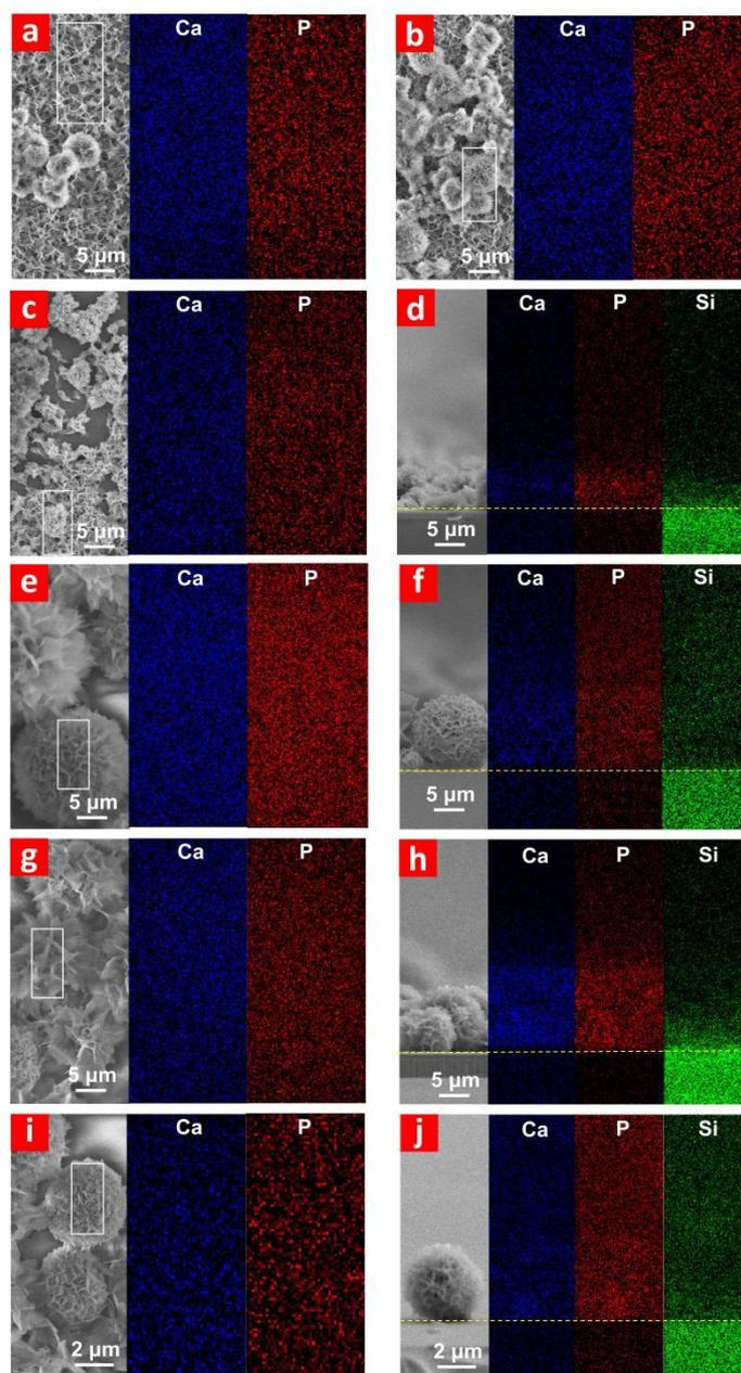
Fig. S14. The element mapping of HAp crystals both on the continuous layer (a) and spheres (b) of 2DP-100%, and both from top view and cross section of (c)(d) 2DP-75%, (e)(f) 2DP-50%, (g)(h) 2DP-25%, (i)(j) 2DP-0% after 5 days of biomineralization
