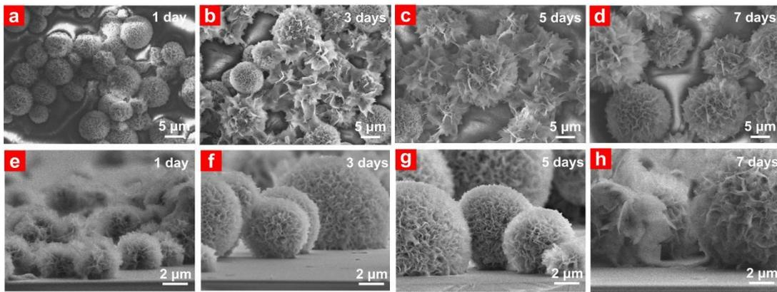
Fig. S9. SEM images show the surface morphology and cross section of 2DP-50% surface after (a)(e)1 day, (b)(f) 3 days, (c)(g) 5 days, and (d)(h) 7 days of biomineralization.
