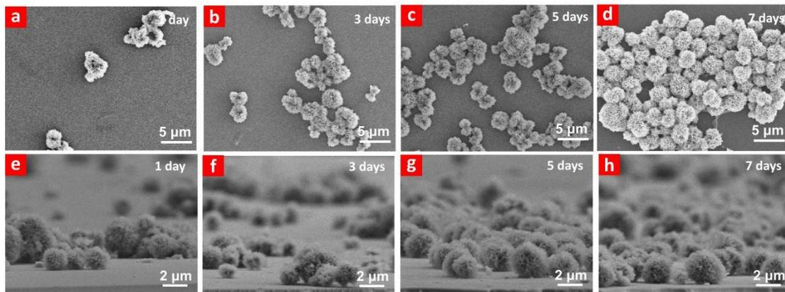
Fig. S12. SEM images show the surface morphology and cross section of glass substrate after (a)(e)1 day, (b)(f) 3 days, (c)(g) 5 days, and (d)(h) 7 days of biom mineralization.
