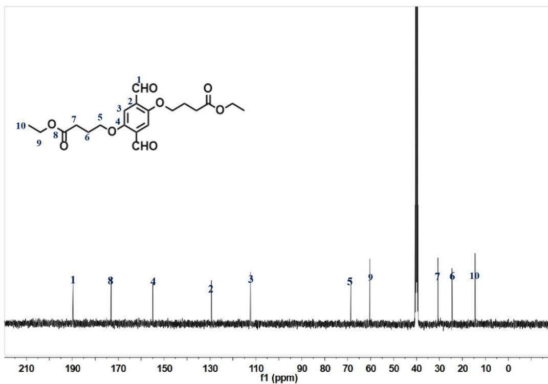
Fig. S2. <sup>13</sup>C NMR spectrum of diethyl-4,4'-((2,5-diformyl-1,4-phenylene)bis(oxy))dibutyrate in CDCl<sub>3</sub>.
