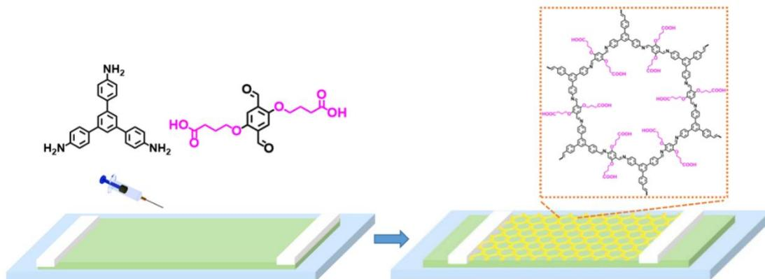
Fig. S5. A schematic illustration on the synthesis of  $2DP_{TAPB+FPBA}$ .
