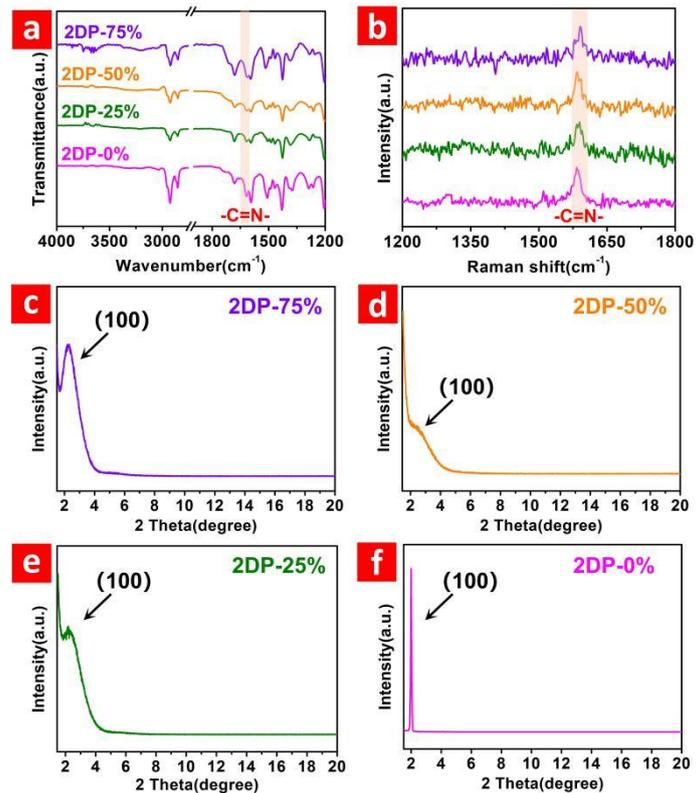
Fig. S7. (a) FT-IR spectra, (b) Raman spectra of 2DPs with different carboxyl density and XRD patterns of the (c) 2DP-75%, (d) 2DP-50%, (e) 2DP-25% and (f) 2DP-0%. (Purple: 2DP-75%, Orange: 2DP-50%, Green: 2DP-25%, Pink: 2DP-0%)
