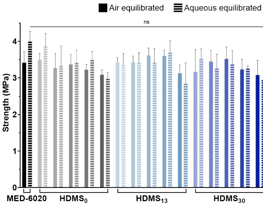
**Figure S14.** Strength of unmodified silicone (MED-6020) and silicones modified with SMAs after air and aqueous equilibration. Statistical analysis ( $p < 0.05$ ); “ns”: not significant.
