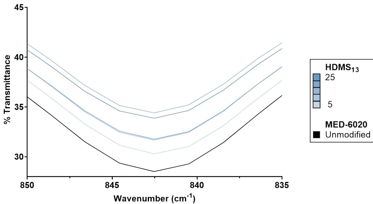
**Figure S9.** ATR-FTIR spectra of unmodified silicone (MED-6020) and silicones modified with HDMS<sub>13</sub> at all concentrations. Color gradient (top of legend) refers to concentration HDMS<sub>13</sub> ( $\mu\text{mol/g}$ ) added to silicone. Characteristic Si-CH<sub>3</sub> stretching peak at 842 cm<sup>-1</sup> decreased with increasing concentration of HDMS<sub>13</sub>.
