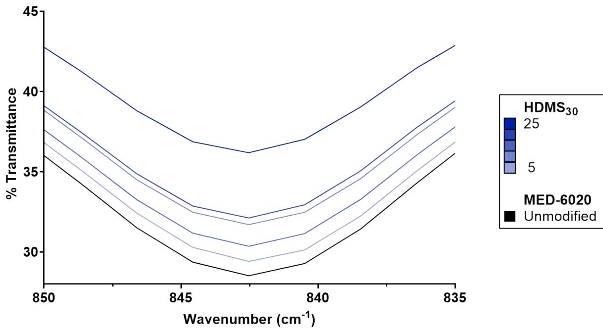
**Figure S12.** ATR-FTIR spectra of unmodified silicone (MED-6020) and silicones modified with HDMS<sub>30</sub> at all concentrations. Color gradient (top of legend) refers to concentration HDMS<sub>30</sub> ( $\mu\text{mol/g}$ ) added to silicone. Characteristic Si-CH<sub>3</sub> stretching peak at 842 cm<sup>-1</sup> decreased with increasing concentration of HDMS<sub>30</sub>.
