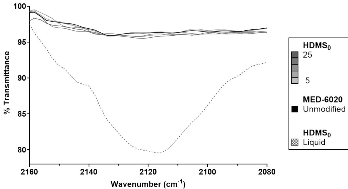
**Figure S5.** ATR-FTIR spectra of unmodified silicone (MED-6020) and silicones modified with HDMS<sub>0</sub> at all concentrations. Color gradient (top of legend) refers to concentration of HDMS<sub>0</sub> ( $\mu\text{mol/g}$ ) added to silicone. The modified silicone spectra lacked the characteristic Si-H peak at 2280-2080 cm<sup>-1</sup>, indicating complete hydrosilylation.
