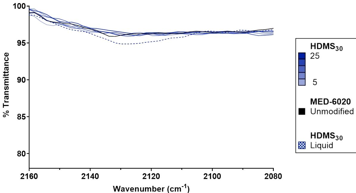
**Figure S11.** ATR-FTIR spectra of unmodified silicone (MED-6020) and silicones modified with HDMS<sub>30</sub> at all concentrations. Color gradient (top of legend) refers to concentration of HDMS<sub>30</sub> ( $\mu\text{mol/g}$ ) added to silicone. The modified silicone spectra lacked the characteristic Si-H peak at 2280–2080  $\text{cm}^{-1}$ , indicating complete hydrosilylation.
