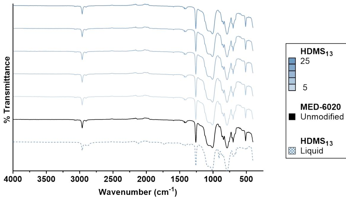
**Figure S7.** ATR-FTIR spectra of unmodified silicone (MED-6020) and silicones modified with HDMS<sub>13</sub> at all concentrations. Color gradient (top of legend) refers to concentration of HDMS<sub>13</sub> ( $\mu\text{mol/g}$ ) added to silicone.
