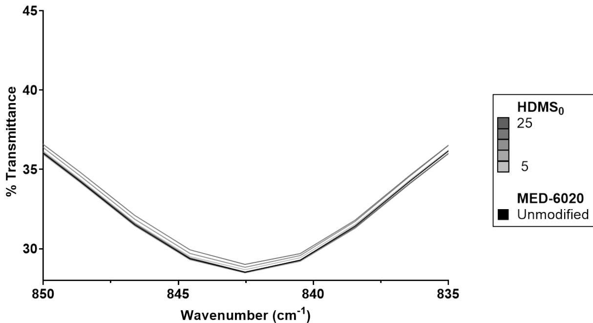
**Figure S6.** ATR-FTIR spectra of unmodified silicone (MED-6020) and silicones modified with HDMS<sub>0</sub> at all concentrations. Color gradient (top of legend) refers to concentration HDMS<sub>0</sub> ( $\mu\text{mol/g}$ ) added to silicone. Characteristic Si-CH<sub>3</sub> stretching peak at  $842 \text{ cm}^{-1}$  decreased with increasing concentration of HDMS<sub>0</sub>.
