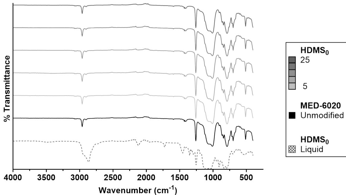
**Figure S4.** ATR-FTIR spectra of unmodified silicone (MED-6020) and silicones modified with HDMS<sub>0</sub> at all concentrations. Color gradient (top of legend) refers to concentration of HDMS<sub>0</sub> ( $\mu\text{mol/g}$ ) added to silicone.
