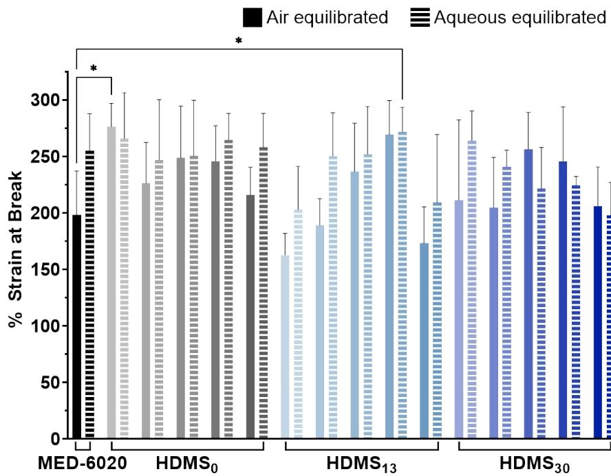
**Figure S15.** % Strain at break of unmodified silicone (MED-6020) and silicones modified with SMAs after air and aqueous equilibration. \* $p < 0.05$ : MED-6020 v. HDMS<sub>0</sub> @ 5  $\mu\text{mol/g}$  after air equilibration; MED-6020 v. HDMS<sub>13</sub> @ 20  $\mu\text{mol/g}$  after aqueous equilibration.
