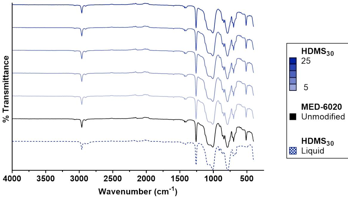
**Figure S10.** ATR-FTIR spectra of unmodified silicone (MED-6020) and silicones modified with HDMS<sub>30</sub> at all concentrations. Color gradient (top of legend) refers to concentration of HDMS<sub>30</sub> ( $\mu\text{mol/g}$ ) added to silicone.
