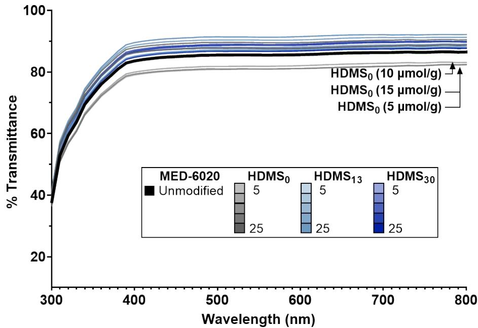
**Figure S13.** % Transmittance of unmodified silicone (MED-6020) and silicones modified with SMAs after air equilibration. Color gradients refer to concentration of HDMS<sub>0</sub>, HDMS<sub>13</sub>, or HDMS<sub>30</sub> ( $\mu\text{mol/g}$ ) added to silicone. All formulations except for those modified with HDMS<sub>0</sub> exhibited greater % transmittance versus MED-6020.
