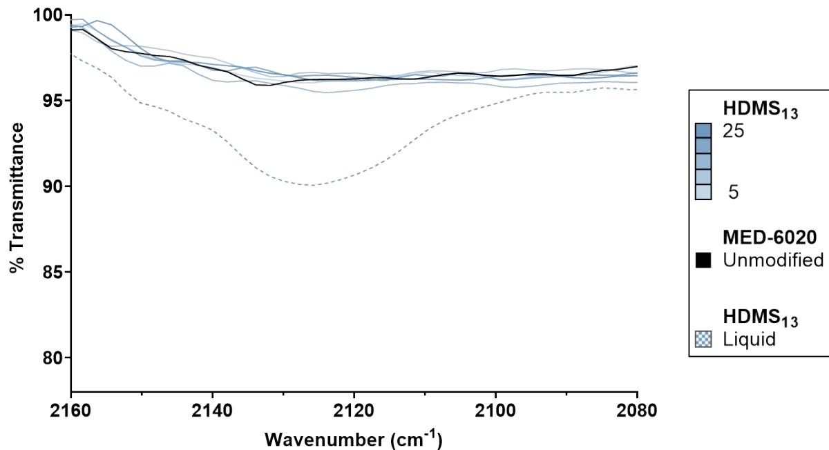
**Figure S8.** ATR-FTIR spectra of unmodified silicone (MED-6020) and silicones modified with HDMS<sub>13</sub> at all concentrations. Color gradient (top of legend) refers to concentration ( $\mu\text{mol/g}$ ) added to silicone. The modified silicone spectra lacked the characteristic Si-H peak at 2280-2080  $\text{cm}^{-1}$ , indicating complete hydrosilylation.
