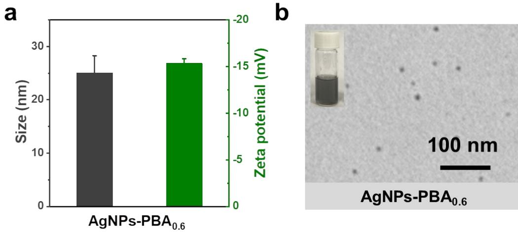
**Fig. S1** (a) The size and Zeta potential of AgNPs-PBA<sub>0.6</sub>. (b) Representative TEM image and the pictures of AgNPs-PBA<sub>0.6</sub>.
