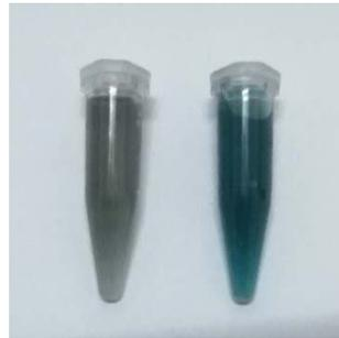
Figure S7. Digital photos of TMB before and after adding CaO<sub>2</sub>@SiO<sub>2</sub> NPs in the presence of Fe<sup>2+</sup>.
