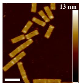
Figure S 9: AFM images of uncoated DNA origami ( $O_8$ ) containing StA and StE sequences.
