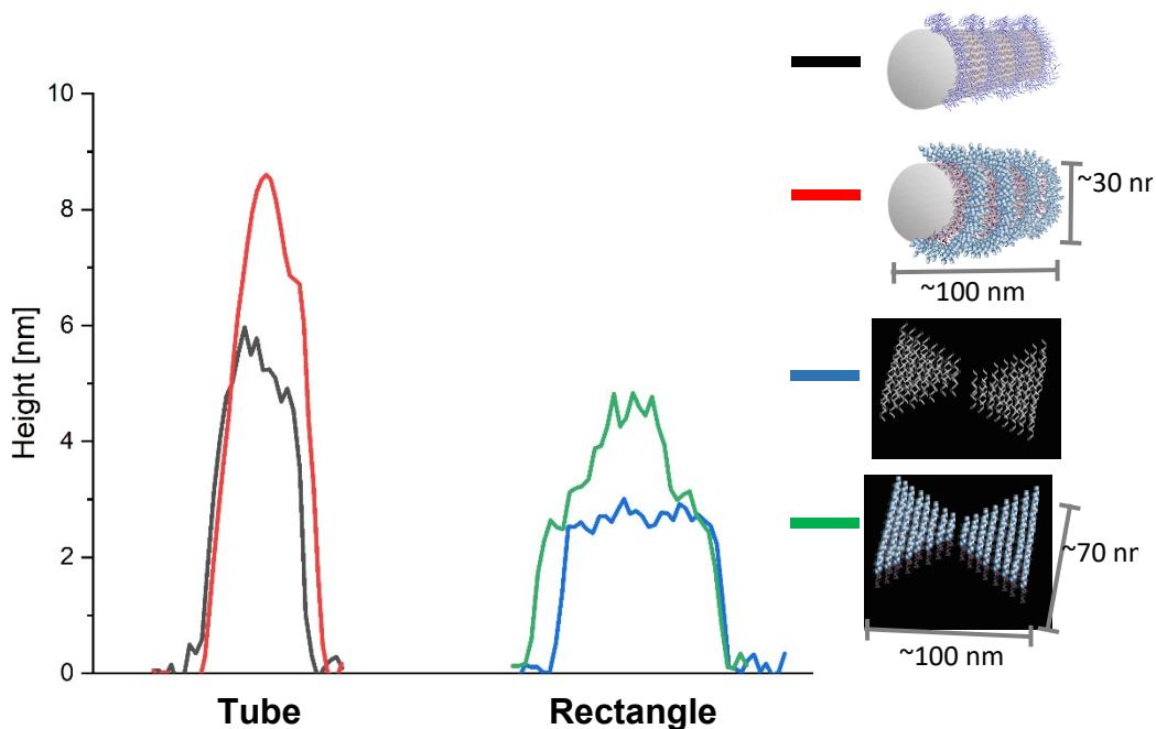
Figure S 10: AFM topographic images of O<sub>4</sub>, O<sub>5</sub>, O<sub>6</sub> and O<sub>7</sub> (Figure 3 f,g,h,i) reveal a significant increase in height of the respective coating area.
