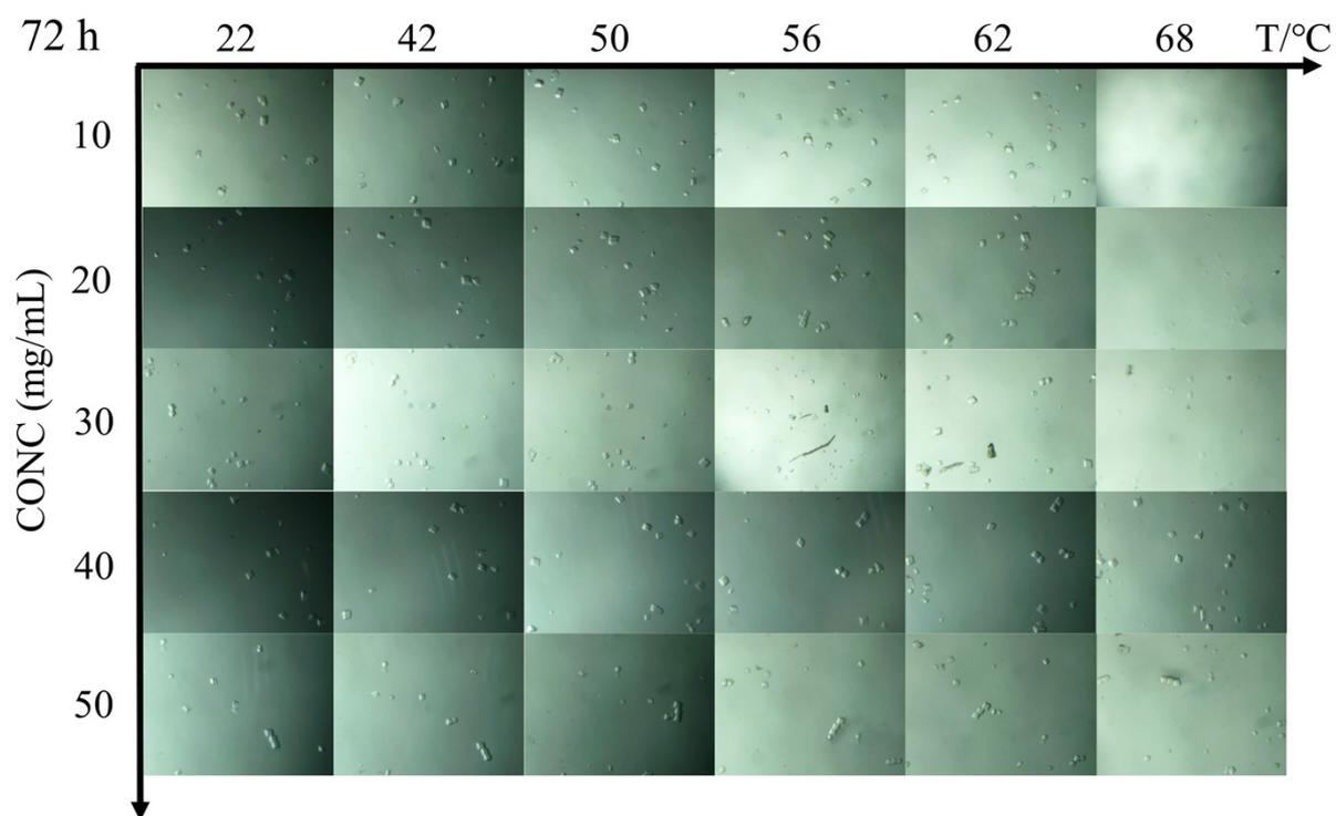
After EDC chemical ligation for 72 hours, the effect of different EDC concentration on thermal stability of SC-5P.
