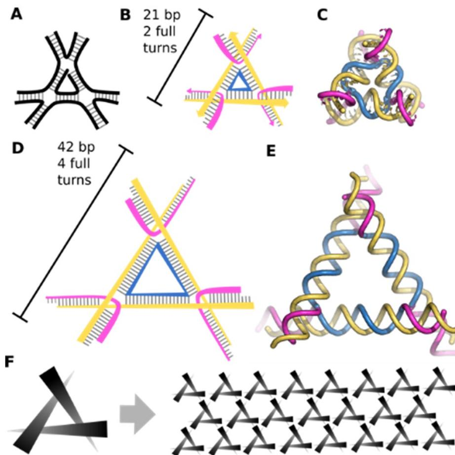
**Figure S3.** Original 3-fold symmetric tensegrity triangle tile (A) 2D cartoon, (B) 3D cartoon illustrating three distinct strand sequences (yellow, blue, pink), (C) the 3D crystal structure of the tile from PDB entry 3gbi. In comparison, (D) the new tile is predicted to have 4 turns of dsDNA per beam, (F) Sticky overhangs at the ends of the protruding arms encode asymmetric assembly in 3 dimensions.
