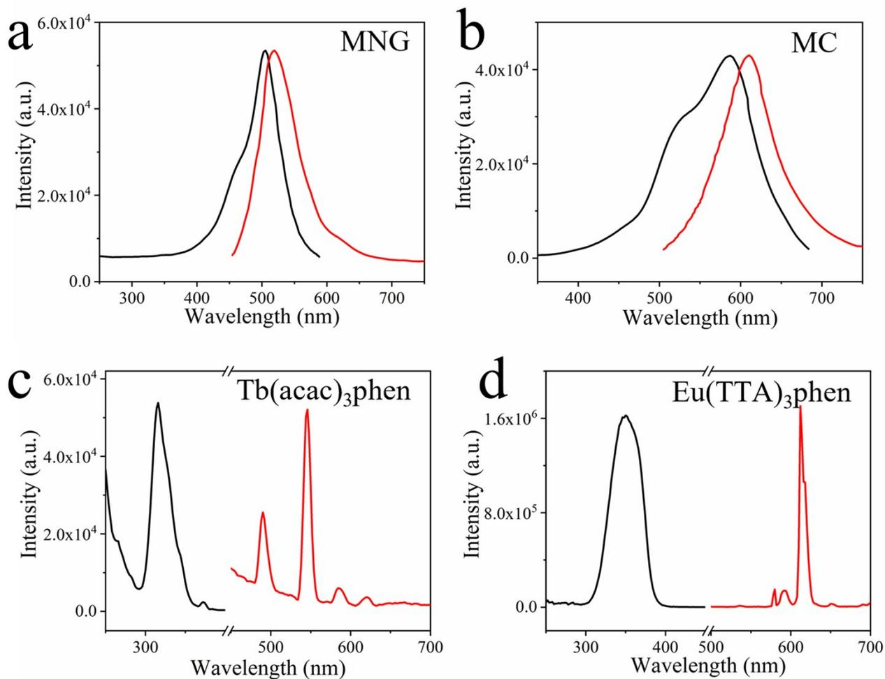
**Figure S8.** Excitation and emission spectra of fluorescent proteins and luminescent rare earth complexes.
