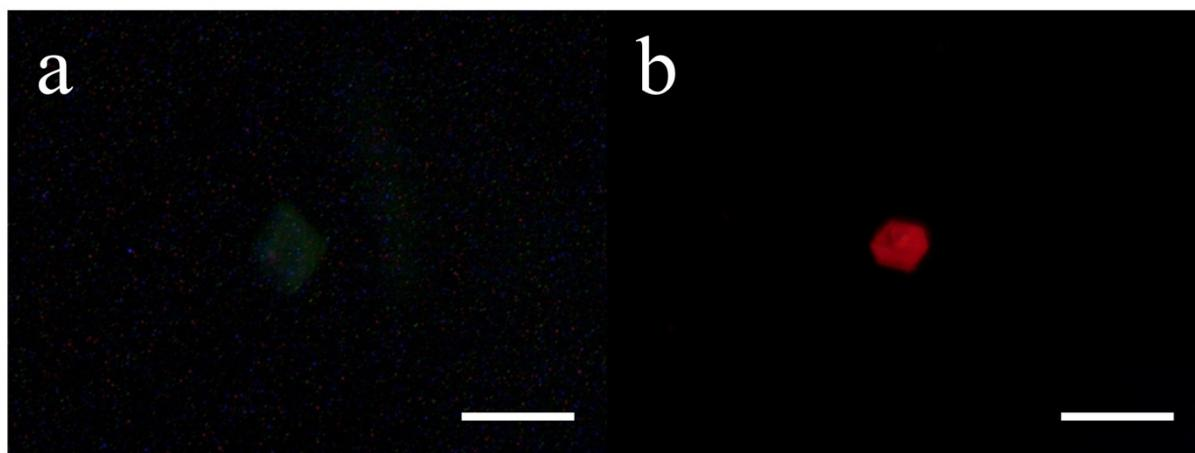
**Figure S14.** Fluorescence microscopy (365 nm excitation light) of rare earth loading of CLSC. **(a)** Incubating a CLSC in  $\text{Tb}(\text{acac})_3\text{phen}$  after 2 min. **(b)** Incubating a CLSC in  $\text{Eu}(\text{TTA})_3\text{phen}$  after 2 min. The scale bar is 100  $\mu\text{m}$ .
