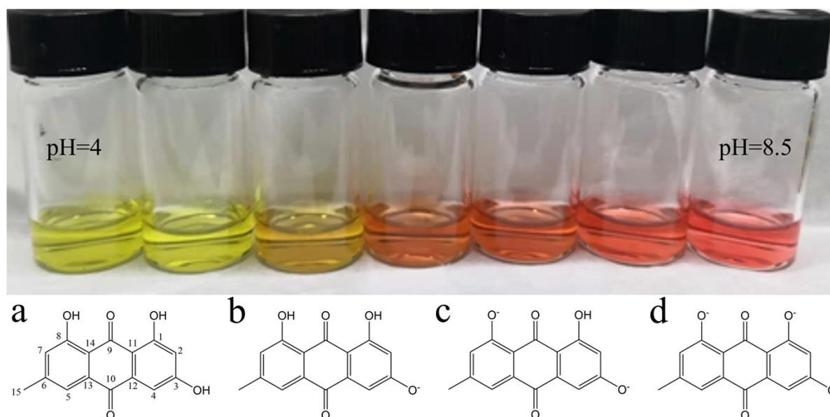
**Figure S11.** Emodin changes color under different pH due to deprotonation process, and the anionic/deprotonated form is red. **(a)** Molecular structure and atomic number of emodin in neutral form, and the stepwise dissociation of three protons: first in position 3 **(b)** 3-oxido-6-methyl-1,8-dihydroxy-9,10-anthraquinone, second in position 8 **(c)** 3,8-oxido-6-methyl-1-hydroxy-9,10-anthraquinone and third in position 1 **(d)** 1,3,8-oxido-6-methyl-9,10-anthraquinone.
