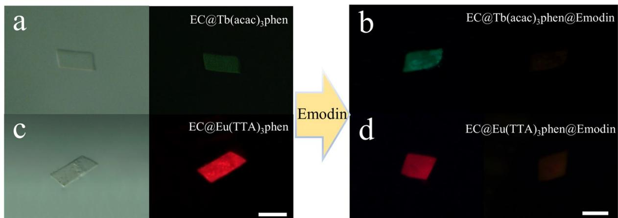
**Figure S12.** Light and fluorescence microscopy (365 nm excitation light) of rare earth loading of CLEC. **(a)** Incubating a CLEC in  $\text{Tb}(\text{acac})_3\text{phen}$  after 2 min. **(c)** Incubating a CLEC in  $\text{Eu}(\text{TTA})_3\text{phen}$  after 2 min. **(b, d)** the crystals after transfer into a 10 mM solution of emodin at 1 min, and 3 min. The scale bar is 100  $\mu\text{m}$ .
