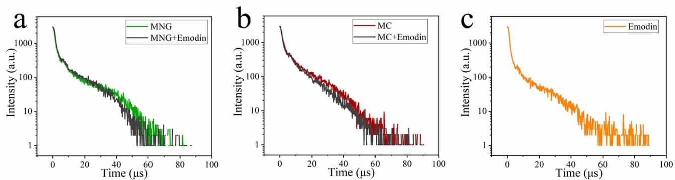
**Figure S13.** The fluorescence lifetime for **(a)** mNeonGreen in water, with and without 1 mM emodin. The excitation wavelength was 506 nm, and **(b)** mCherry in water, with and without 1 mM emodin. The excitation wavelength was 588 nm. **(c)** The fluorescence lifetime for emodin was also measured.
