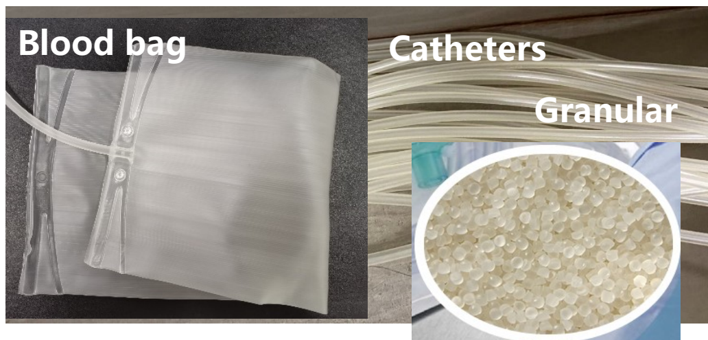
Figure S4. Digital photos for anticoagulation PVC granular and extrusion end products of blood bags and PVC tubing.
