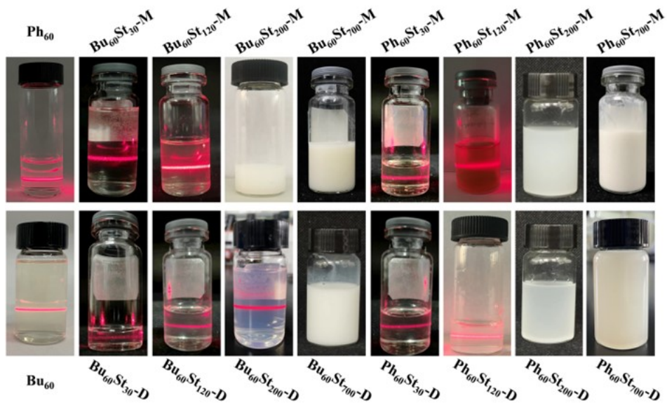
Figure S8. Tyndall effect of Bu_{60}St_y and Ph_{60}St_y PFDCs in either methanol or 1,4-dioxane solvent.
