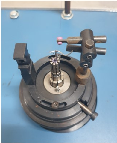
Figure S1. Tubular knit scaffold is manufactured by knitting PGA suture fiber from knitting machine.
