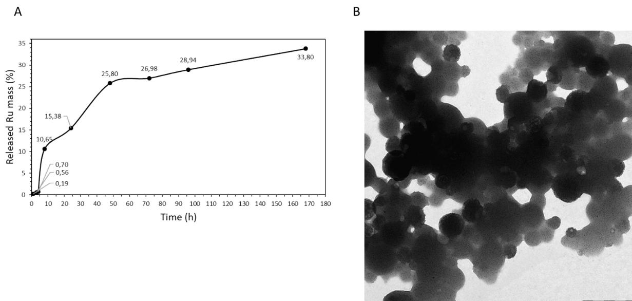
**Figure S4:** Release assay of RuCy from NAS-RuCy and TEM characterization after 7 days. (A) Nanoparticles were incubated in HEPES buffer for 7 days at 37°C. For each time point a buffer aliquot was withdrawn and ruthenium content was analyzed by ICP-MS analysis. Percentage was calculated with respect to the amount of ruthenium placed in the dialysis membrane. (B) TEM characterization of NAS-RuCy after 7 days in HEPES buffer at 37°C.
