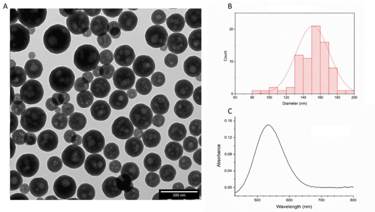
**Figure S2:** Physical-chemical characterization of NAs-CisPt. (A) TEM images of NAs-CisPt. Scale bar: 300 nm. (B) Size histogram of NAs-CisPt made on at least 100 NAs observed by TEM. (C) Background subtracted UV-Vis absorbance spectrum of NAs-CisPt.
