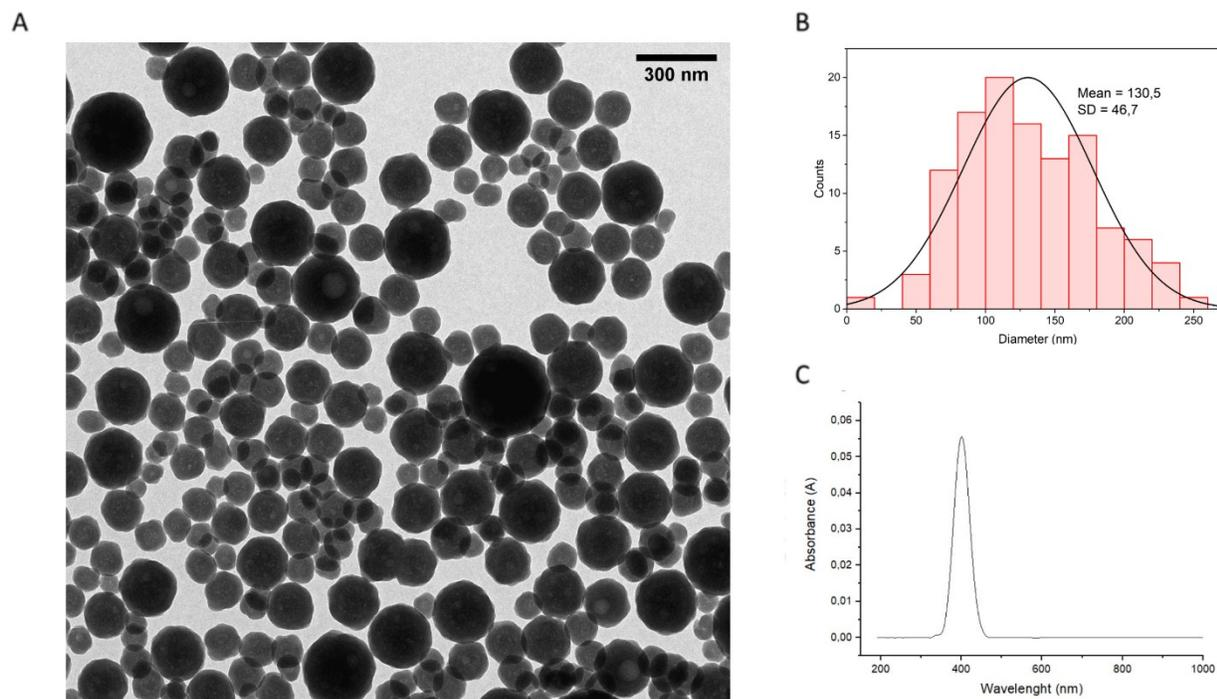
**Figure S3:** Physical-chemical characterization of NAS-RuCy. (A) TEM images of NAS-RuCy. Scale bar: 300 nm. (B) Size histogram of NAS-RuCy made on at least 100 NAs observed by TEM. (C) Background subtracted UV-Vis absorbance spectrum of NAS-RuCy.
