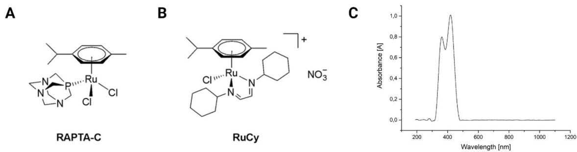
**Figure S1:** Chemical structures of ruthenium compounds (A) RAPTA-C and (B) RuCy. (C) UV-Vis spectrum of RuCy dissolved in milliQ® water.
