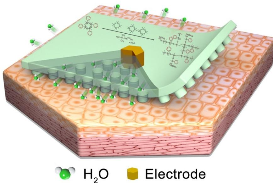
**Figure S12.** Conceptual illustration of the phenyl-rich microfibrillar adhesive used as skin patches showing strong hydrophobic effect.
