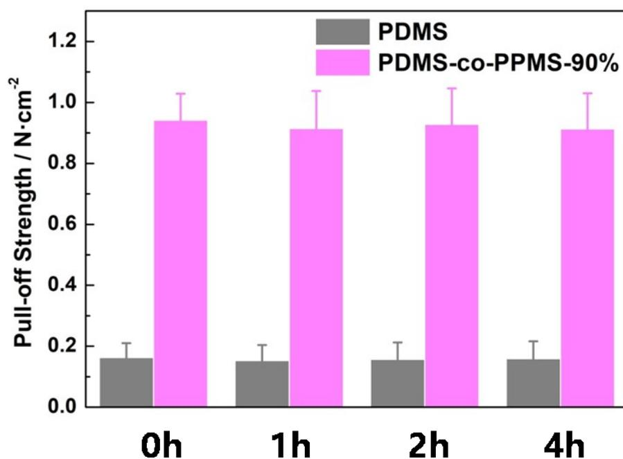
**Figure S8.** The comparison of average pull-off strength of PDMS and PDMS-co-PPMS-90% at 95±3.0% RH under various equilibration time.
