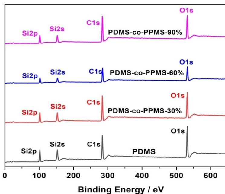
**Figure S3.** XPS spectra of bulk elastomers with various phenyl contents. The binding energy of N1s is around 403 eV, which was not labeled due to the low relative contents.
