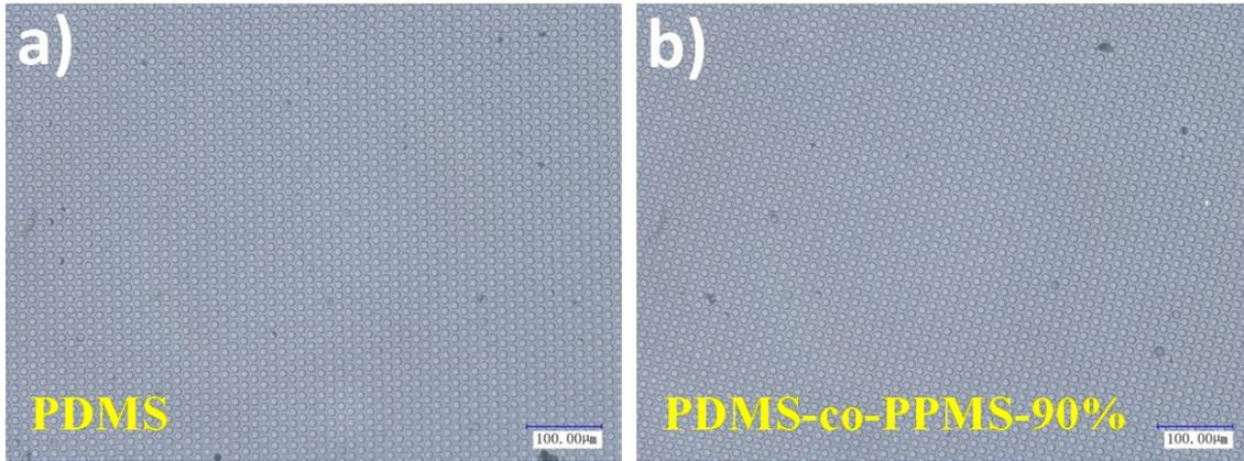
**Figure S9.** Optical microstructures of PDMS (a) and PDMS-co-PPMS-90% (b) microfibrillar adhesives after humidity macroadhesion tests.
