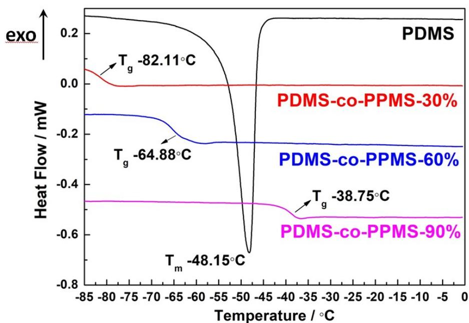
**Figure S4.** DSC curves of polysiloxane elastomers with various phenyl contents.
