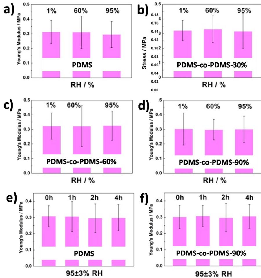
**Figure S5.** Results of humidity tensile tests results. Young's moduli of PDMS (a), PDMS-co-PPMS-30% (b), PDMS-co-PPMS-60% (c), and PDMS-co-PPMS-90% (d) at RH of  $1\pm 0.5\%$ ,  $60\pm 3\%$ , and  $95\pm 3\%$ , respectively, and each humidity set point was equilibrated for 1h. Young's moduli of two specimens, PDMS (e) and PDMS-co-PPMS-90% (f), equilibrated for 1h, 2h, 3h and 4h at  $95\pm 3\%$  RH, respectively.
