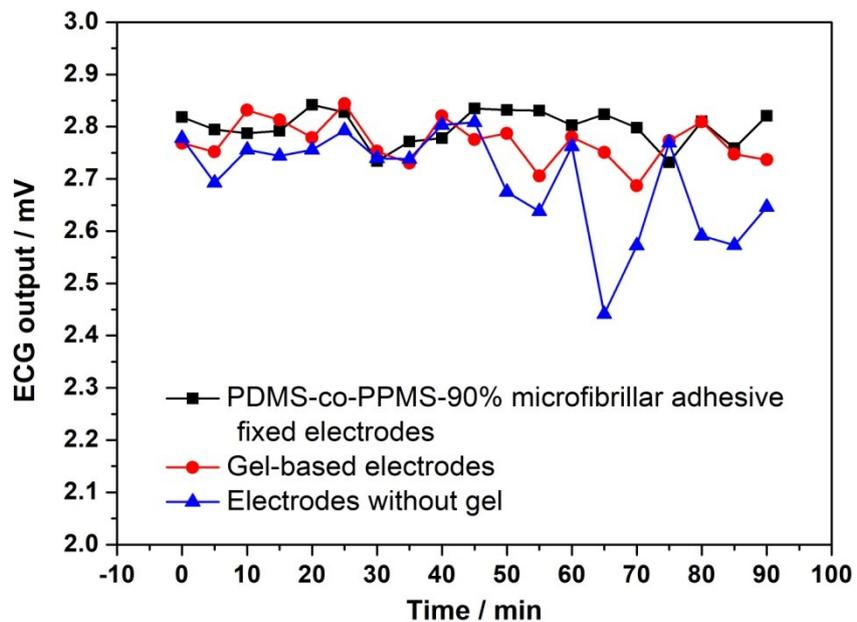
**Figure S11.** The ECG output voltage (R-wave) of three kinds of electrodes as a function of monitoring time.
