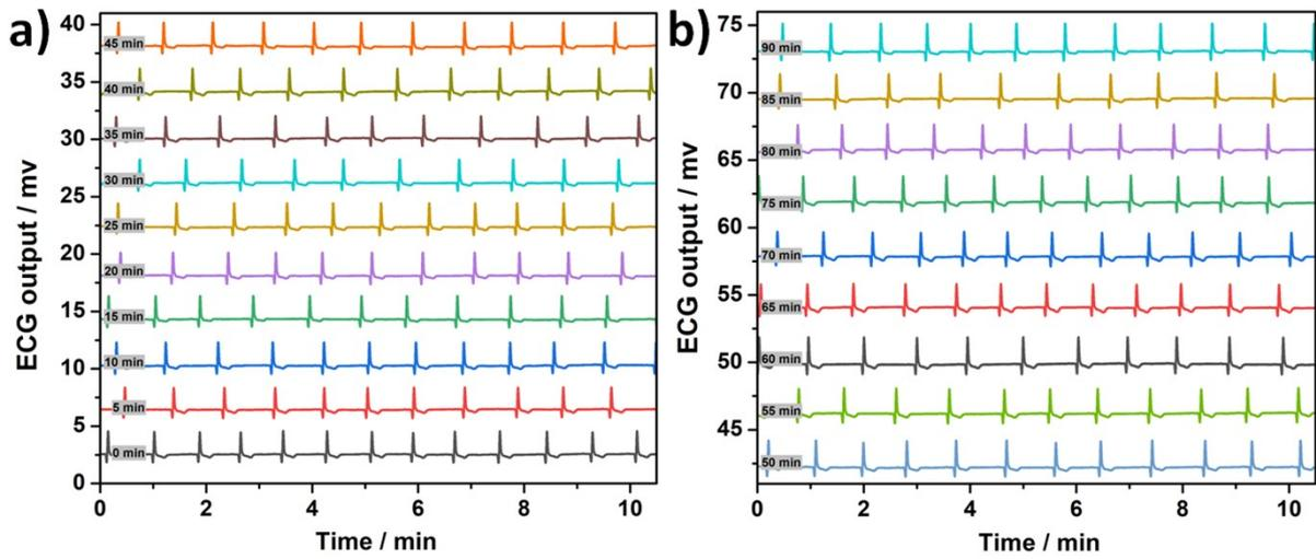
**Figure S10.** ECG data taken on a seated subject based on electrodes without gel. (a) 0-45min; (b) 50-90min.
