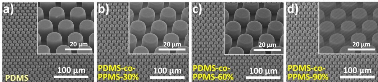
**Figure S7.** Morphologies of microfibrillar adhesives fabricated by PDMS (a), PDMS-co-PPMS-30% (b), PDMS-co-PPMS-60% (c), and PDMS-co-PPMS-90% (d), with pillar diameter of  $10\ \mu\text{m}$ , pillar height of  $10\ \mu\text{m}$  and spacing of  $15\ \mu\text{m}$ , respectively. Insets showed the magnified morphologies of four microfibrillar adhesives.
