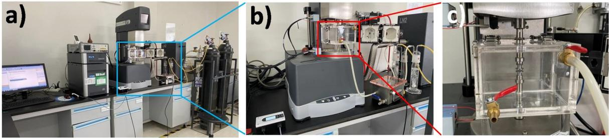
**Figure S6.** The photograph of humidity macroadhesion measurement device. It consists of RSA G2 solid rheometer (a) and humidity regulating setup. By aerating the dry and wet nitrogen with different flow rates through the tailored mixing chamber (b and c), RH levels can be varied from  $1\pm 0.5\%$  to  $95\pm 3\%$ .
