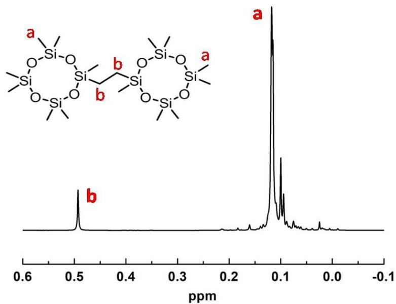
**Figure S1.**  $^1\text{H-NMR}$  of Bis-D4. 600 MHz,  $\text{CDCl}_3$ ,  $\delta = 0.49$  ppm (4H, 2  $-\text{CH}_2-$ ), 0.13-0.08 ppm (42H, 14  $-\text{CH}_3$ ).
