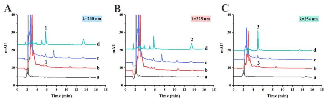
**Fig. S4** Chromatograms of sample 1. (A) Chromatogram at 230 nm; (B) chromatogram at 225 nm; (C) chromatogram at 254 nm; (a) sample 1 direct injection; (b) extracted sample 1 by MIP; (c) MIP extracted spiked 1  $\mu\text{g/L}$  sample 1; and (d) 1 mg/L mixed standard solution: 1. BPF, 2. DEP, and 3. MP.
