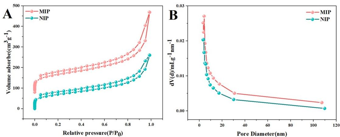
Fig. S2 (A) N<sub>2</sub> adsorption–desorption isotherms, (B) pore size distribution of MIP and NIP.
