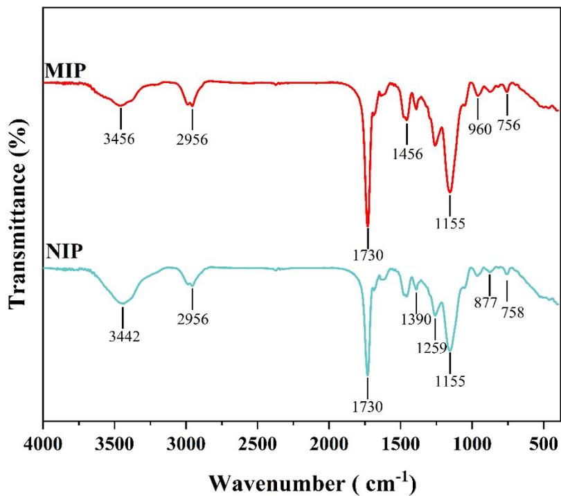
Fig. S1 FT-IR spectra of MIP and NIP fibers.
