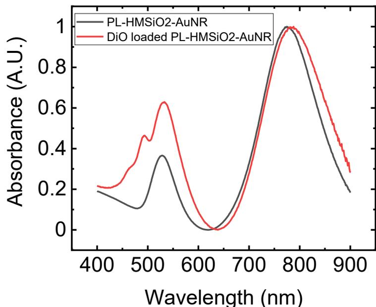
Figure S6. UV-Vis spectra of PL-HMSiO<sub>2</sub>-AuNR with and without loading of DiO.
