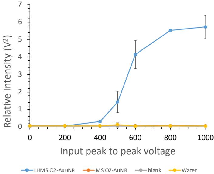
Figure S5. Intensity of received acoustic signal vs. input driving voltage from the PL-HMSiO2-AuNR, MSiO2-AuNR, water, and blank (no sample holder).
