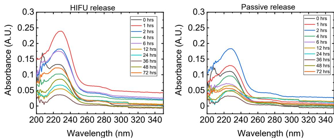
Figure S8. UV-Vis spectra of PTX released from PL-HMSiO<sub>2</sub>-AuNR at various timepoints with either (a) HIFU applied or (b) HIFU not applied.
