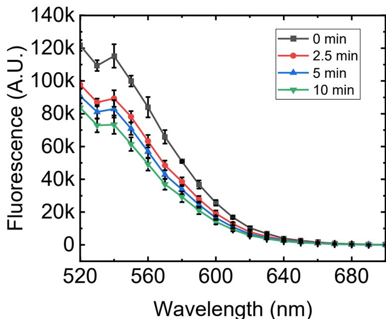
Figure S7. Fluorescence emission spectra of DiO-loaded PL-HMSiO<sub>2</sub>-AuNRs following 0, 2.5, 5, and 10 min HIFU insonation.
