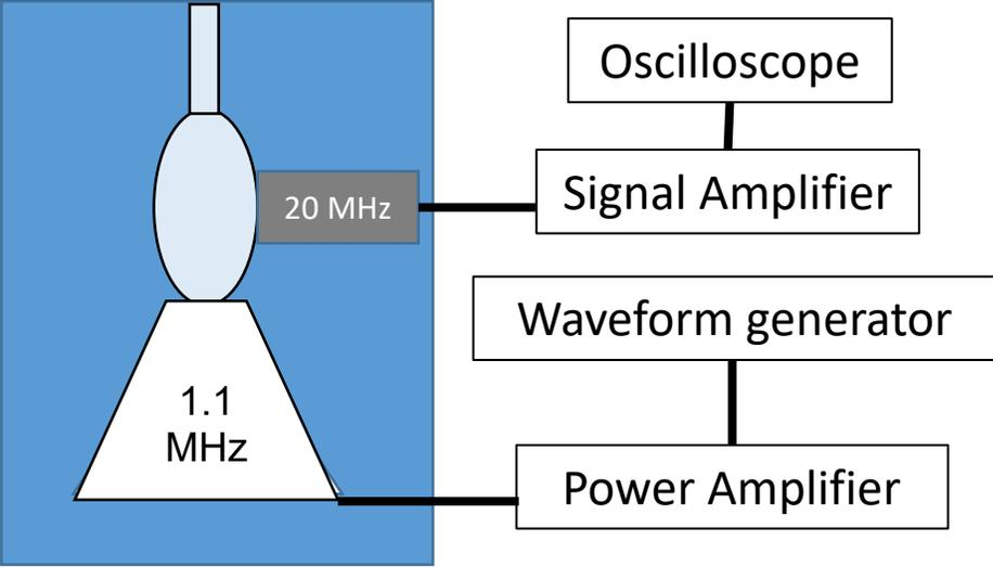
Figure S4. Schematic of HIFU setup for passive cavitation detection.
