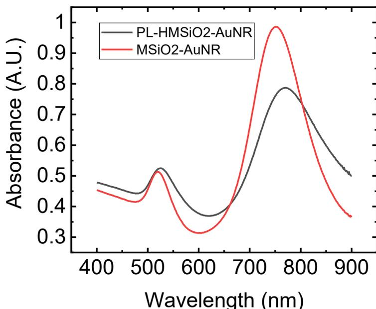
Figure S1. UV-Vis spectra of PL-HMSiO<sub>2</sub>-AuNR and MSiO<sub>2</sub>-AuNR with concentrations adjusted to match absorbance at 800 nm.
