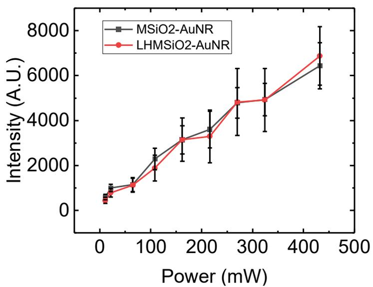
Figure S3. Intensity of two-photon luminescence of PL-HMSiO<sub>2</sub>-AuNR and the MSiO<sub>2</sub>-AuNR at 120 s irradiation at different input laser powers.
