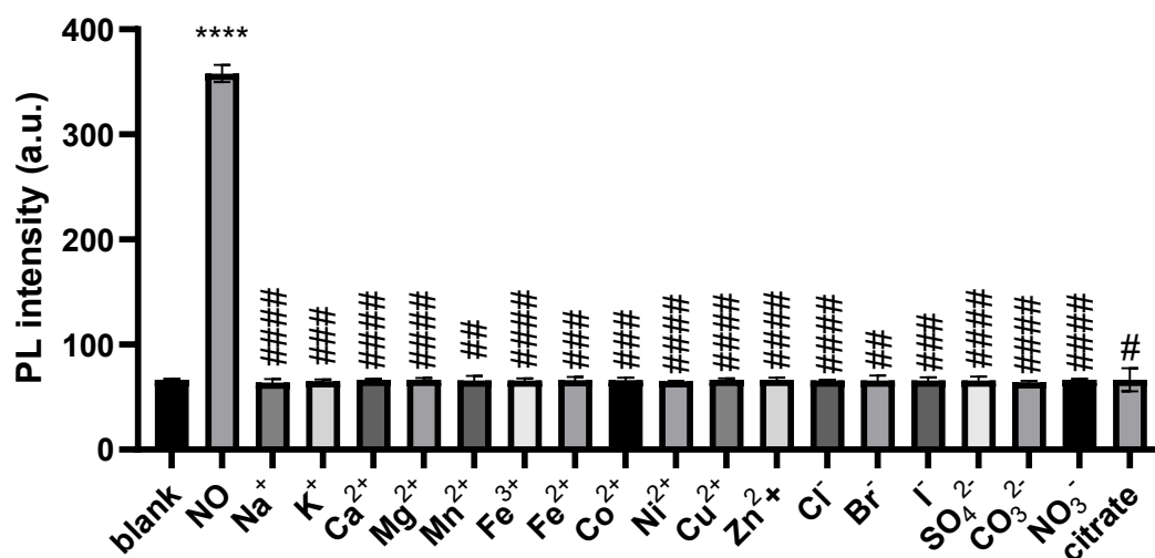
Figure S5. The reaction of 10 \mu M AIE probe to NO and other different ions; **** indicates the difference compared to blank, #, ##, ###, #### indicate the differences compared to NO. #, p < 0.05 ; ##, p < 0.01 ; ###, p < 0.001 ; **** and ####, p < 0.0001 .
