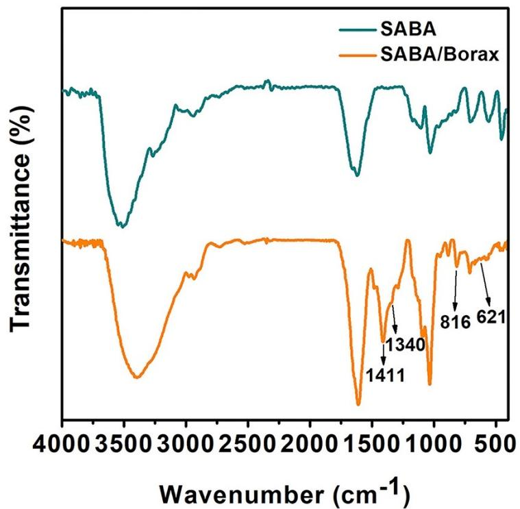
Fig. S3. FTIR spectra of SABA and SABA/Borax hydrogel.
