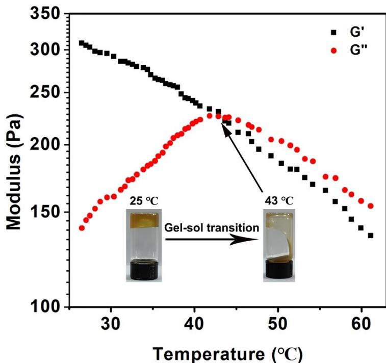
Fig. S6. The temperature-dependent development of  $G'$  and  $G''$  for SABA/Borax hydrogel.
