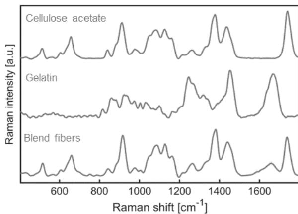
**Fig. S5** Raman spectra of reference substances and blend fibers.
