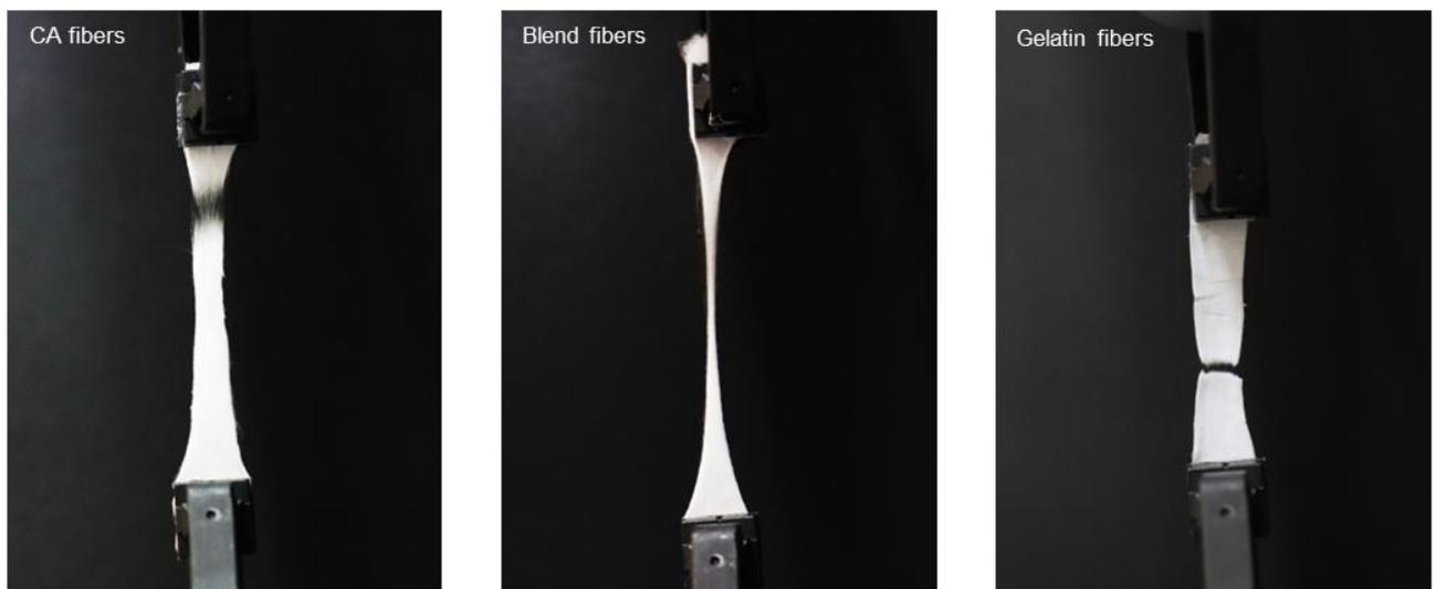
**Fig. S2** Photographs of CA, blend, and gelatin fiber scaffolds after failure during tensile testing experiments.
