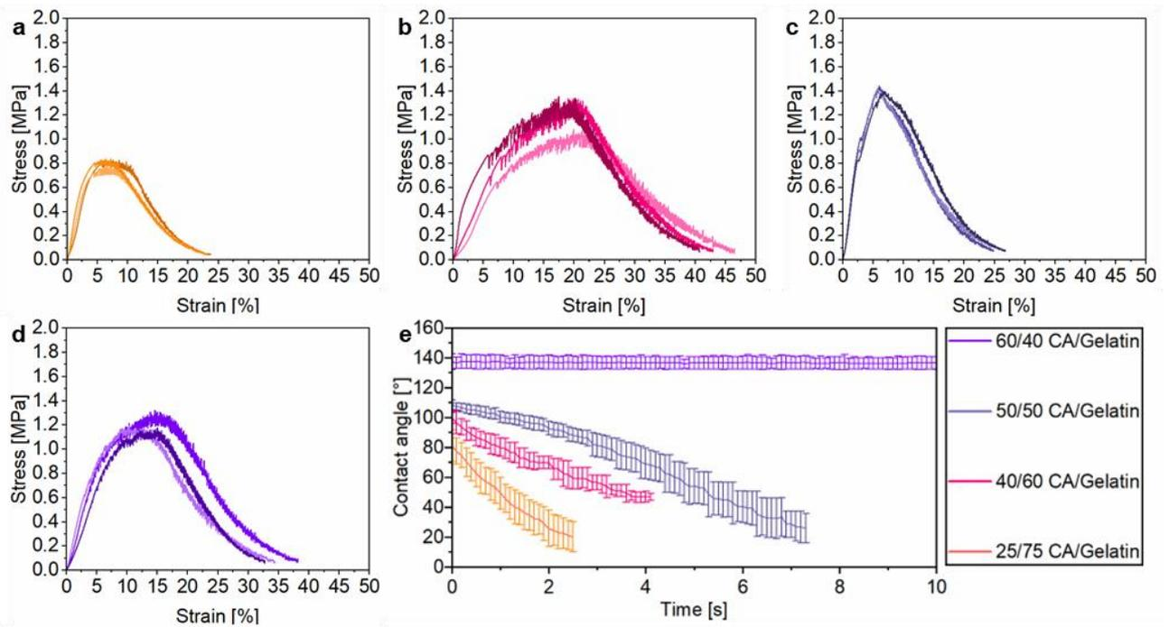
**Fig. S1** Systematic evaluation of electrospun fibers composed of cellulose acetate (CA) and gelatin in different ratios regarding their physicochemical properties. Stress-strain-curves of electrospun fiber mats of CA and gelatin in ratios of (a) 25/75, (b) 40/60, (c) 50/50 and (d) 60/40 as well as (e) contact angle measurements of all scaffolds.
