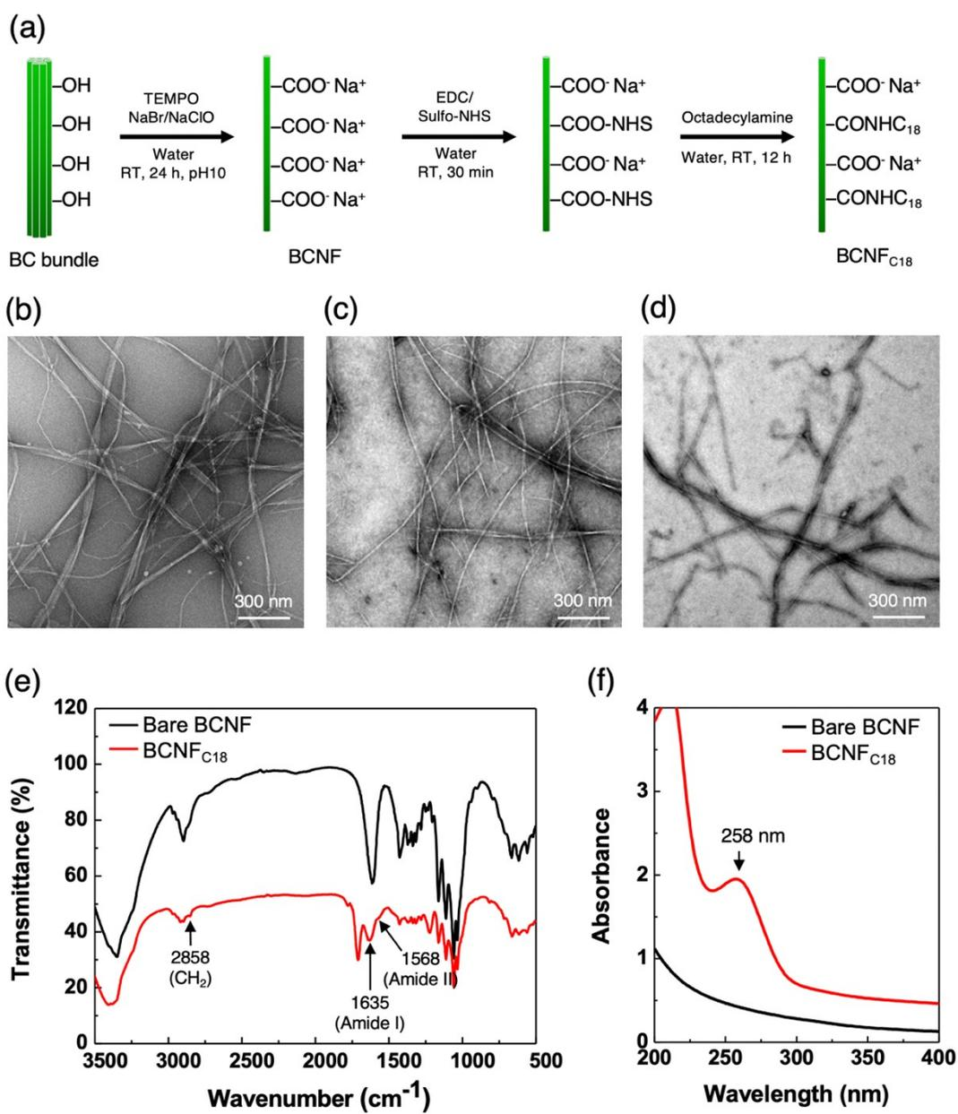
**Fig. S2** (a) Synthesis of  $\text{BCNF}_{\text{C18}}$  from a bacterial cellulose bundle. TEM images of bacterial celluloses (b) before and (c) after TEMPO oxidation, and (d) after grafting of C18 alkyl chains. (e) FT-IR spectra and (f) UV spectra of BCNFs before and after grafting of C18 alkyl chains.
