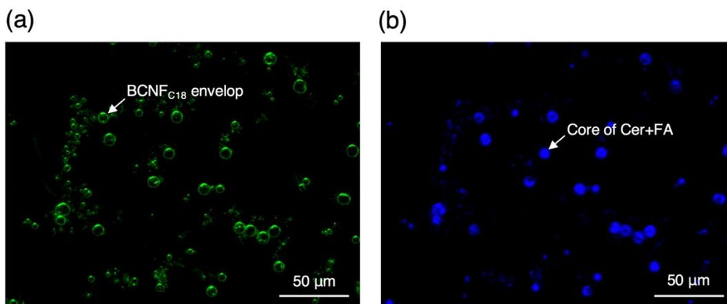
**Fig. S3** Fluorescence images of CerMPs labelled with (a) rhodamine B for BCNF<sub>C18</sub> membrane (green) and (b) 9-vinylanthracene for particle core (blue).  $\phi_{\text{Cer}} = 0.4$ , [Ceramide NP+SA] = 20 wt%, and [BCNF<sub>C18</sub>] = 0.5 wt%.
