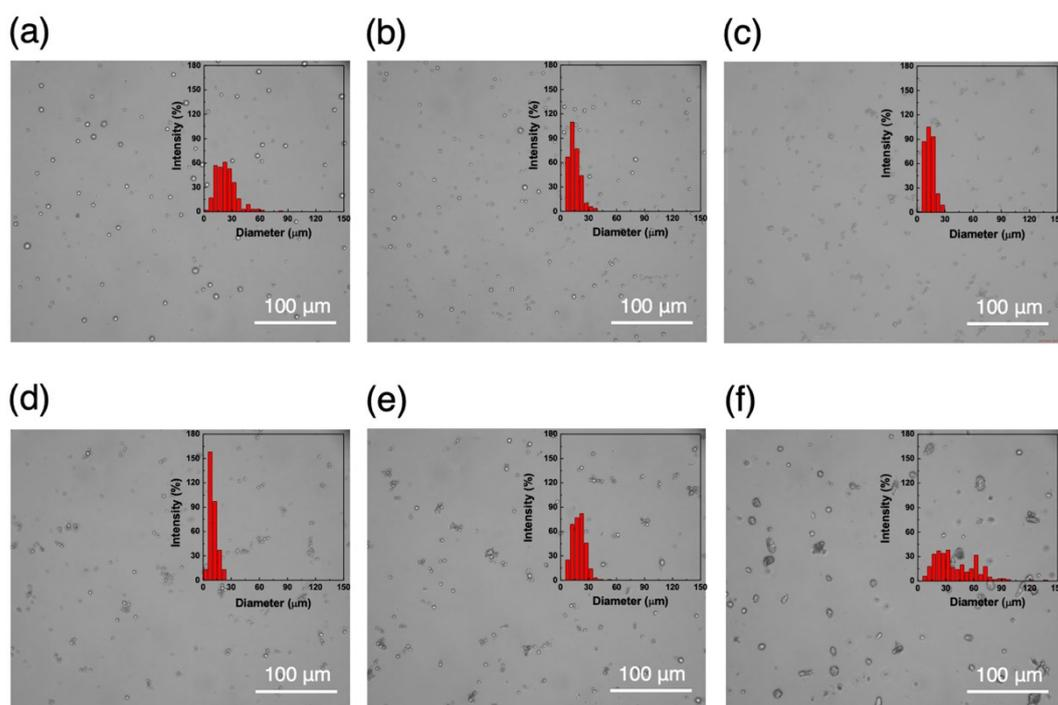
**Fig. S4** Bright-field microscope images and particle size distribution of CerMPs with varying the incorporation amount of C18 alkyl chain against total mass of Ceramide NP and FA: (a) 0.08 mmol g<sup>-1</sup>, (b) 0.16 mmol g<sup>-1</sup>, (c) 0.48 mmol g<sup>-1</sup>, (d) 0.64 mmol g<sup>-1</sup>, (e) 0.96 mmol g<sup>-1</sup>, and (f) 1.28 mmol g<sup>-1</sup> octadecylamine.  $\phi_{\text{Cer}} = 0.4$ , [Ceramide NP+SA] = 20 wt%, and [BCNF<sub>C18</sub>] = 0.5 wt%.
