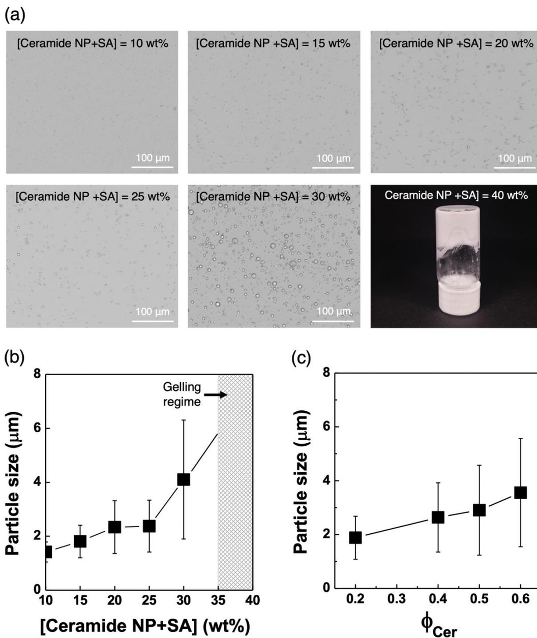
**Fig. S6** (a) Bright-field microscope images of CerMPs with varying the solid (Ceramide NP + SA) concentration. A gel-like dispersion phase was obtained from around 35 wt%. Average particle size change of CerMPs with varying (b) the core content at  $\phi_{Cer} = 0.4$  and (c) the  $\phi_{Cer}$  at [Ceramide NP+SA] = 20 wt%. [BCNF<sub>C18</sub>] = 0.5 wt%.
