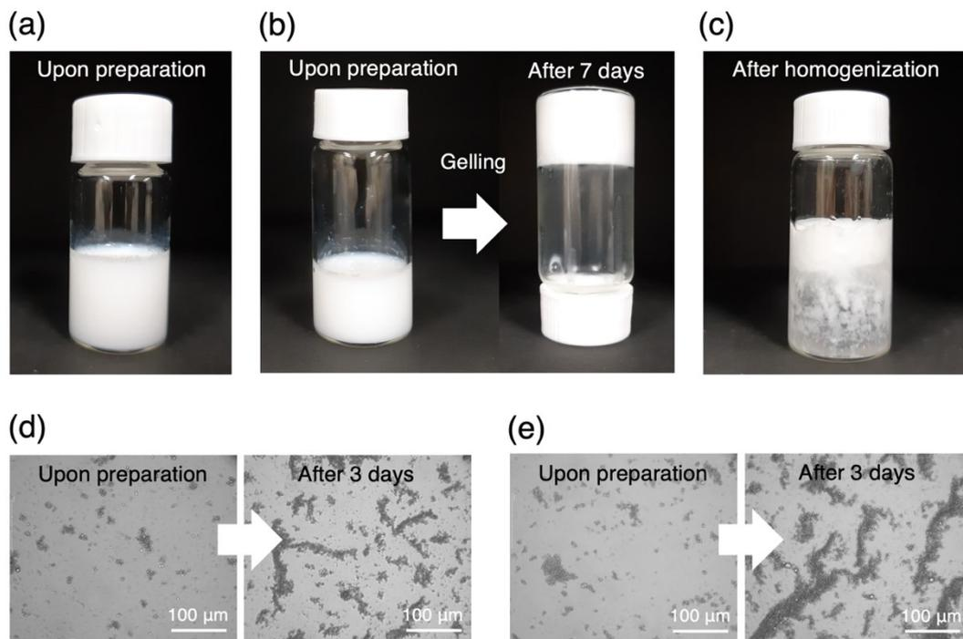
**Fig. S5** Appearances CerMP dispersions prepared with conventional molecular surfactants: (a) Pluronic F127, (b) Tween 80, and (c) SLS.  $\phi_{\text{Cer}} = 0.2$ , [Ceramide NP+SA]=20 wt%, and [Surfactant] = 5 wt%. Destabilization behavior of CerMPs prepared with Pluronic F127 with the storage time at 4 °C: (d) [Pluronic F127] = 3 wt% and (e) [Pluronic F127] = 5 wt%.  $\phi_{\text{Cer}} = 0.2$  and [Ceramide NP+SA] = 20 wt%.
