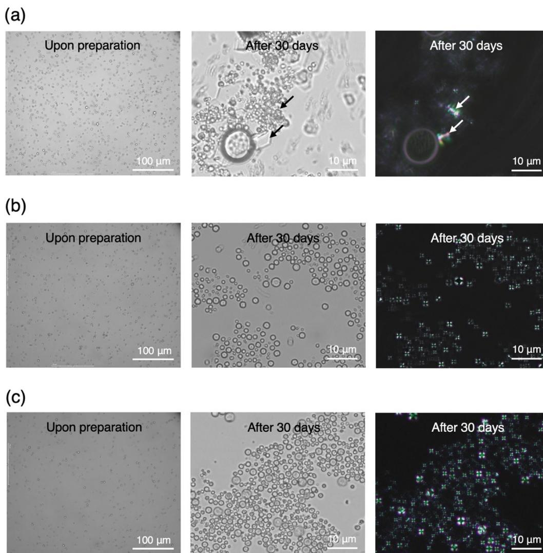
**Fig. S8** Bright-field microscope images and polarized microscope images of CerMPs upon preparation and after 30-day storage at 4 °C: (a) CerMP<sub>MA</sub>, (b) CerMP<sub>SA</sub>, and (c) CerMP<sub>BA</sub>. Arrows indicate ceramide crystals grown out of CerMP<sub>MA</sub> in the aqueous phase.  $\phi_{\text{Cer}} = 0.4$ , [Ceramide NP+FA] = 20 wt%, and [BCNF<sub>C18</sub>] = 0.5 wt%.
