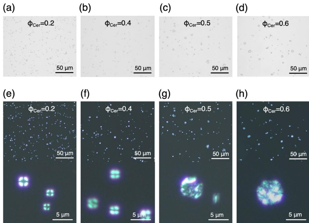
**Fig. S7** Bright-field microscope (a-d) and polarized microscope images (e-h) of CerMPs prepared with varying  $\phi_{\text{Cer}}$  after 6-month storage at 4 °C. [Ceramide NP+BA] = 20 wt% and [BCNF<sub>C18</sub>] = 0.5 wt%.
